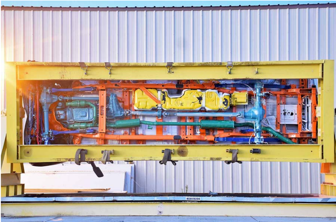
FIGURE 76. Vehicle at 270° on Static Rollover Device
