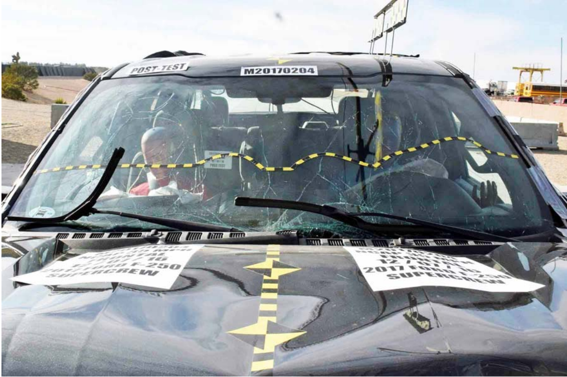
FIGURE 19. Post-Test Windshield View
