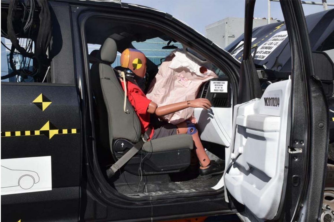
FIGURE 56. Post-Test Passenger Dummy and Vehicle Interior View
