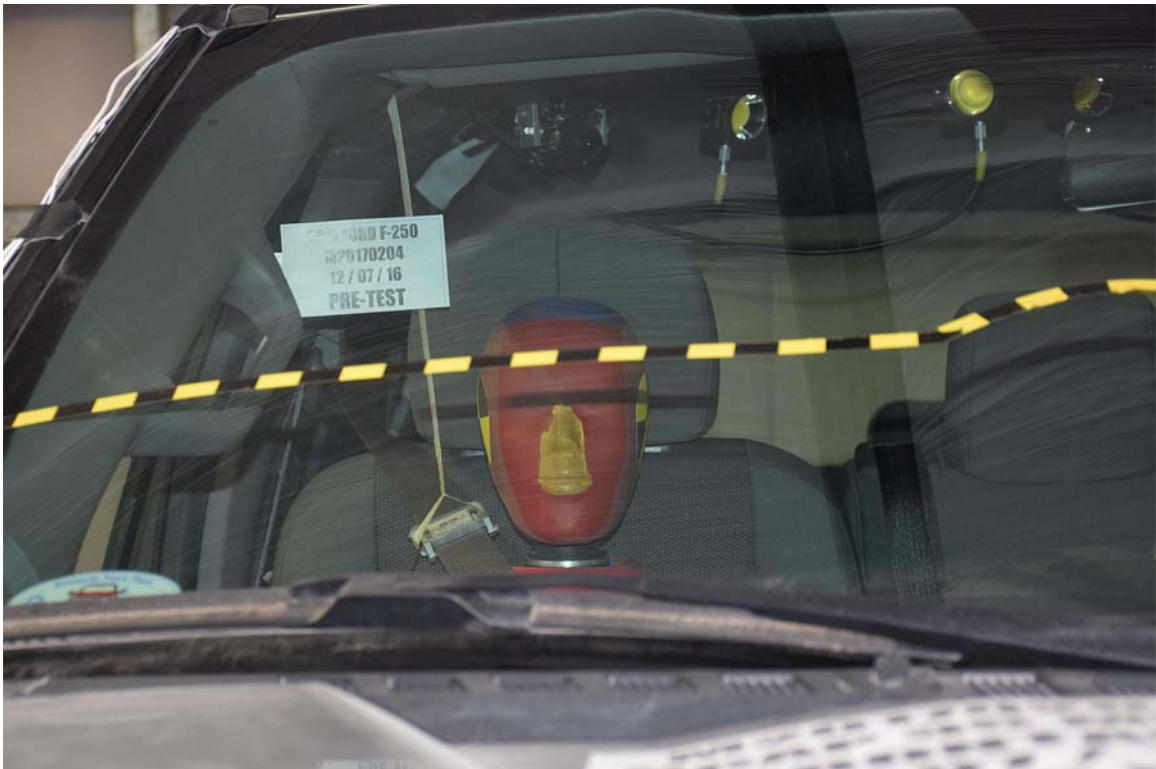
FIGURE 51. Pre-Test Passenger Dummy Front View
