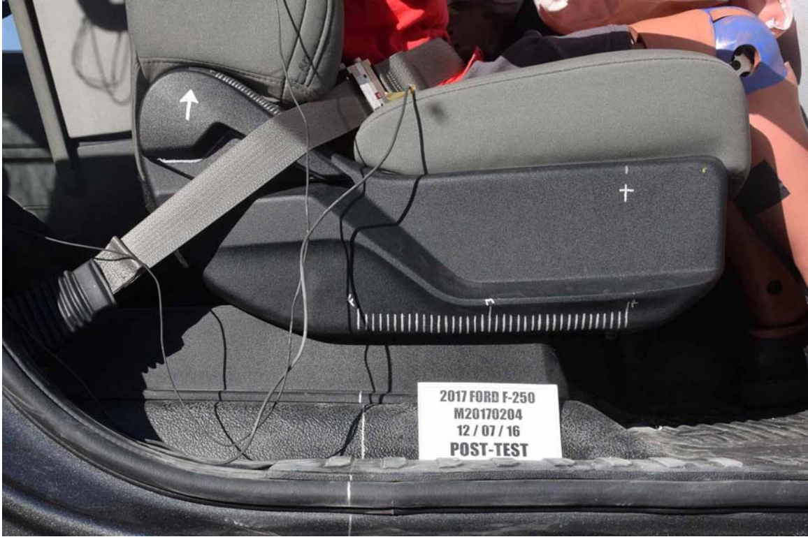
FIGURE 58. Post-Test Passenger's Seat Fore-Aft Markings
