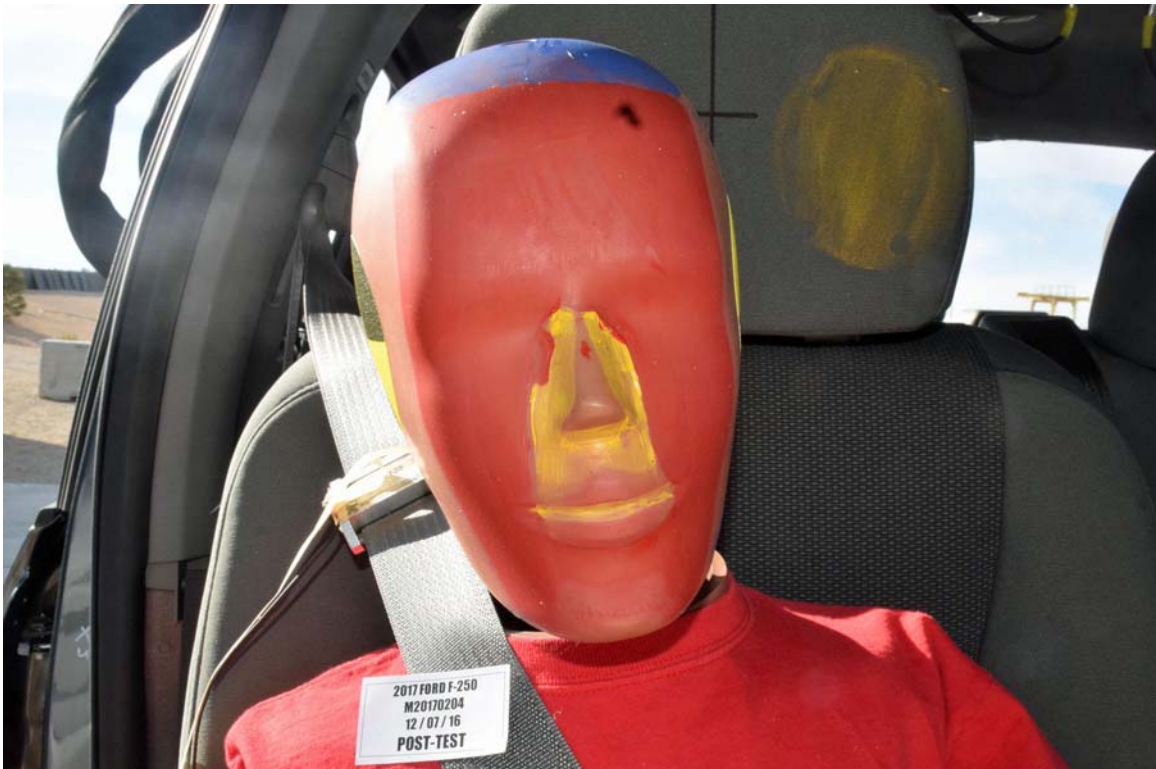
FIGURE 67. Post-Test Passenger Dummy Face
