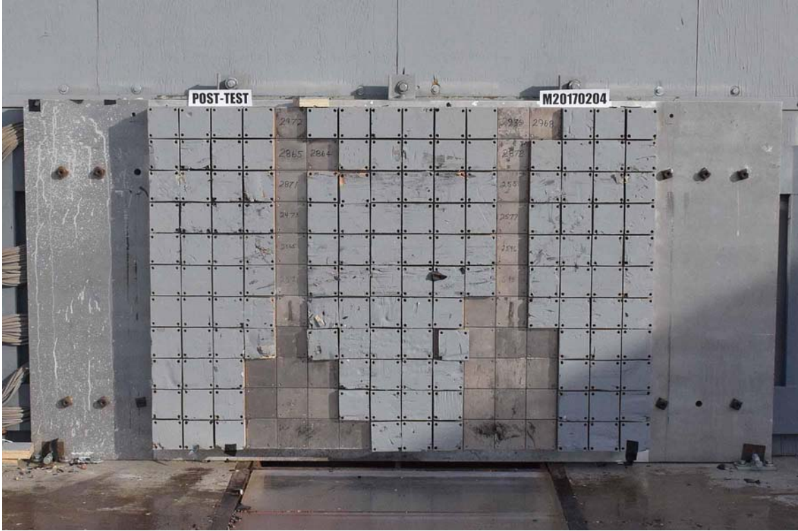
FIGURE 3. Post-Test Load Cell Wall
