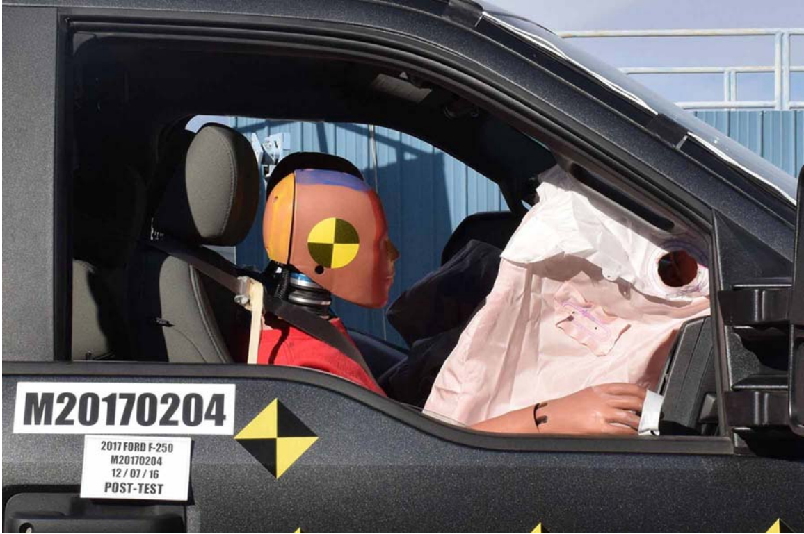
FIGURE 54. Post-Test Passenger Dummy Window View
