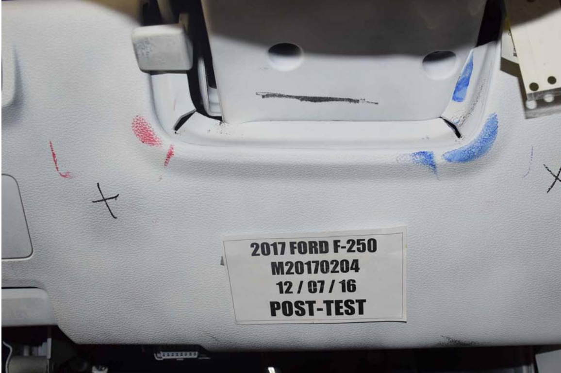
FIGURE 48a. Post-Test Driver Dummy Contact with Knee Bolster
