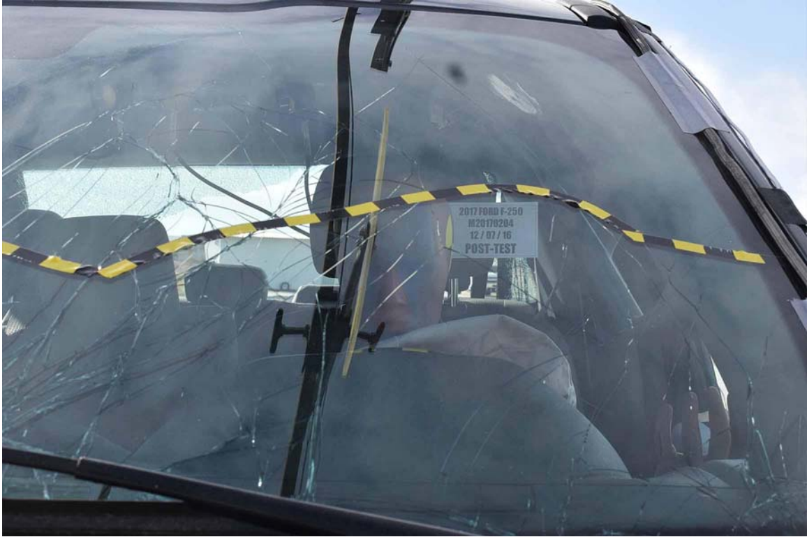
FIGURE 31. Post-Test Driver Dummy Front View
