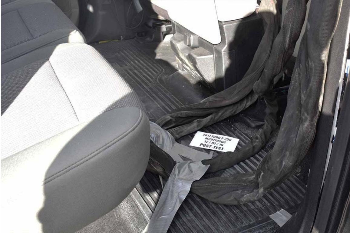
FIGURE 29. Post-Test Dummy Cable Routing
