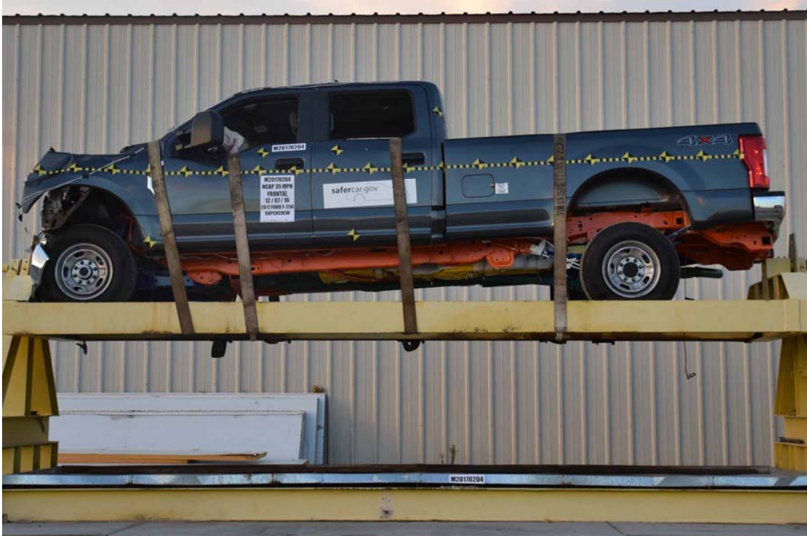
FIGURE 73. Vehicle at 0° on Static Rollover Device
