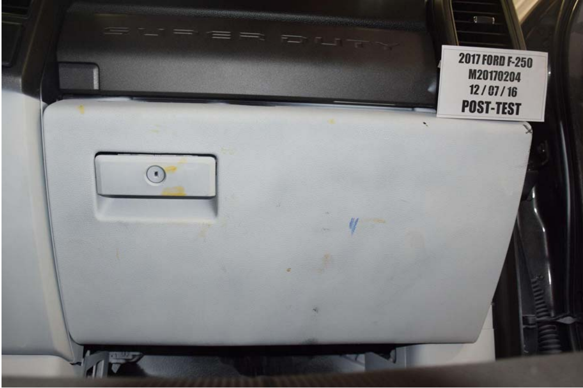
FIGURE 64. Post-Test Passenger's Side Knee Bolster
