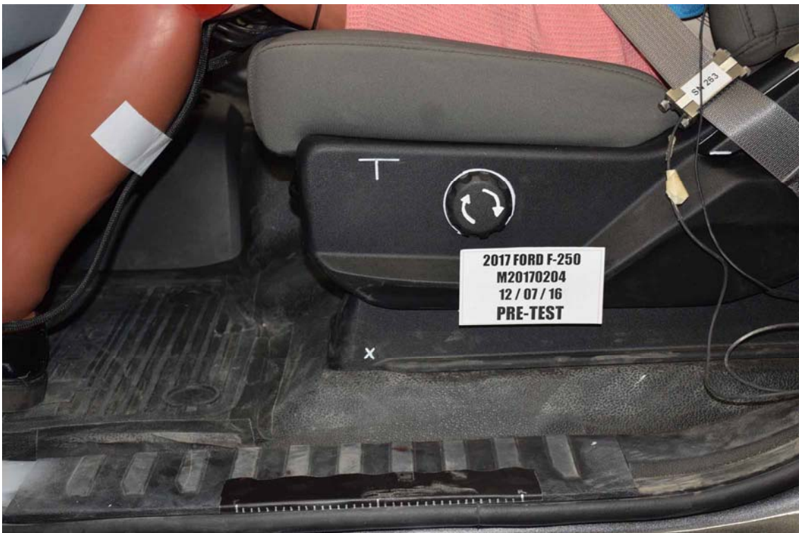
FIGURE 36. Pre-Test Driver's Seat Fore-Aft Markings
