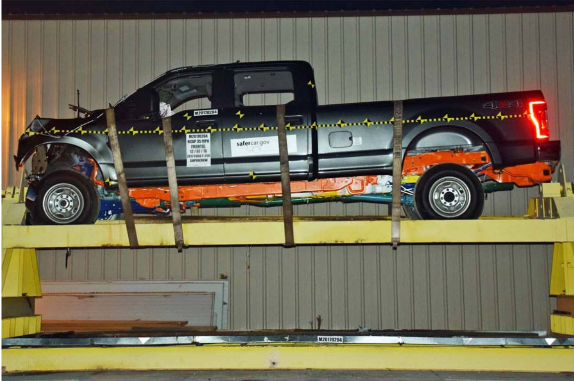
FIGURE 77. Vehicle at 360° on Static Rollover Device
