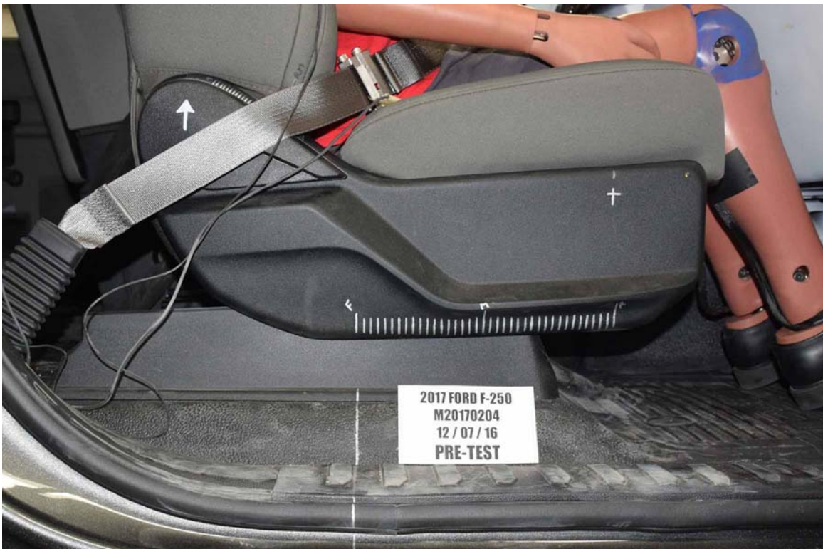
FIGURE 57. Pre-Test Passenger's Seat Fore-Aft Markings
