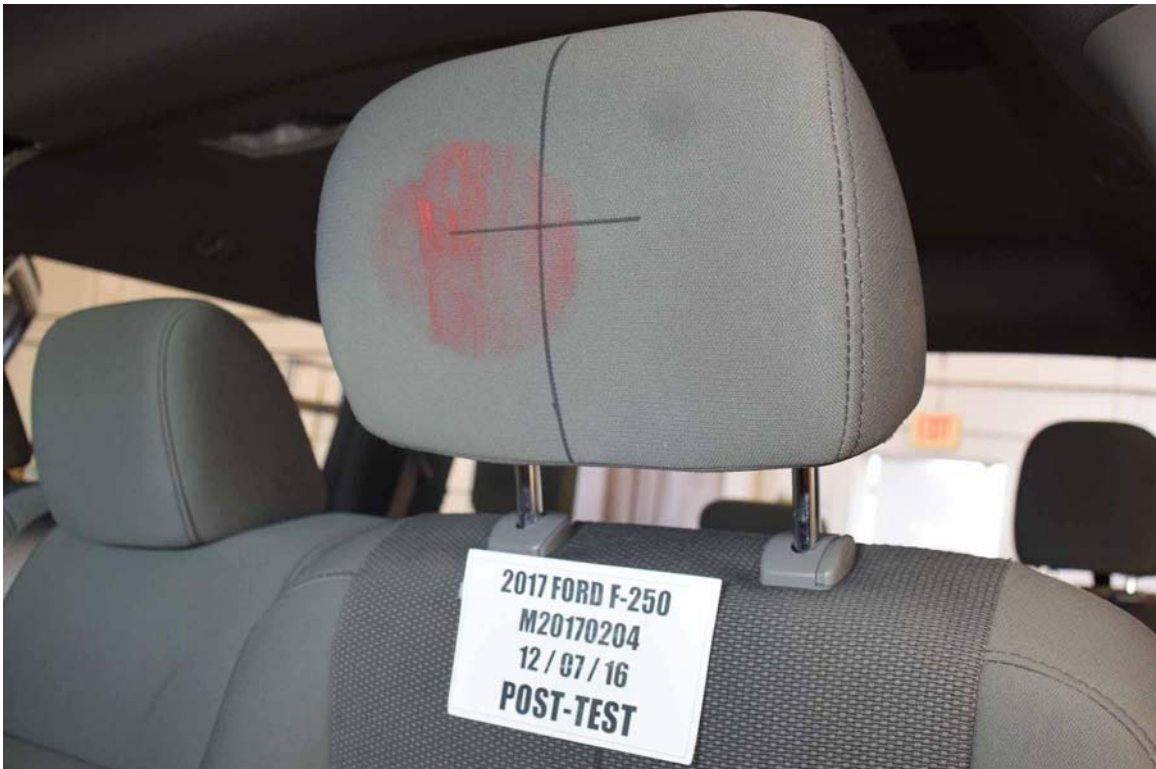
FIGURE 48. Post-Test Driver Dummy Contact with Headrest
