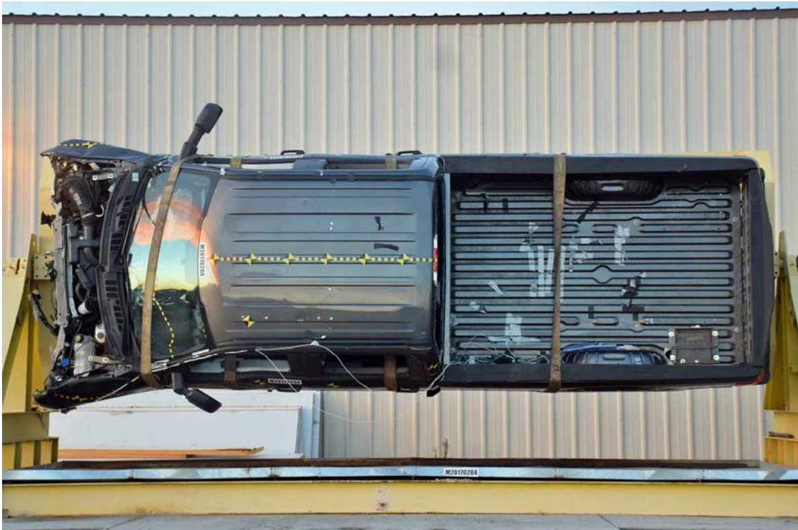
FIGURE 74. Vehicle at 90° on Static Rollover Device
