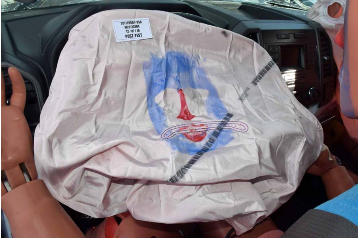
FIGURE 47. Post-Test Driver Dummy Contact with Airbag
