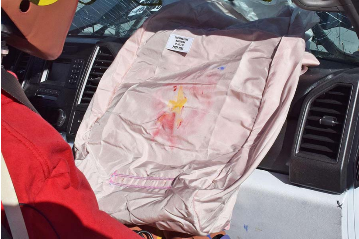
FIGURE 68. Post-Test Passenger Dummy Contact with Airbag
