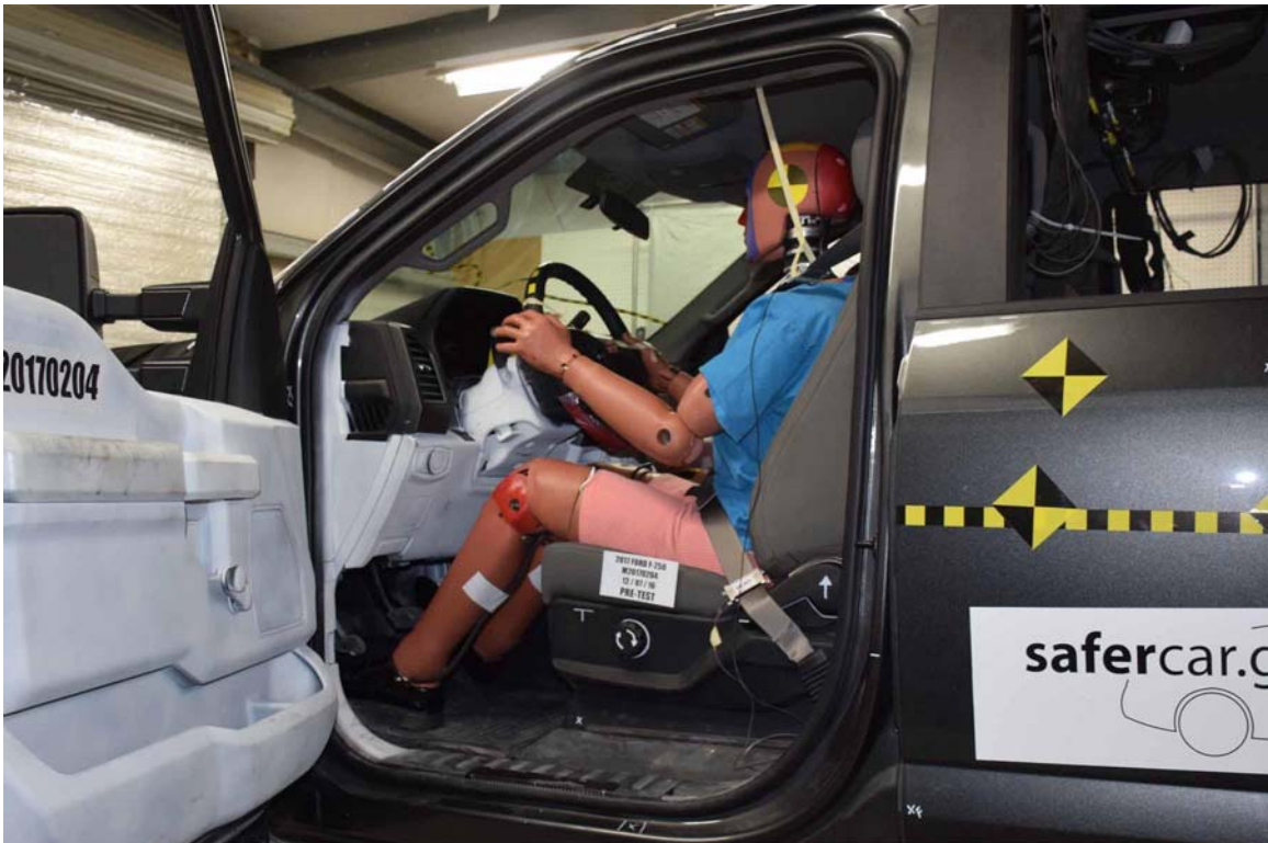
FIGURE 34. Pre-Test Driver Dummy and Vehicle Interior View
