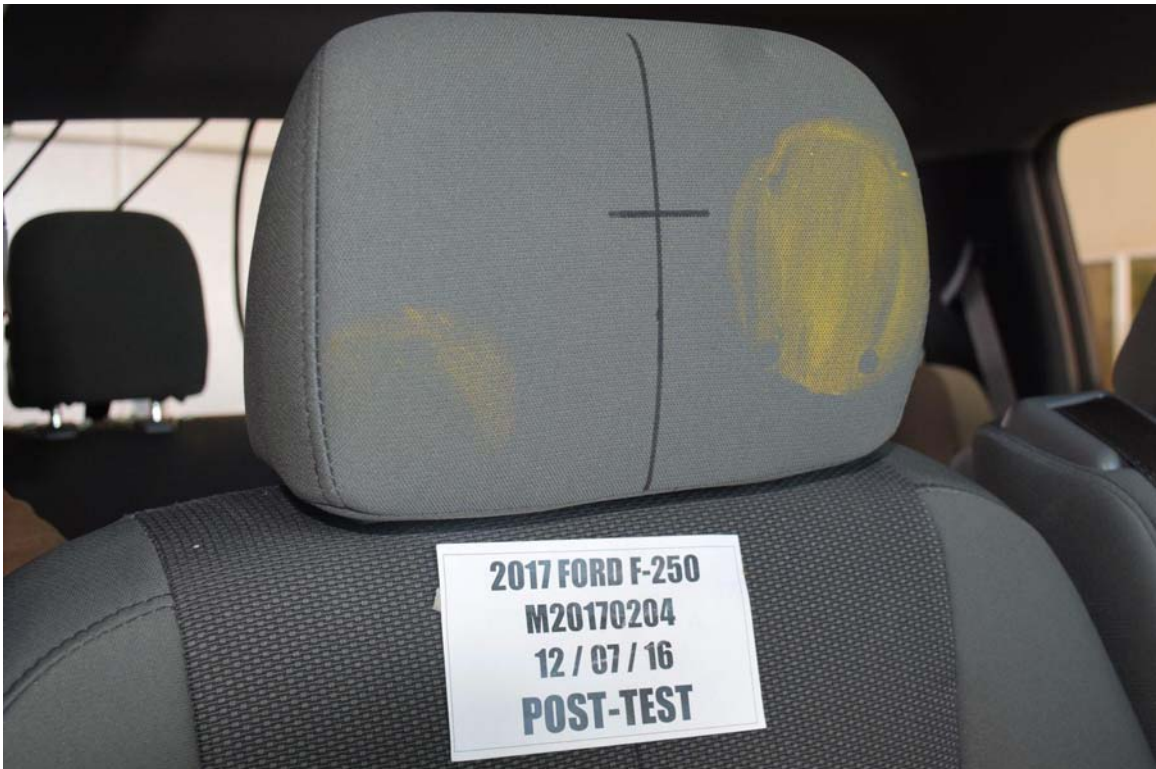
FIGURE 69. Post-Test Passenger Dummy Contact with Headrest
