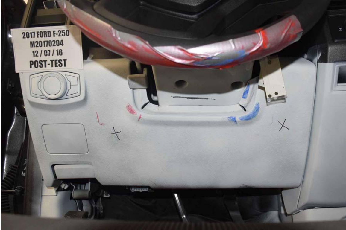
FIGURE 43. Post-Test Driver's Side Knee Bolster
