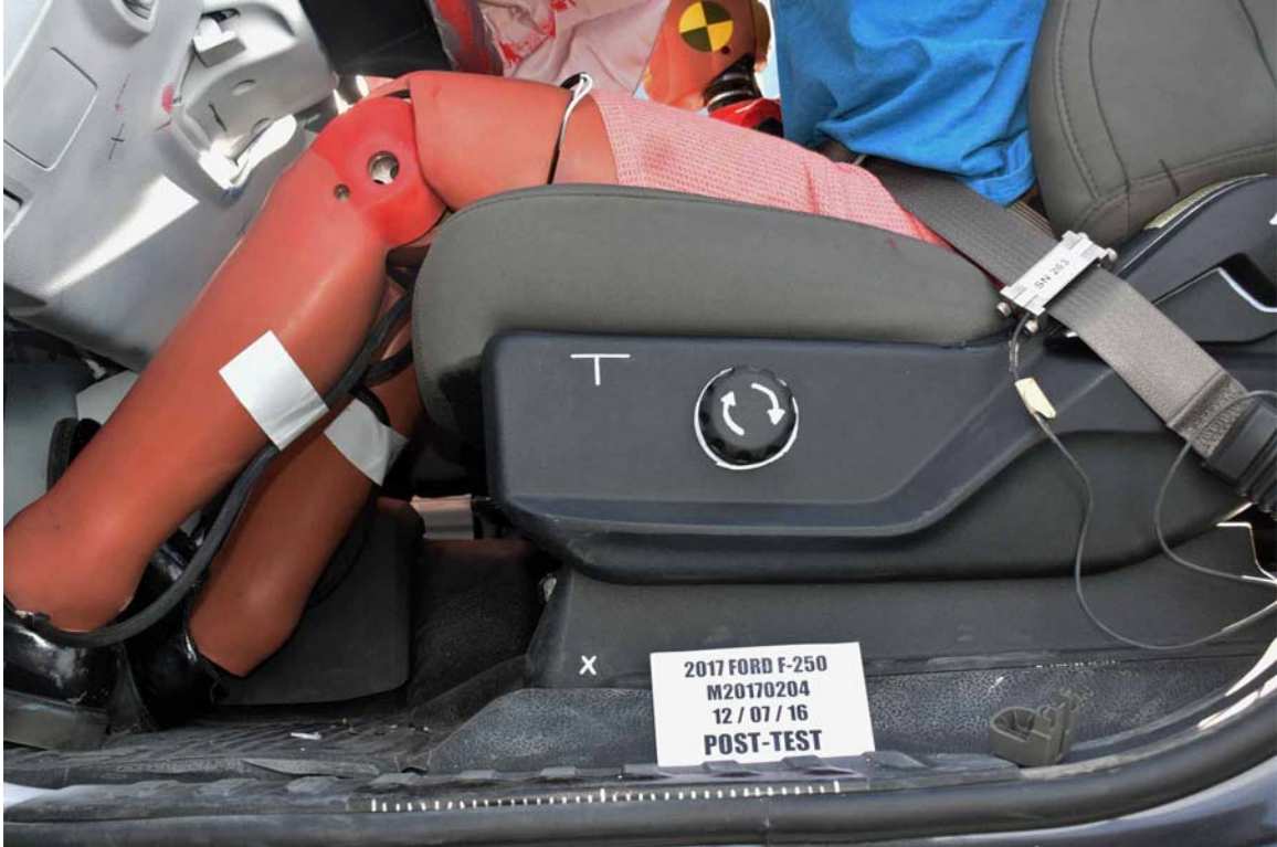
FIGURE 37. Post-Test Driver's Seat Fore-Aft Markings
