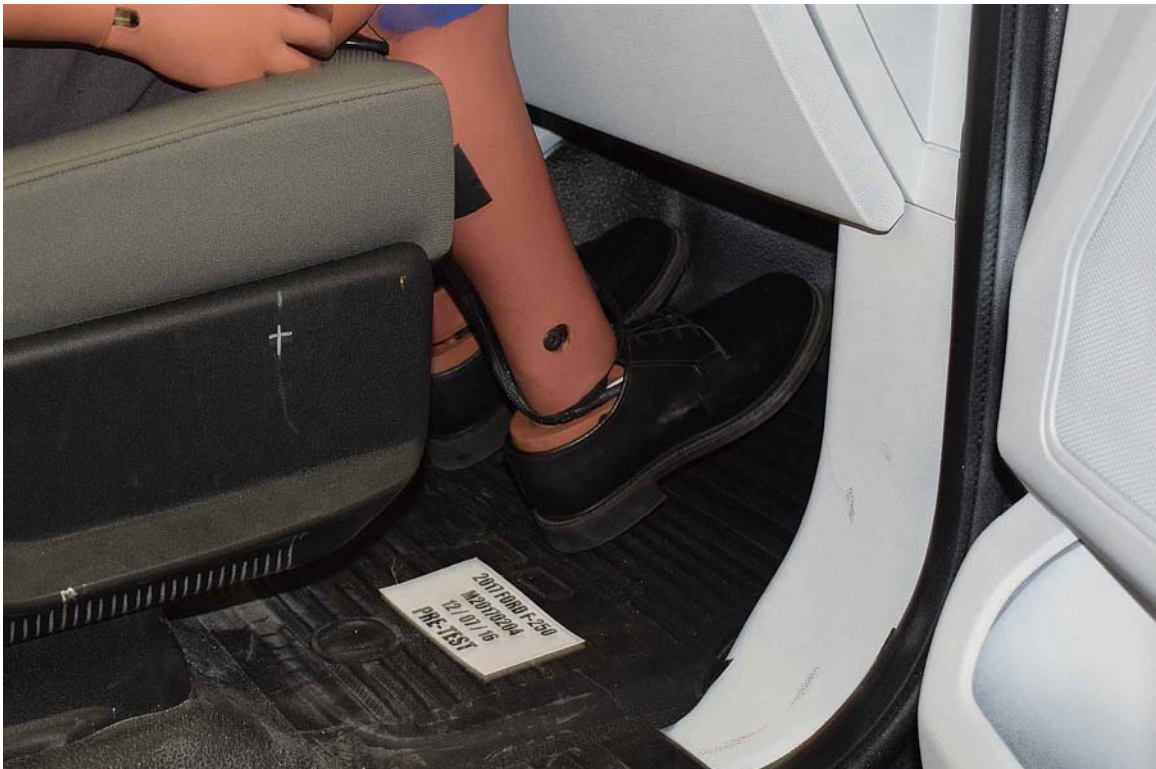
FIGURE 61. Pre-Test Passenger Dummy Feet
