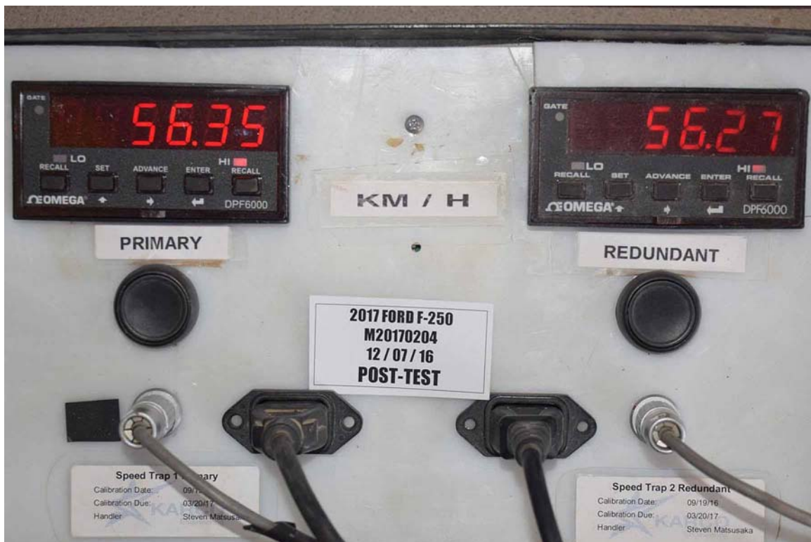
FIGURE 72. Post-Test Speed Trap Read-Out
