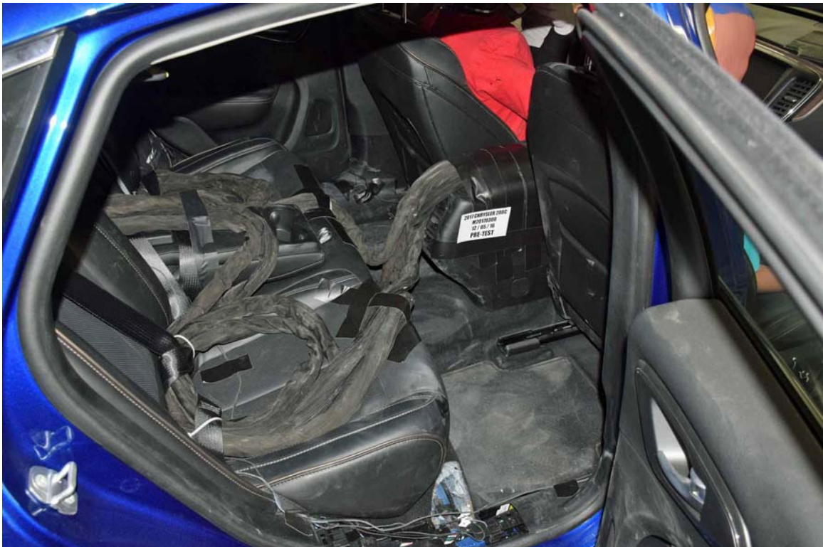
FIGURE 28. Pre-Test Dummy Cable Routing
