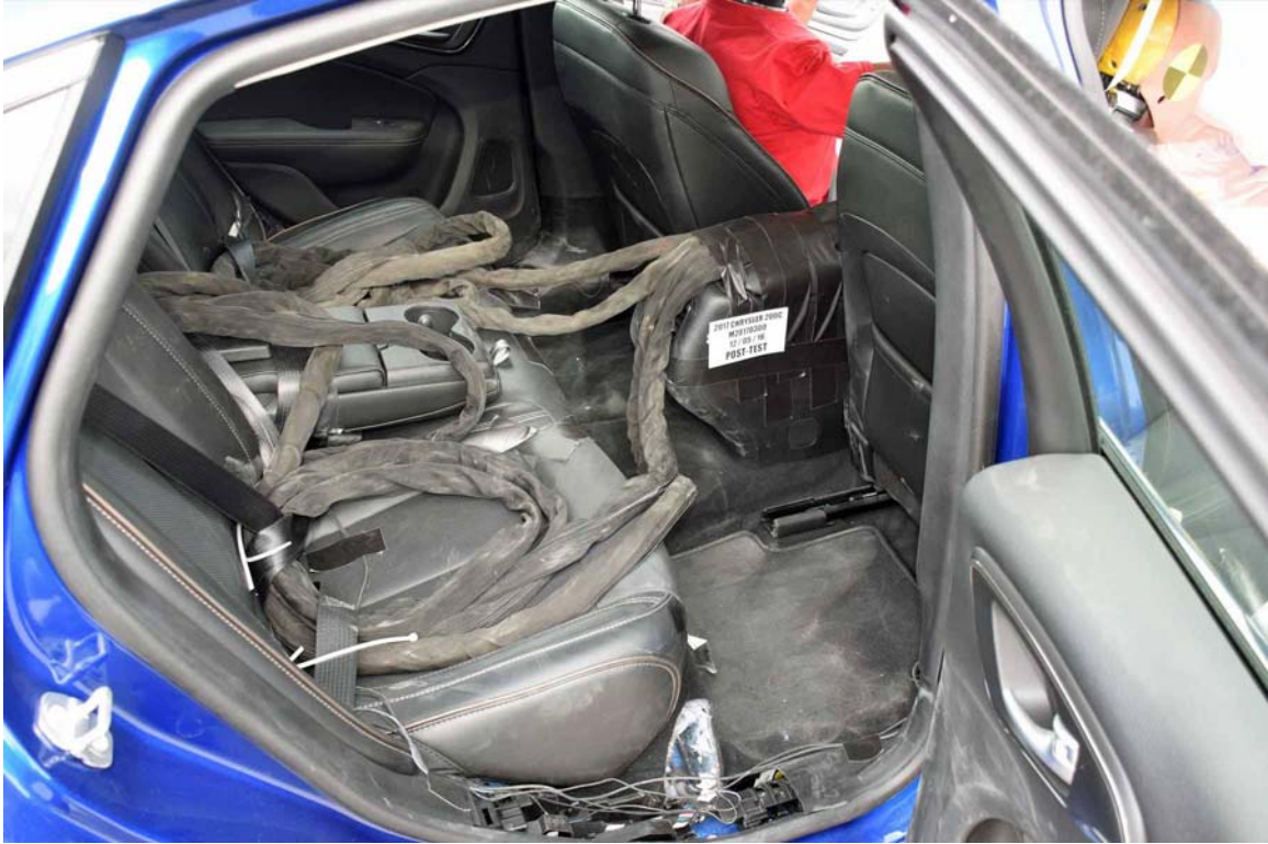
FIGURE 29. Post-Test Dummy Cable Routing
