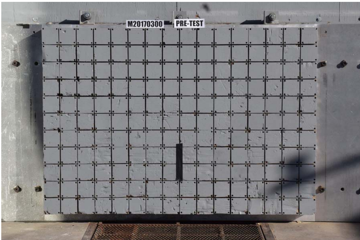
FIGURE 2. Pre-Test Load Cell Wall
