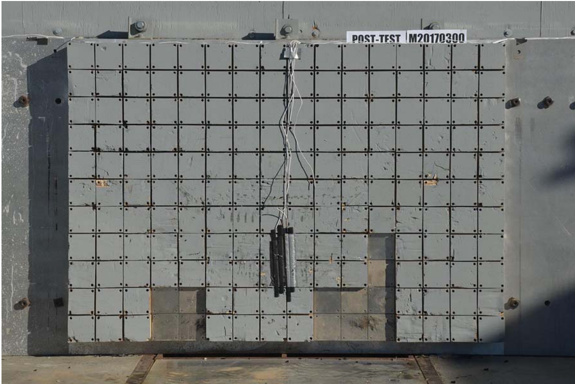
FIGURE 3. Post-Test Load Cell Wall
