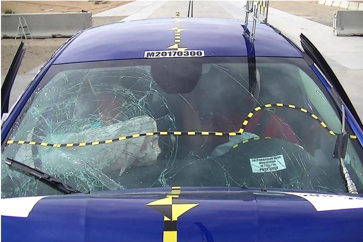
FIGURE 19. Post-Test Windshield View
