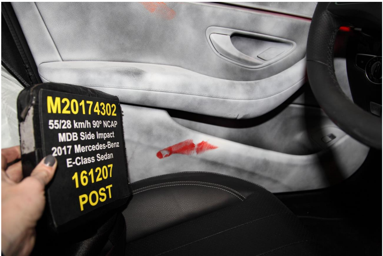
052 Post-Test Driver Dummy Close-Up Pelvis Contact View
