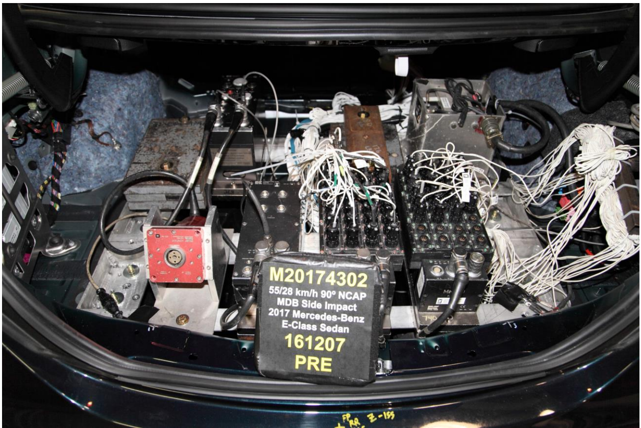
094 Pre-Test Ballast View
