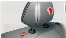
Fig. 68 Rear seat: removing the head restraint
