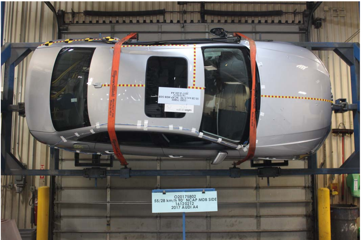
Photo No. 097 - FMVSS No. 301 Static Rollover 90 Degrees
