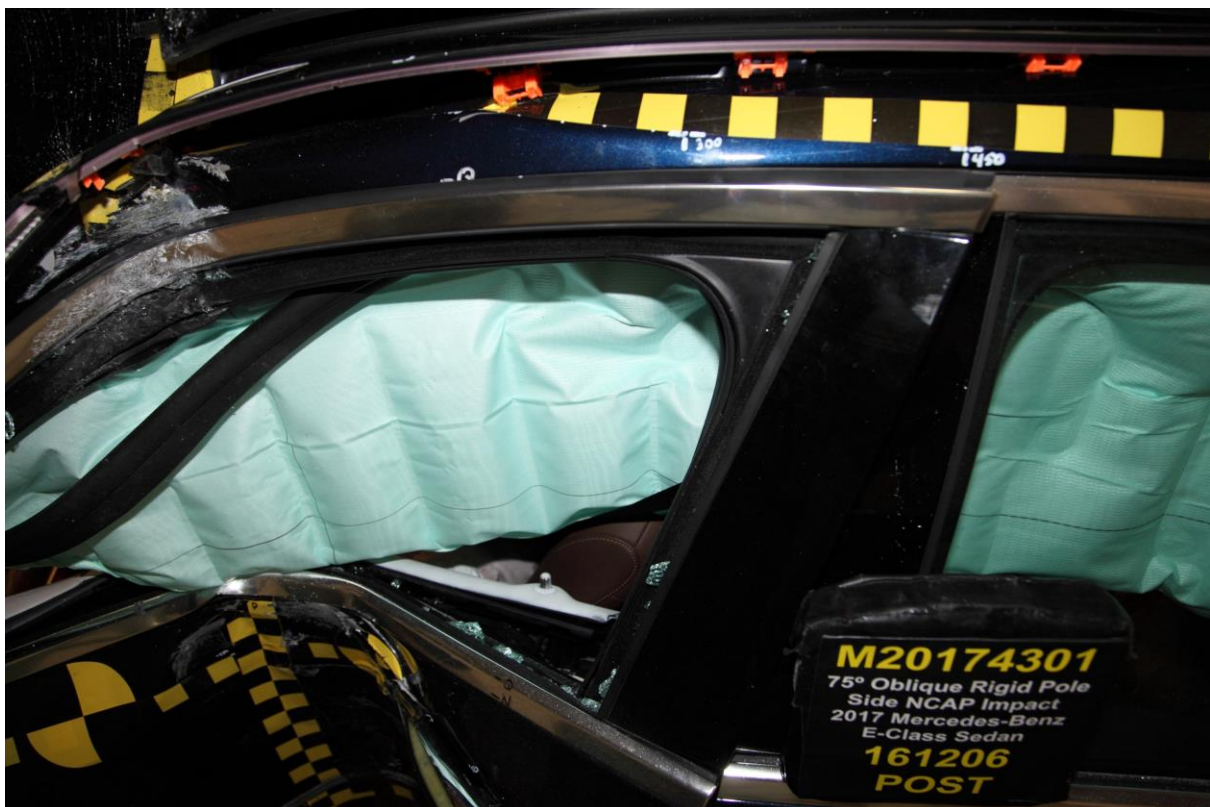
No. 041 Post-Test Dummy and Door Clearance View
