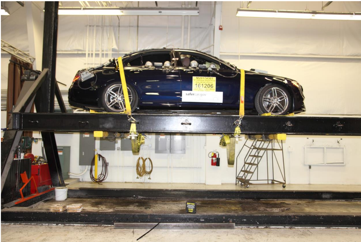
No. 067 FMVSS No. 301 Static Rollover 360 Degrees
