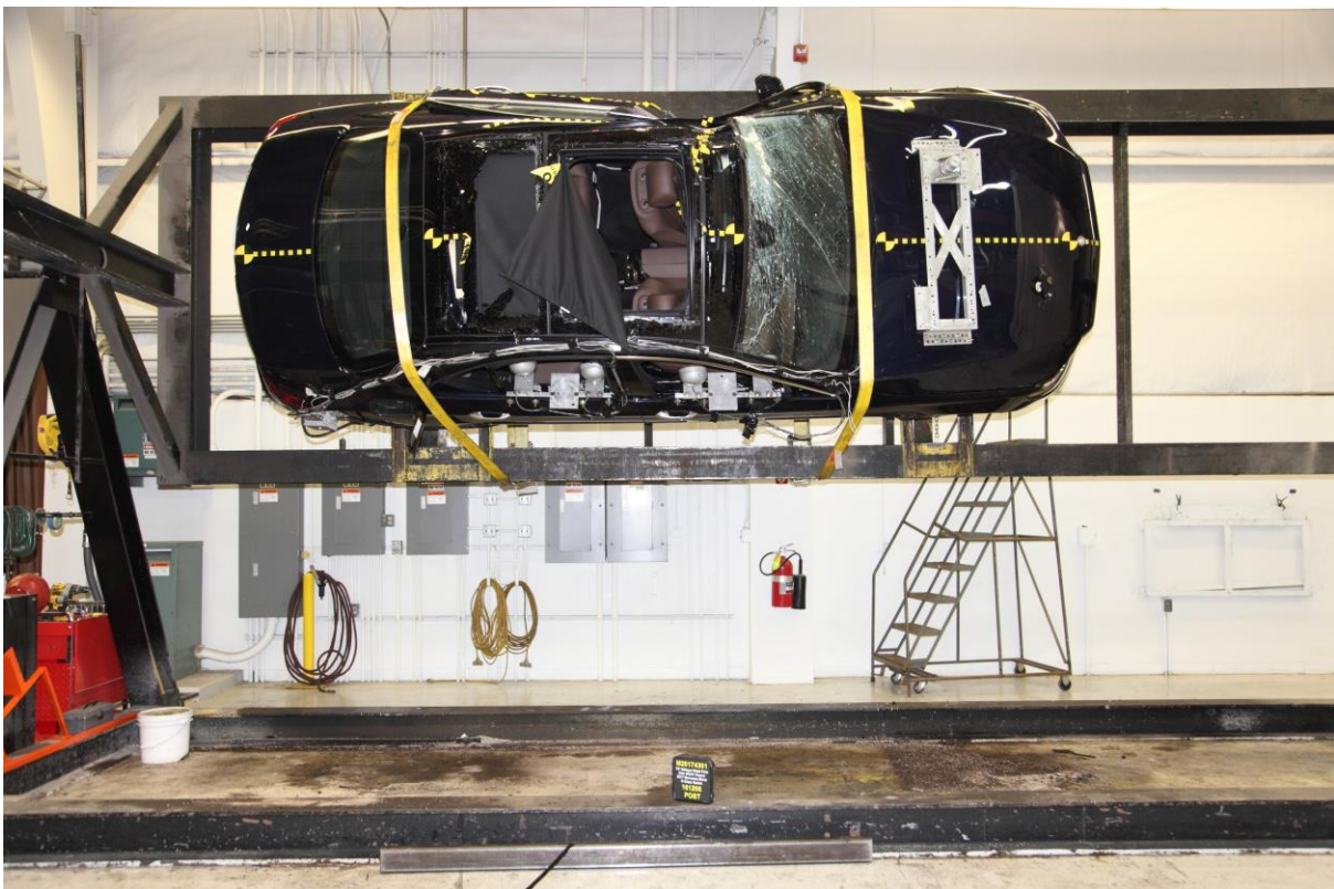
No. 064 FMVSS No. 301 Static Rollover 90 Degrees
