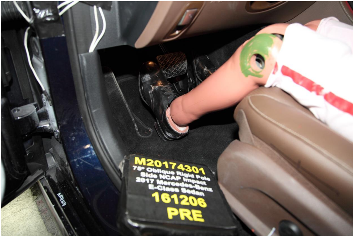
No. 032 Pre-Test Placement of Dummy Feet
