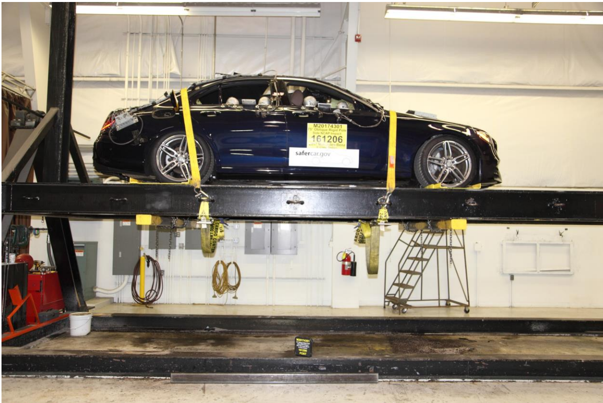
No. 063 FMVSS No. 301 Static Rollover 0 Degrees
