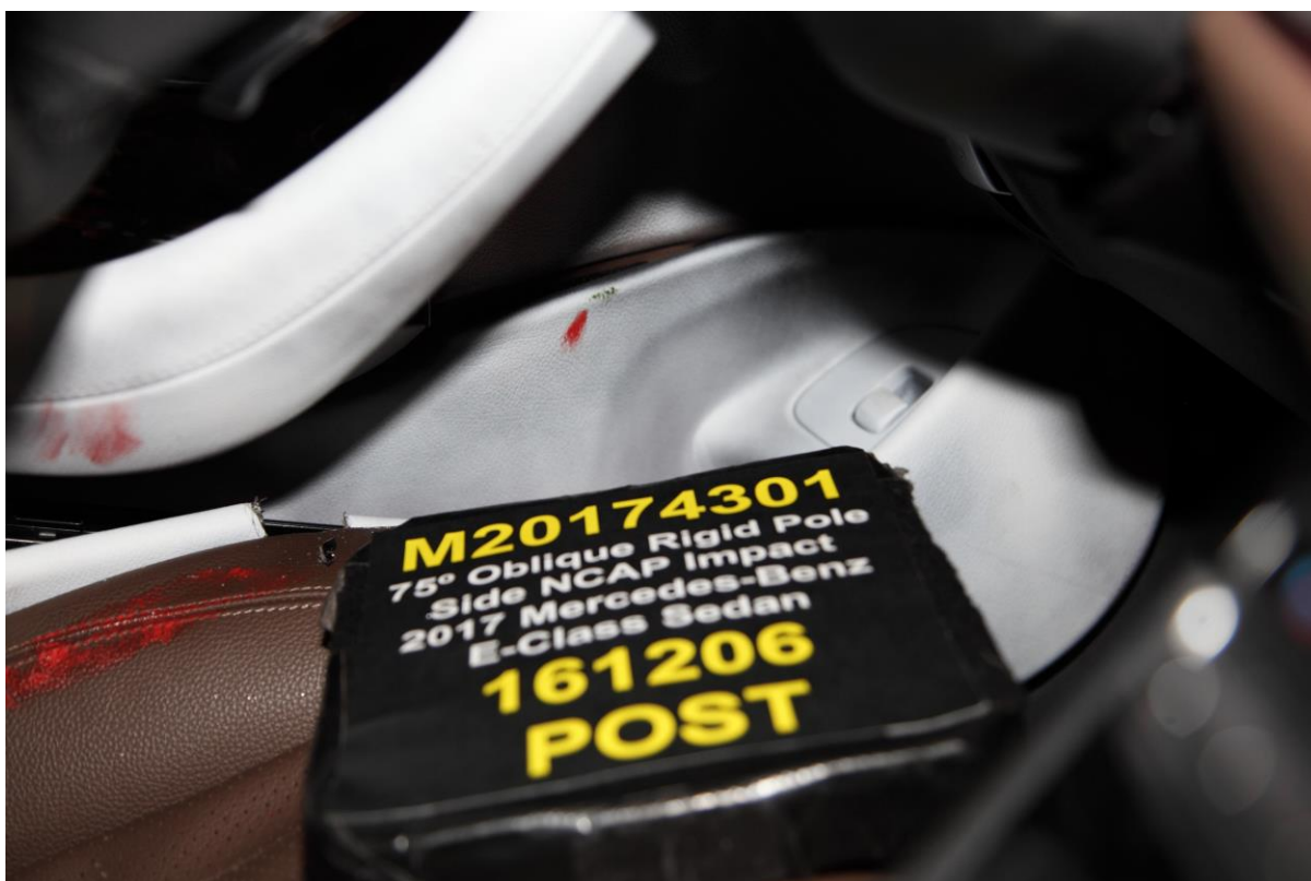
No. 052 Post-Test Dummy Close-Up Knee Contact with Vehicle Interior View
