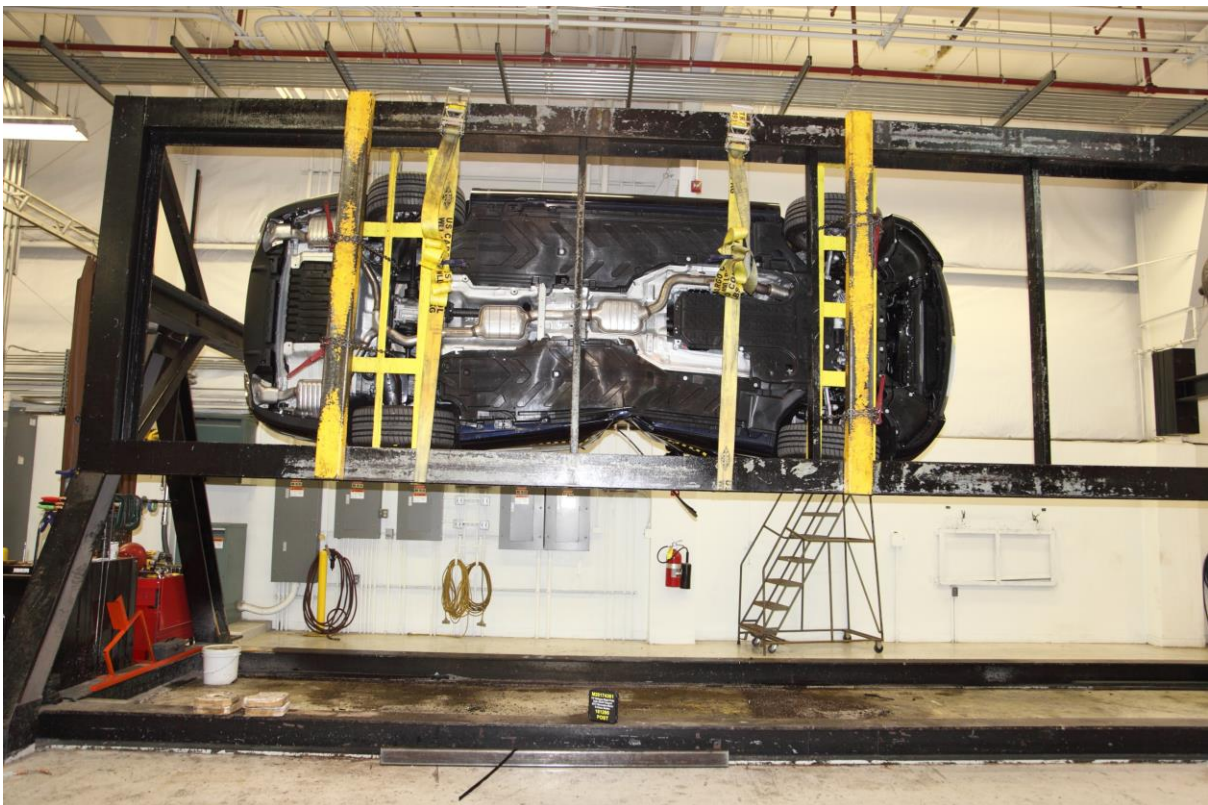
No. 066 FMVSS No. 301 Static Rollover 270 Degrees
