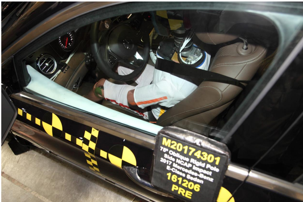
No. 040 Pre-Test Dummy and Door Clearance View
