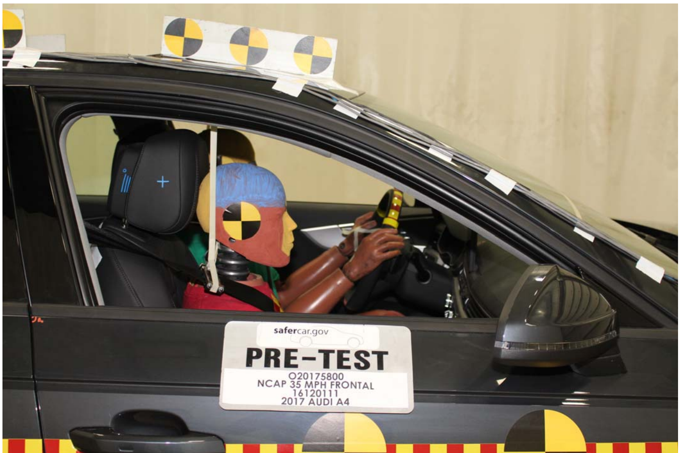
Photo No. 053 - Pre-Test Passenger Dummy Window View
