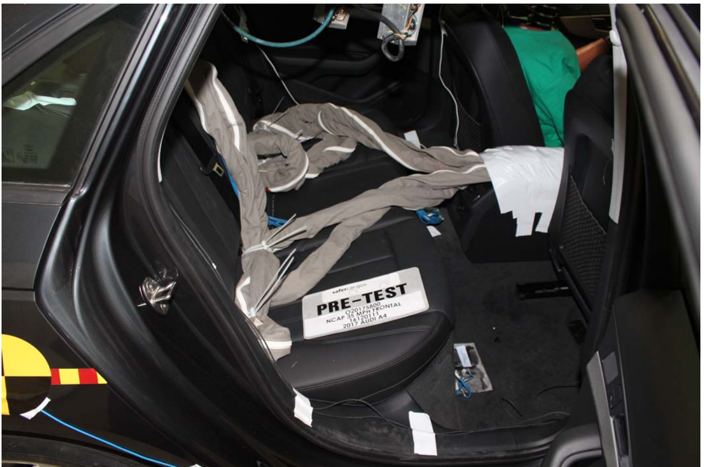
Photo No. 028 - Pre-Test Dummy Cable Routing
