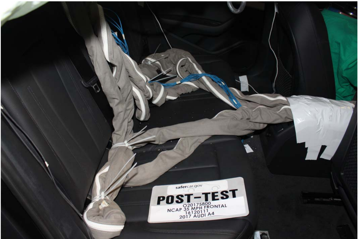
Photo No. 029 - Post-Test Dummy Cable Routing
