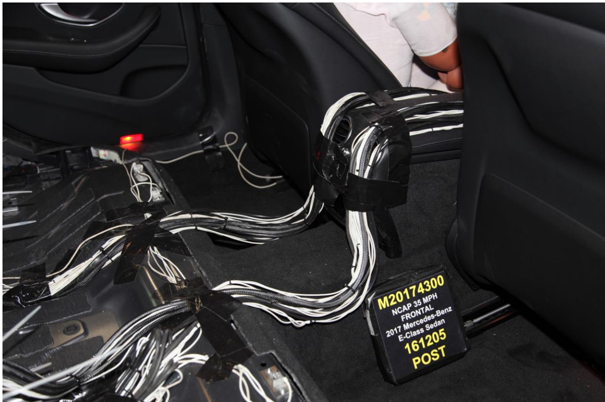
029 Post-Test Dummy Cable Routing
