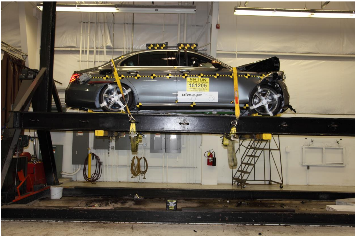
077 Vehicle at 360° on Static Rollover Device
