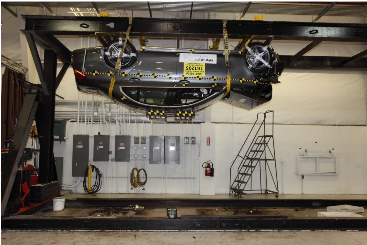
075 Vehicle at 180° on Static Rollover Device
