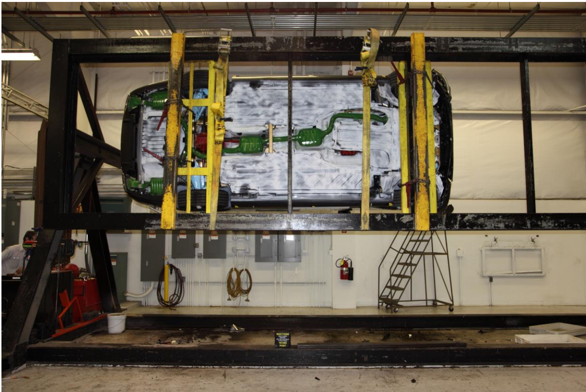
076 Vehicle at 270° on Static Rollover Device
