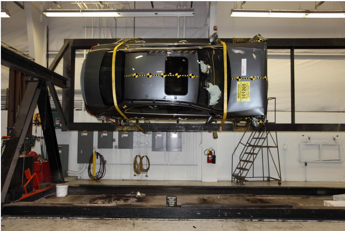
074 Vehicle at 90° on Static Rollover Device
