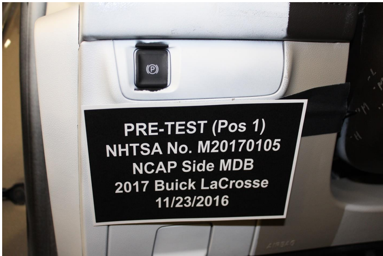
Figure A-37: View of Disengaged Parking Brake
