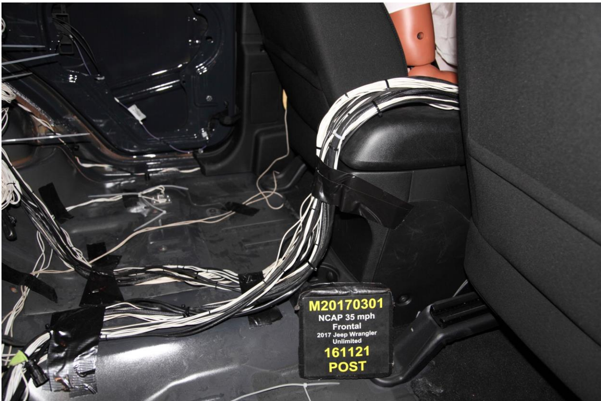
029 Post-Test Dummy Cable Routing
