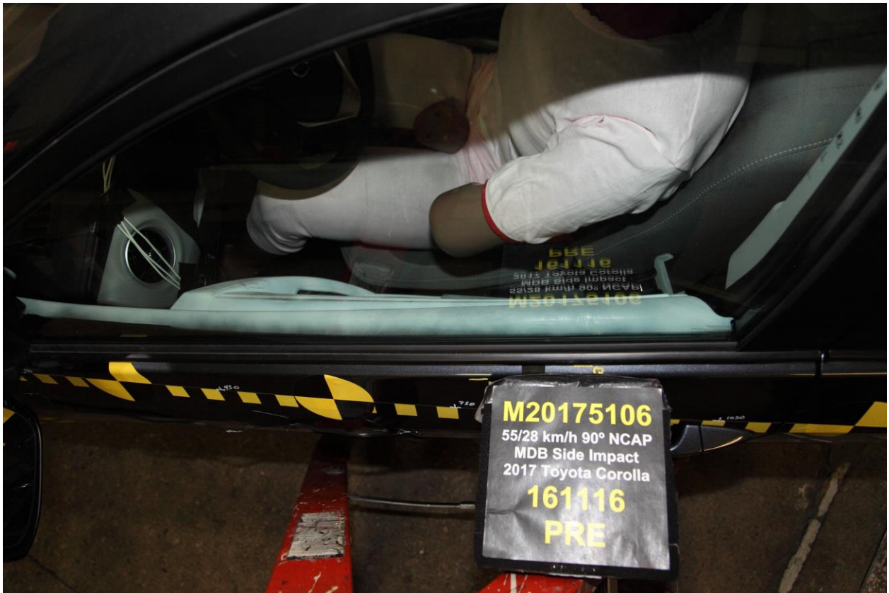
042 Pre-Test Driver Dummy and Door Clearance View
