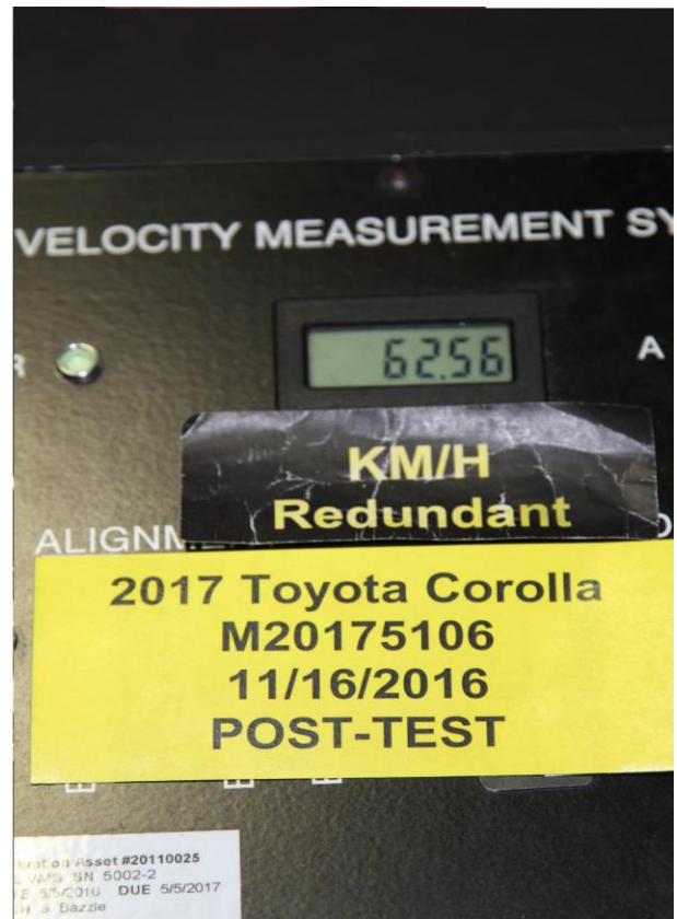
095 Post-Test Primary Speed Trap Read-Out
