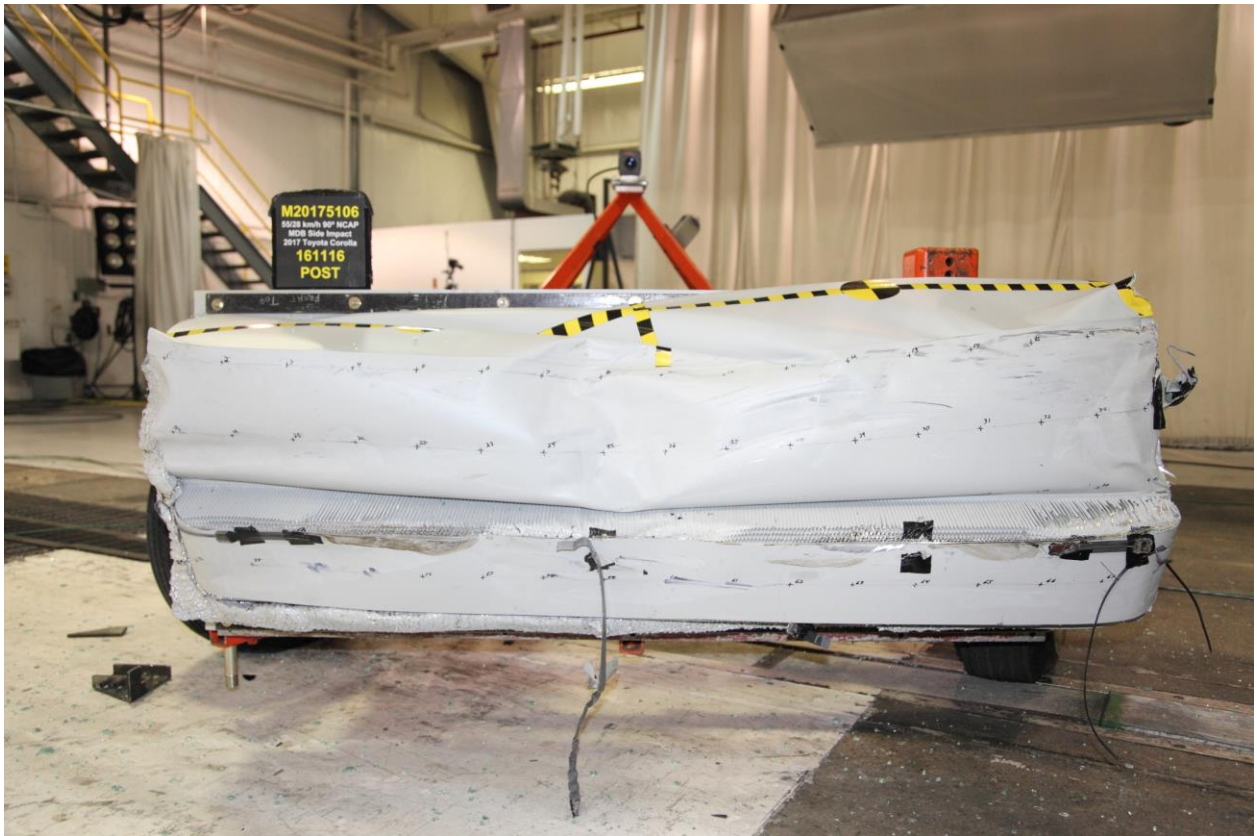
085 Post-Test Front View of MDB Impactor Face
