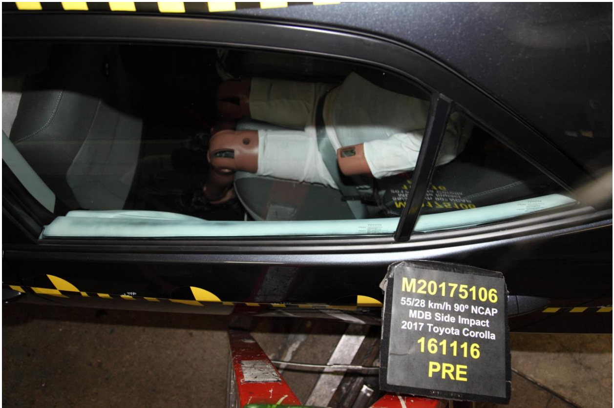
069 Pre-Test Passenger Dummy and Door Clearance View
