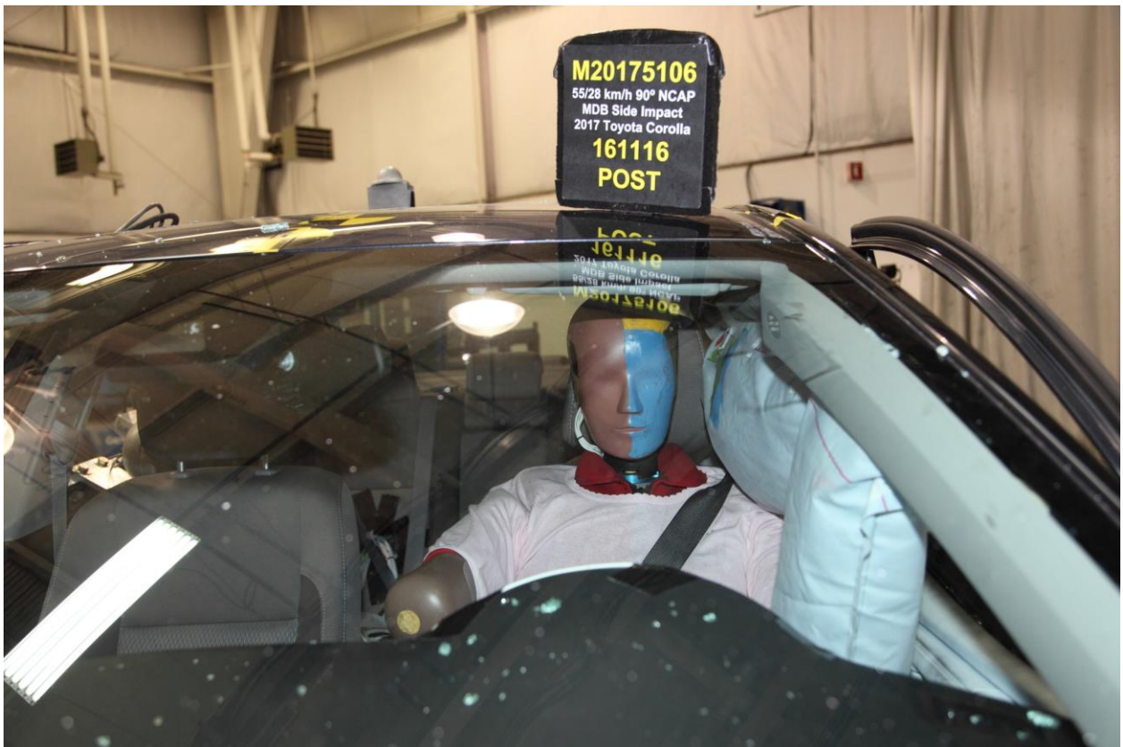
026 Post-Test Front Close-Up View of Driver Dummy
