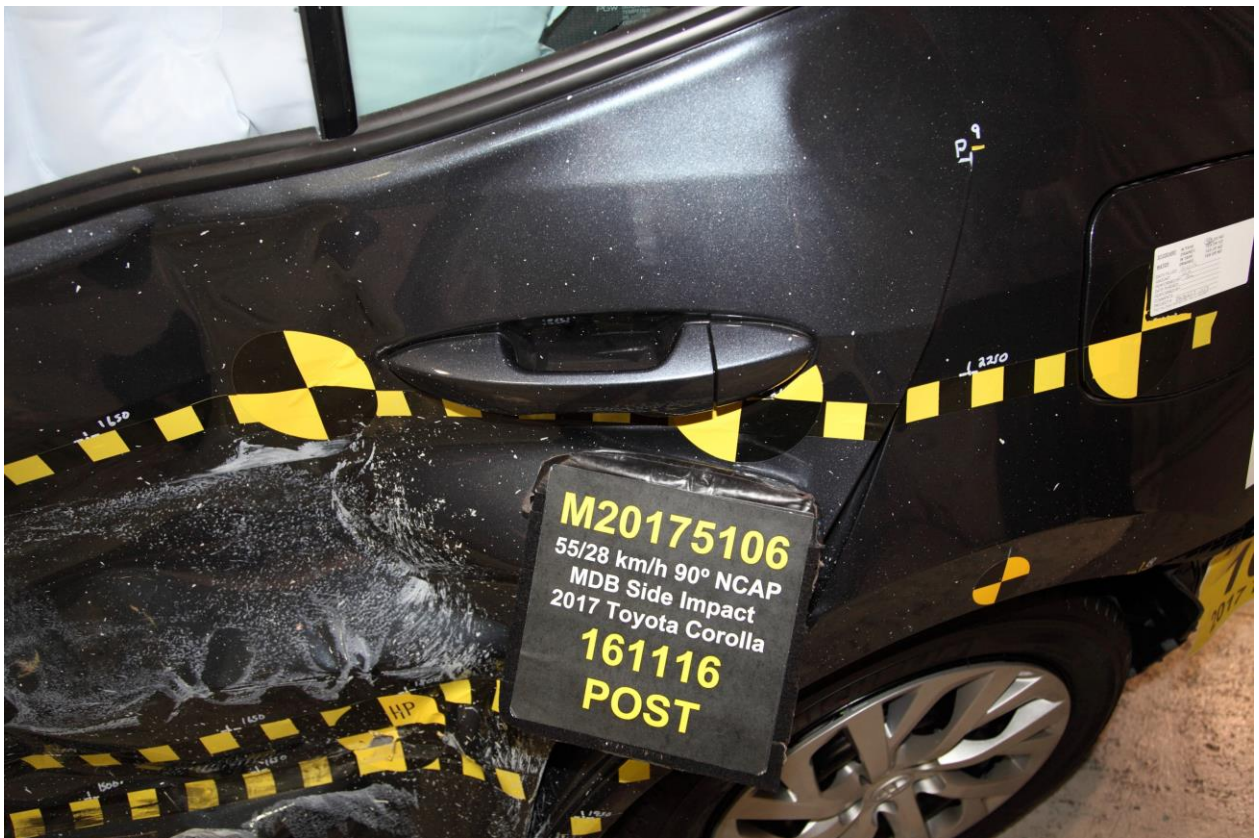
024 Post-Test Left Rear Door Latch Close-Up
