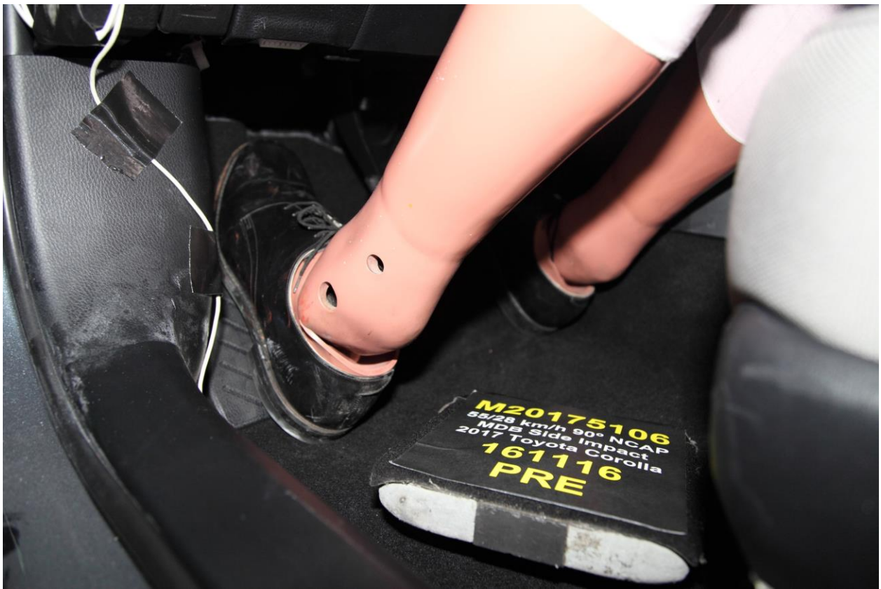
034 Pre-Test Placement of Driver Dummy Feet
