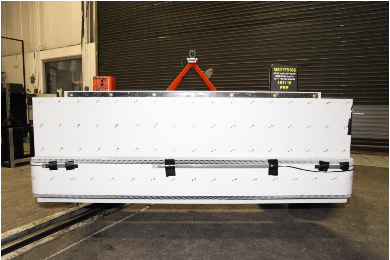
084 Pre-Test Front View of MDB Impactor Face
