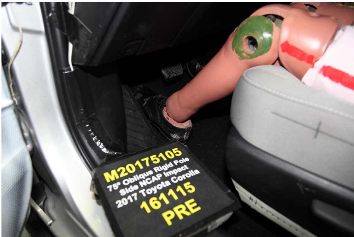
No. 032 Pre-Test Placement of Dummy Feet
