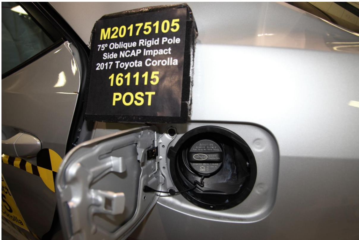
No. 054 Post-Test View of Fuel Filler Cap or Fuel Filler Neck
