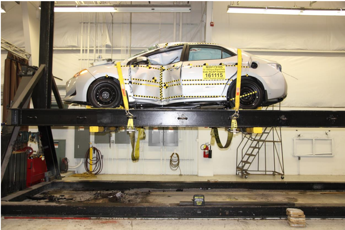
No. 067 FMVSS No. 301 Static Rollover 360 Degrees
