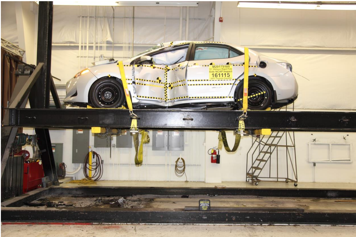
No. 063 FMVSS No. 301 Static Rollover 0 Degrees
