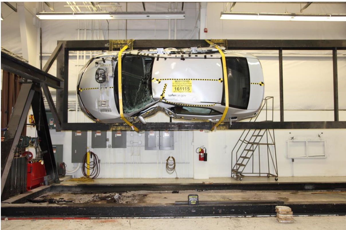
No. 064 FMVSS No. 301 Static Rollover 90 Degrees
