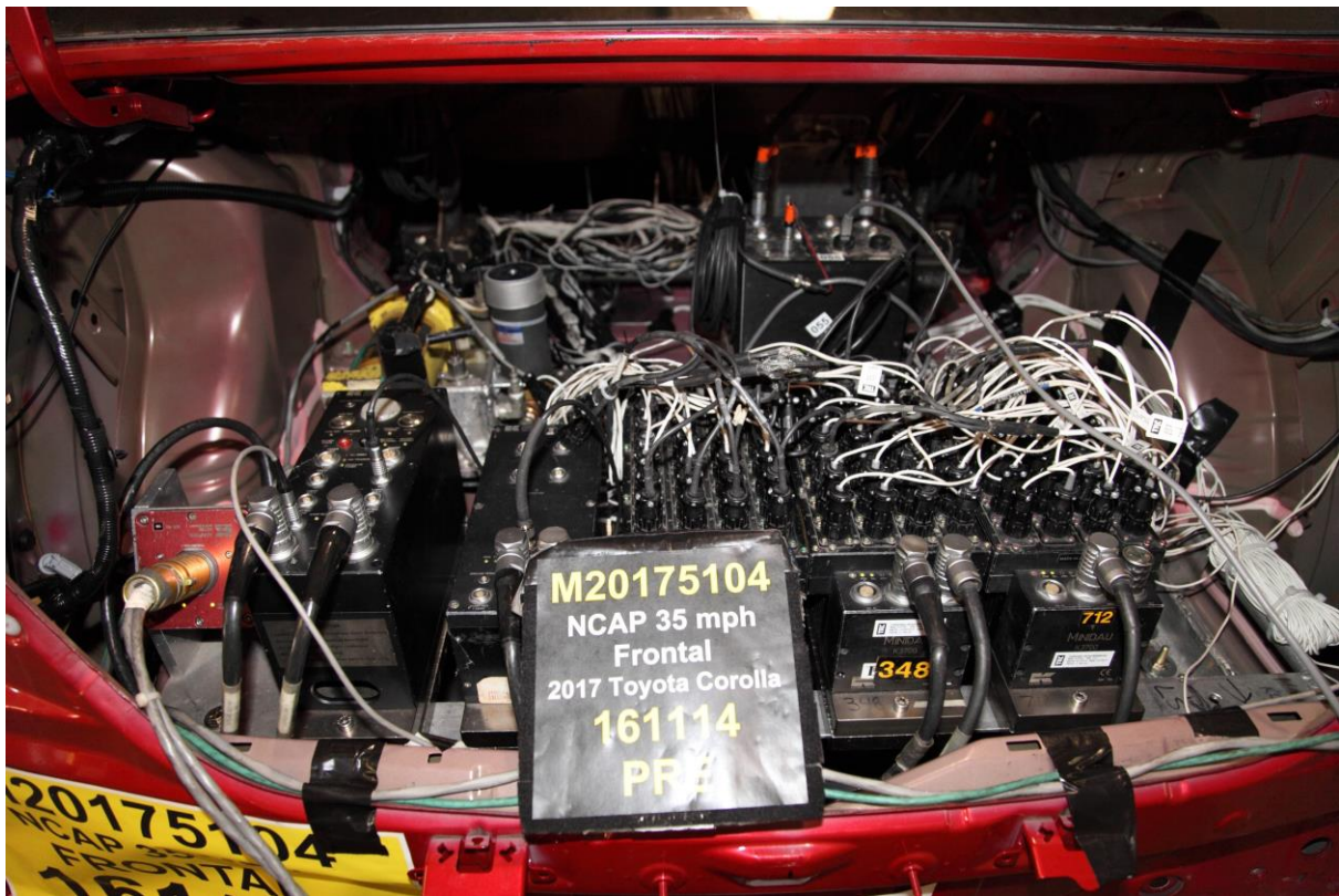
070 Photograph of Ballast Installed in Vehicle View
