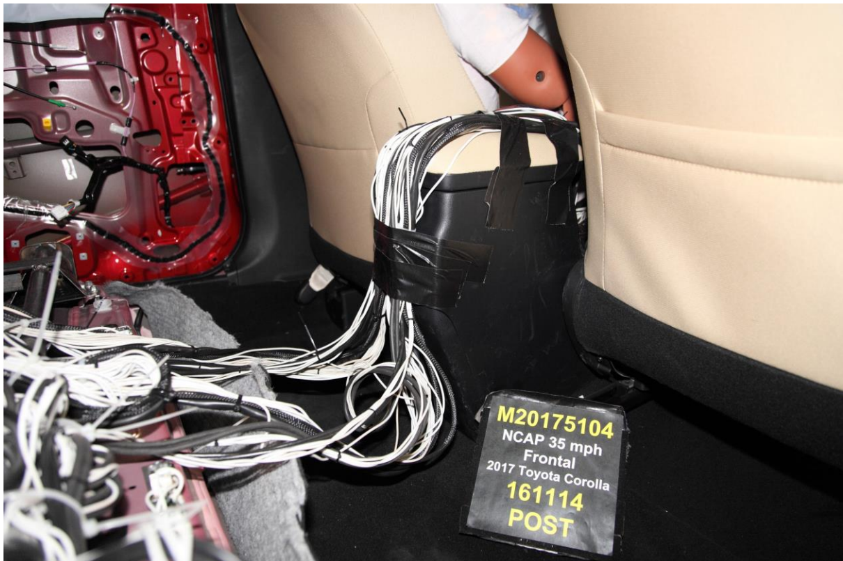
029 Post-Test Dummy Cable Routing
