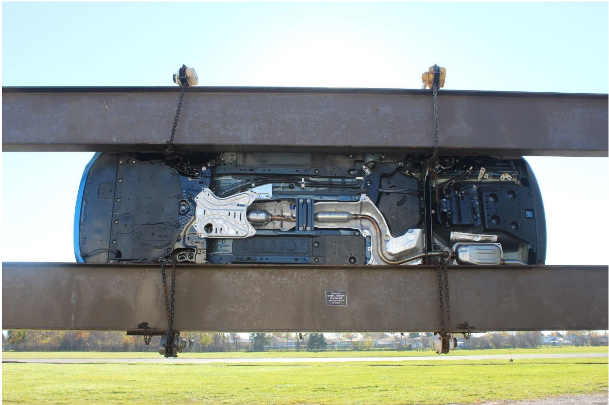
Figure A-99: FMVSS No. 301 Static Rollover 270 Degrees
