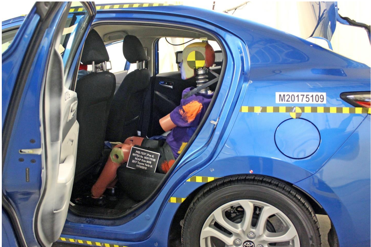
Figure A-55: Pre-Test Left Side View of Passenger Dummy Showing Belt and Chalking
