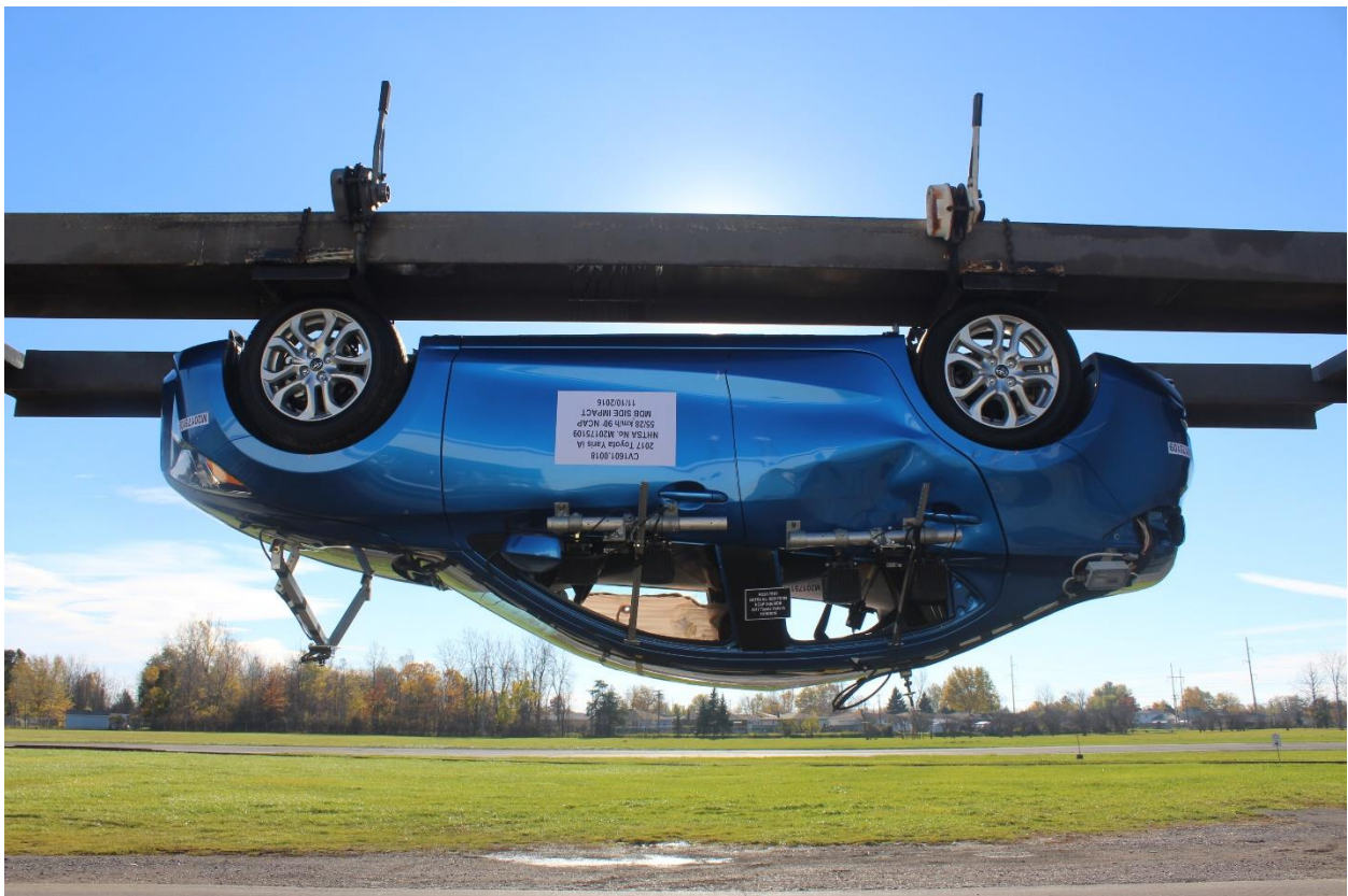
Figure A-98: FMVSS No. 301 Static Rollover 180 Degrees
