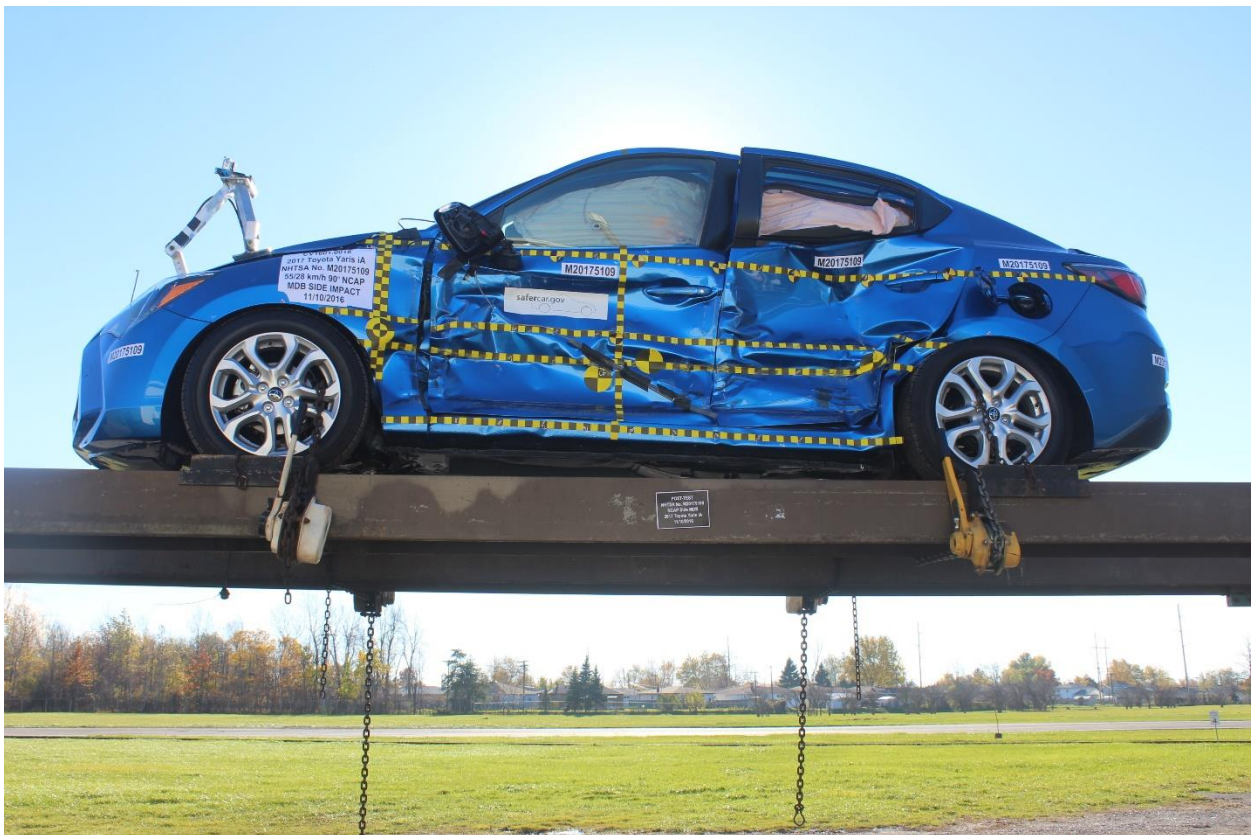
Figure A-100: FMVSS No. 301 Static Rollover 360 Degrees
