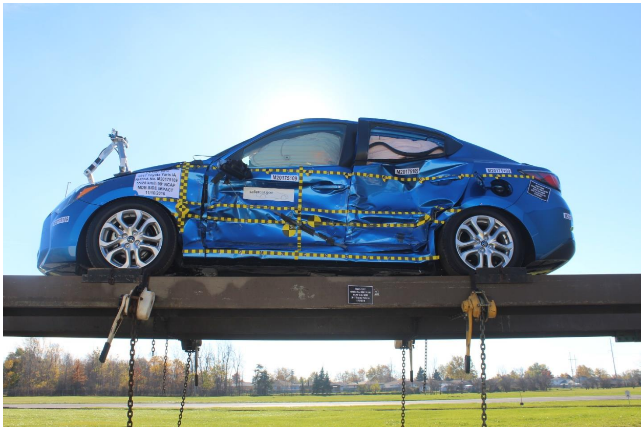
Figure A-96: FMVSS No. 301 Static Rollover 0 Degrees
