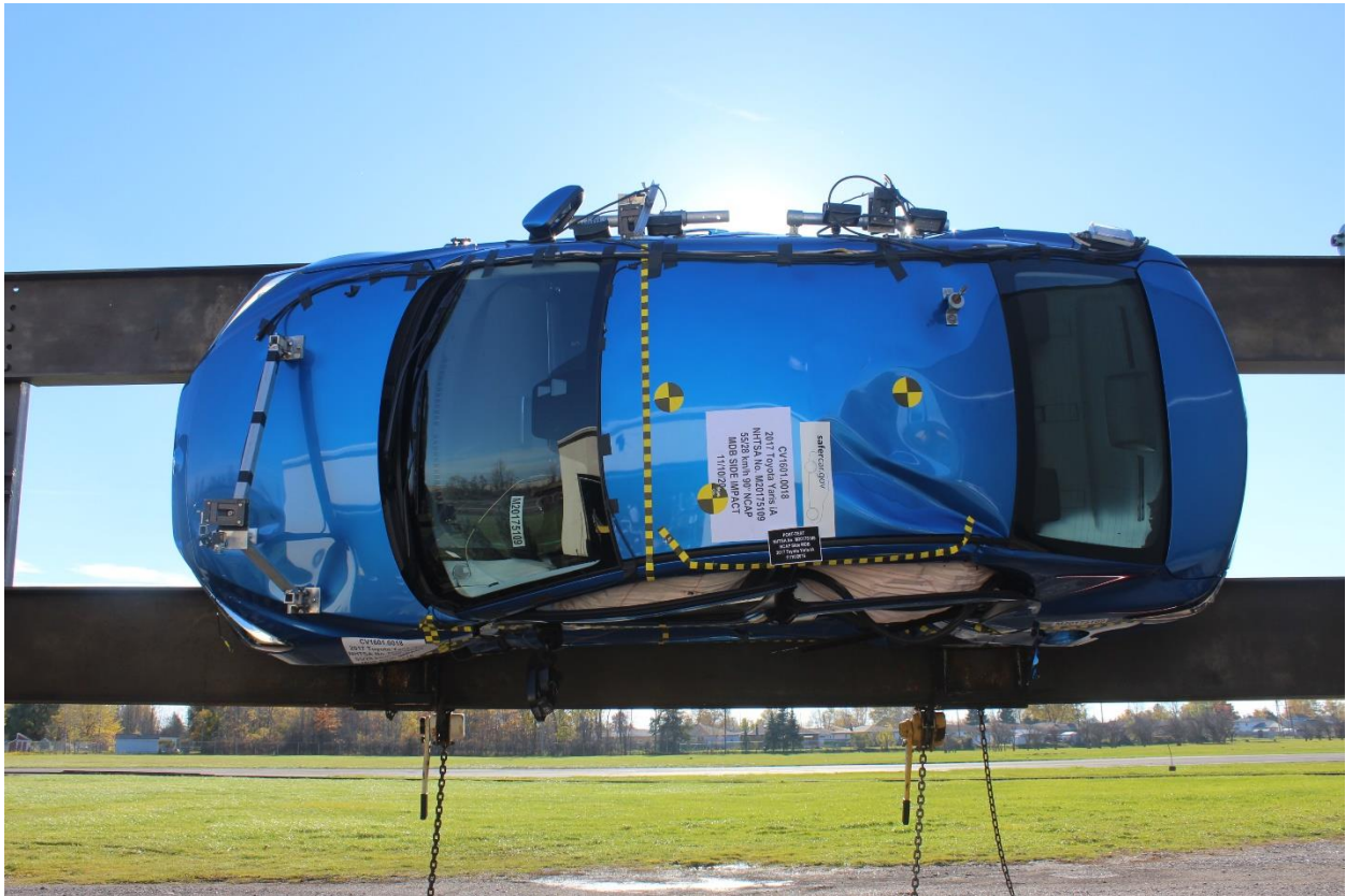
Figure A-97: FMVSS No. 301 Static Rollover 90 Degrees
