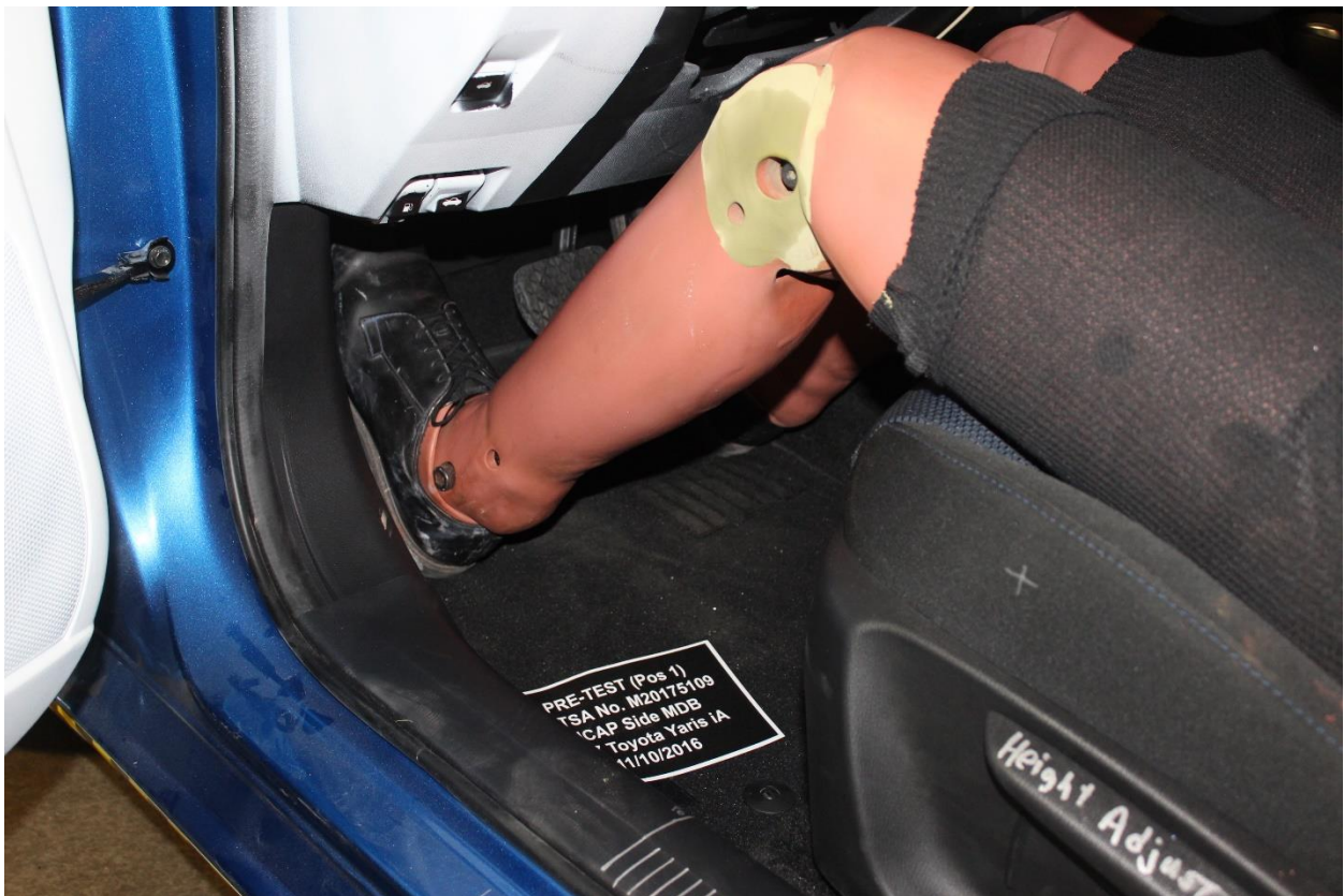
Figure A-34: Pre-Test Placement of Driver Dummy's Feet
