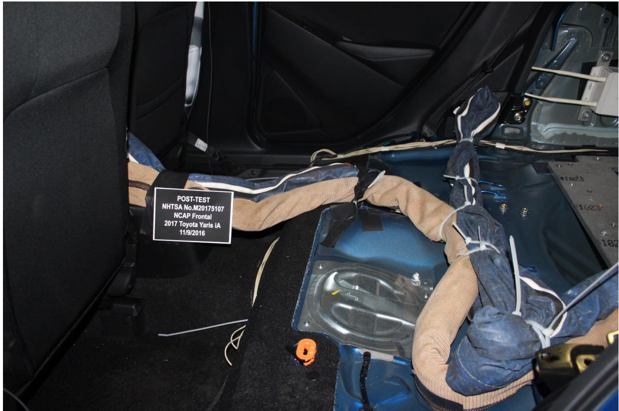
Figure A-29: Post-Test Dummy Cable Routing
