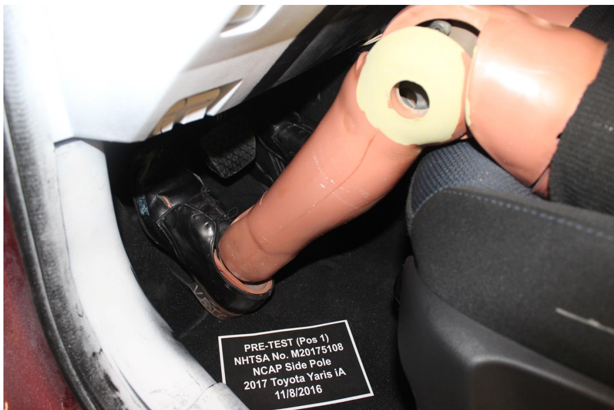
Figure A-32: Pre-Test Placement of Dummy's Feet
