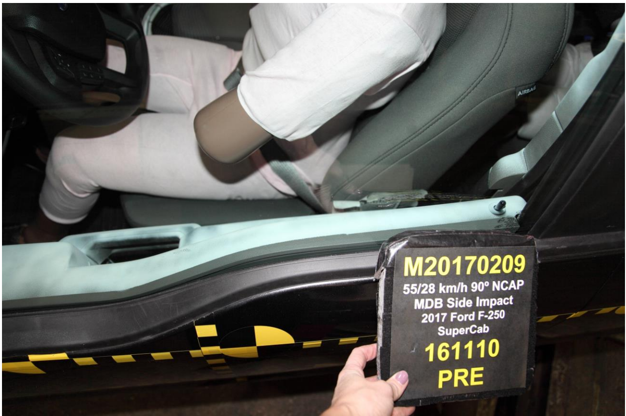
042 Pre-Test Driver Dummy and Door Clearance View
