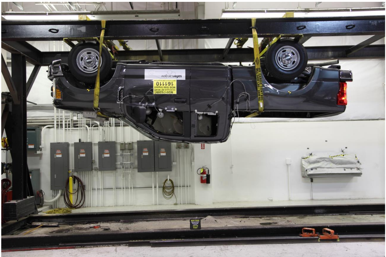
098 FMVSS No. 301 Static Rollover 180 Degrees
