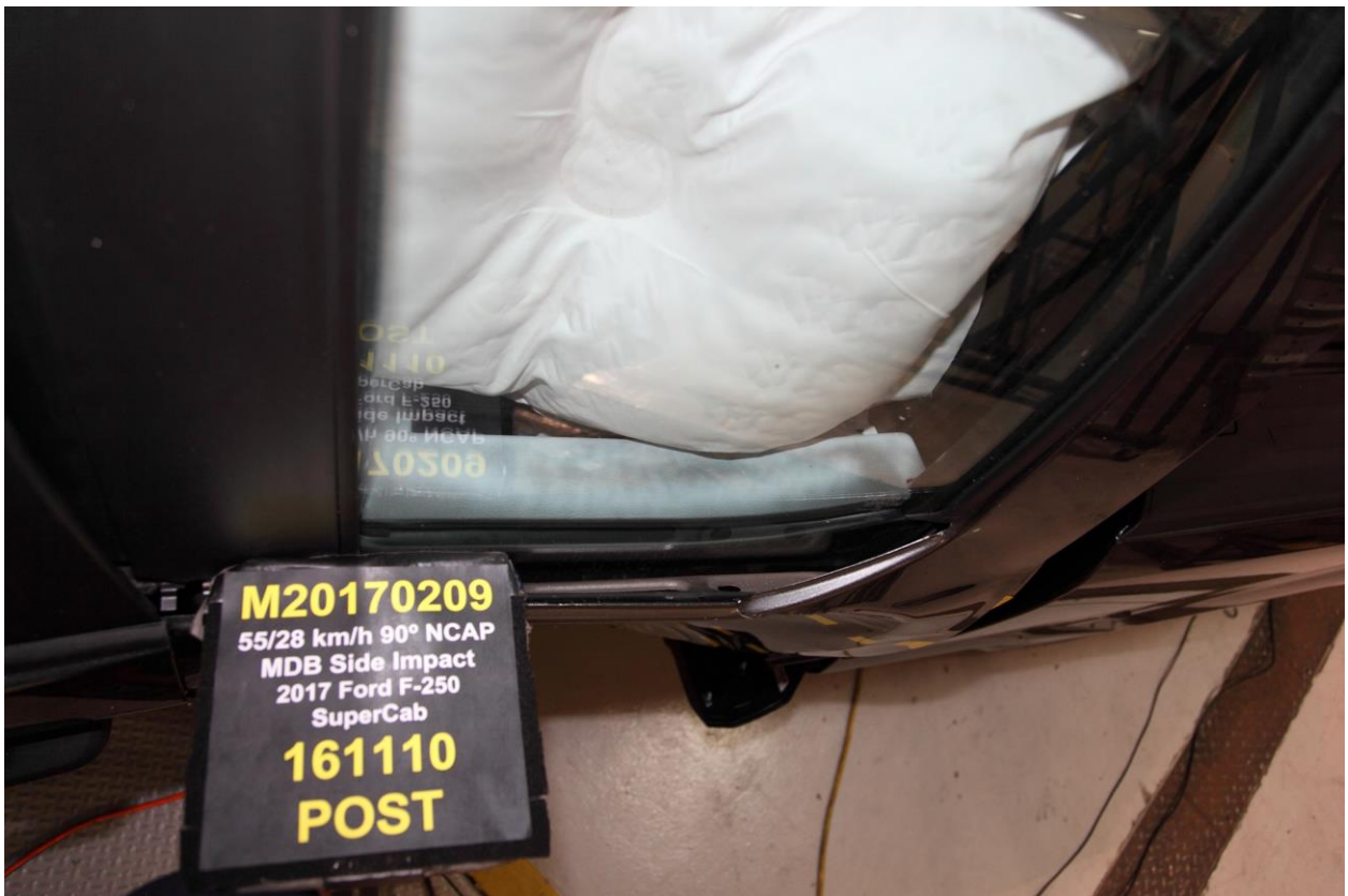
070 Post-Test Passenger Dummy and Door Clearance View
