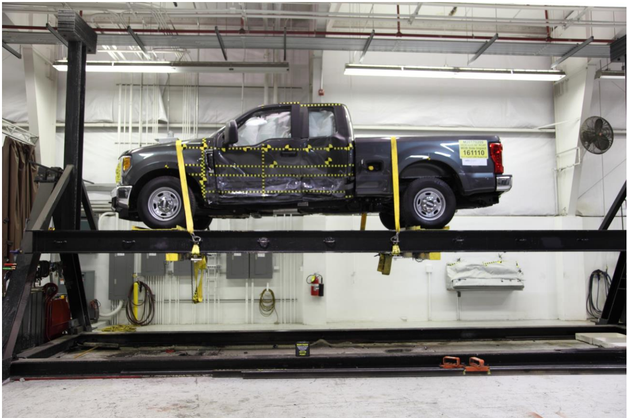
100 FMVSS No. 301 Static Rollover 360 Degrees
