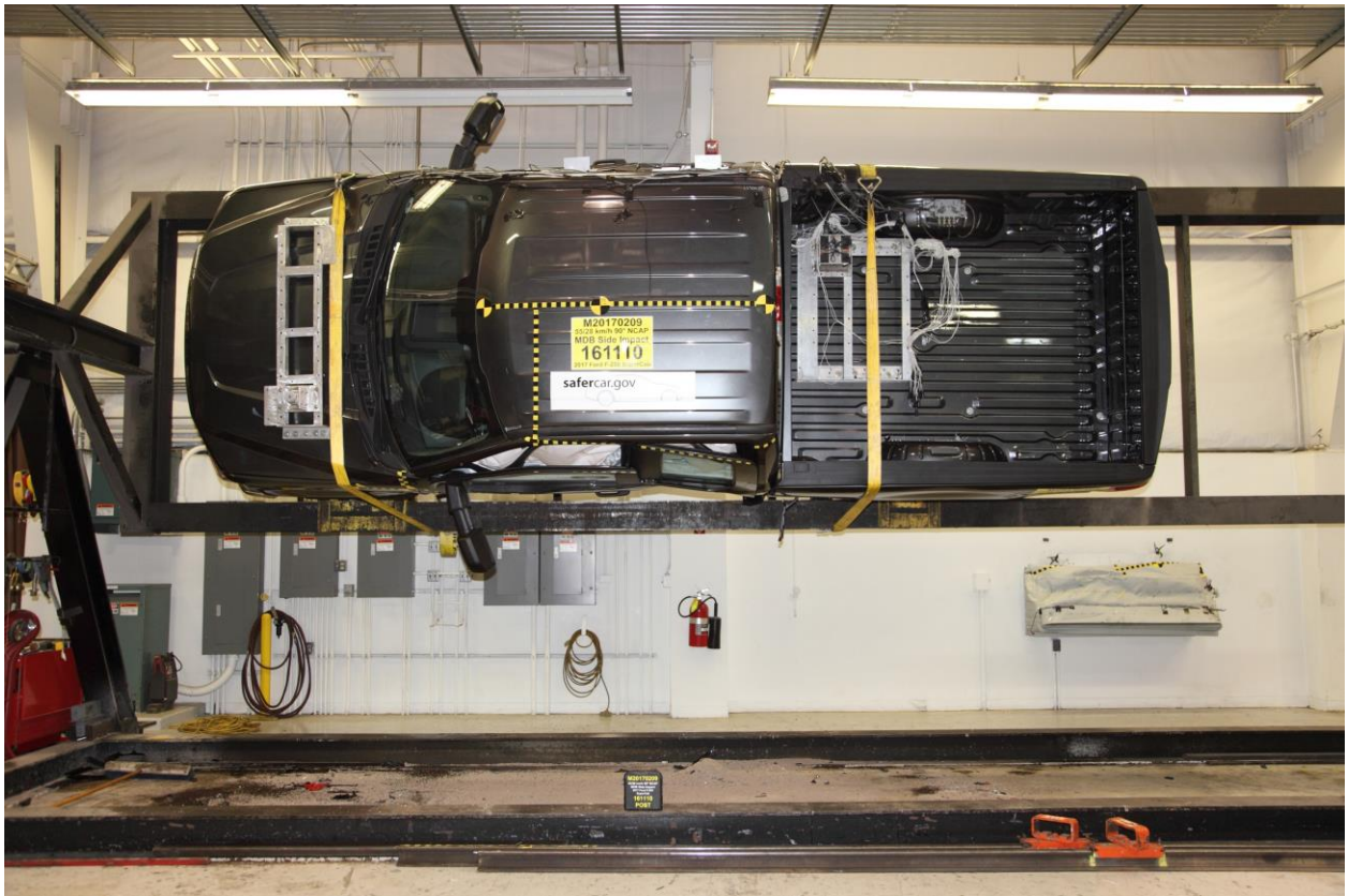
097 FMVSS No. 301 Static Rollover 90 Degrees
