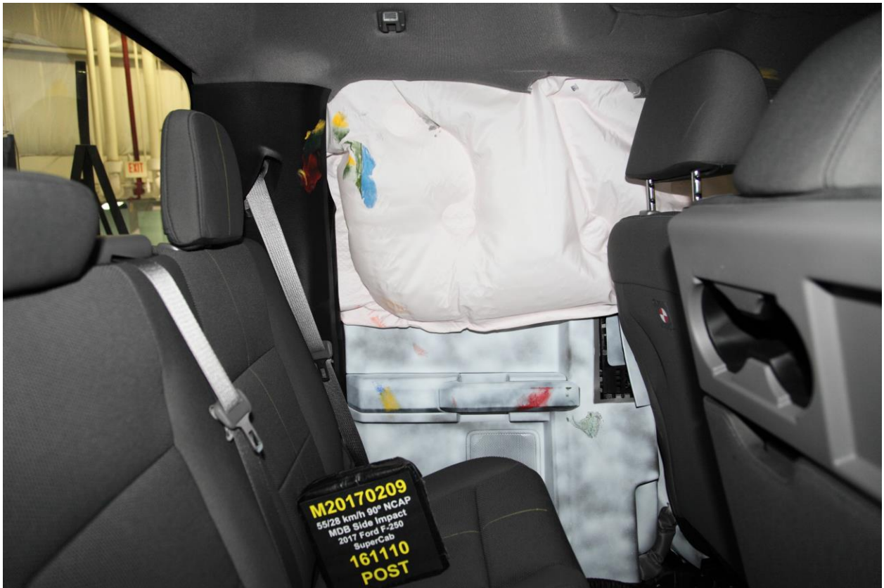
074 Post-Test Passenger Inner Door Panel View
