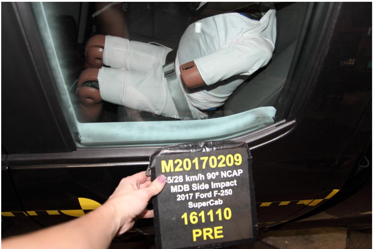
069 Pre-Test Passenger Dummy and Door Clearance View
