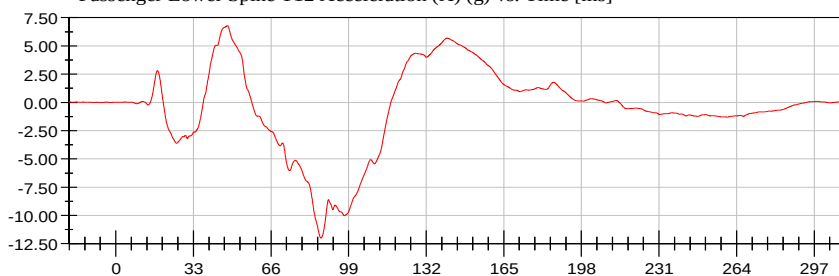
Passenger Lower Spine T12 Acceleration (Y) (g) vs. Time [ms]
