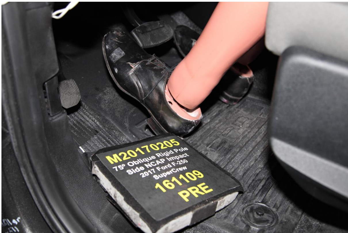
No. 032 Pre-Test Placement of Dummy Feet
