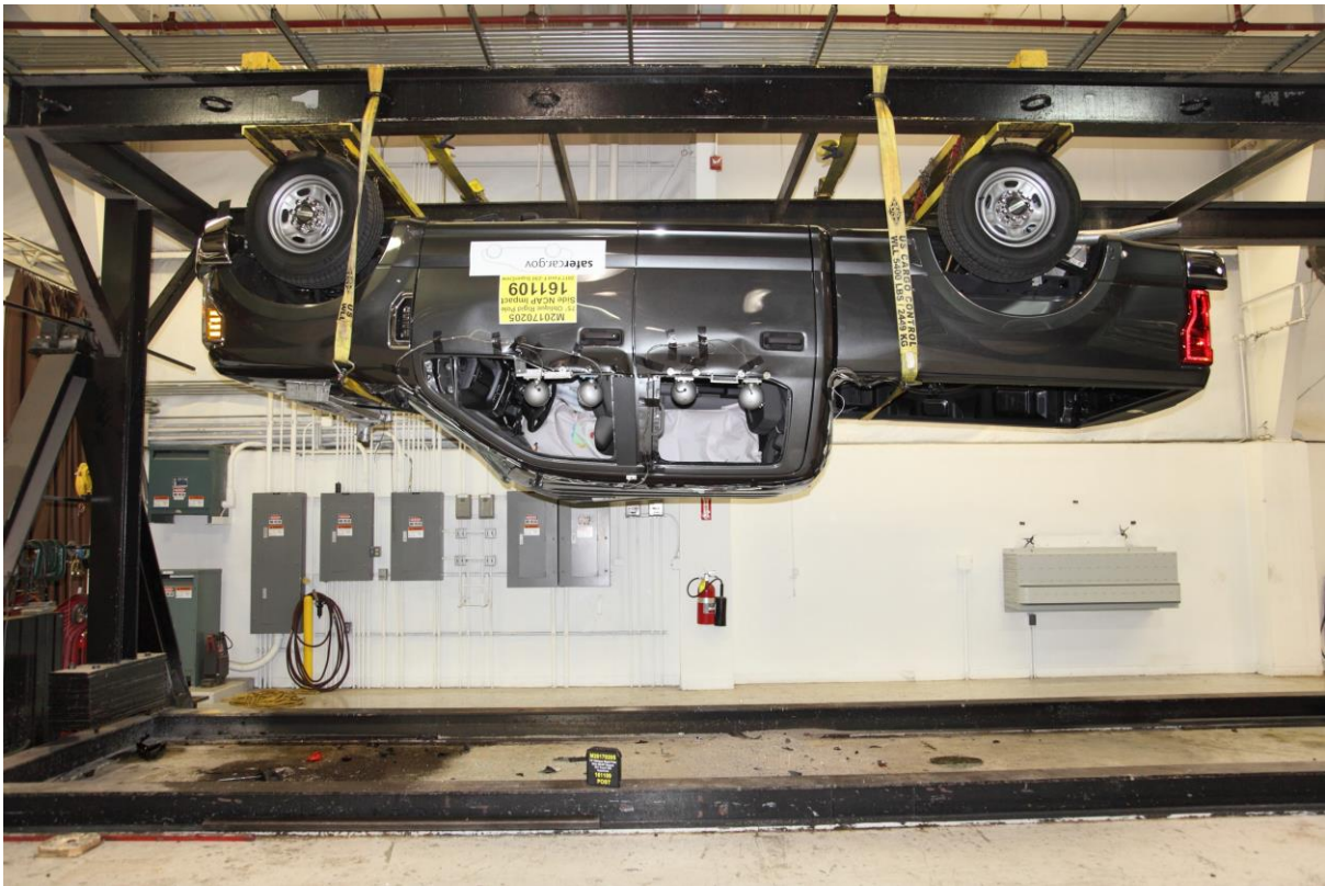
No. 065 FMVSS No. 301 Static Rollover 180 Degrees
