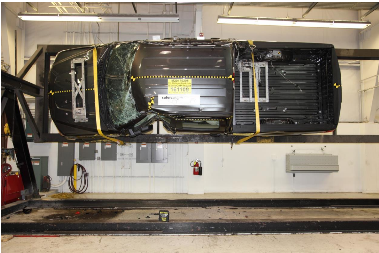
No. 064 FMVSS No. 301 Static Rollover 90 Degrees
