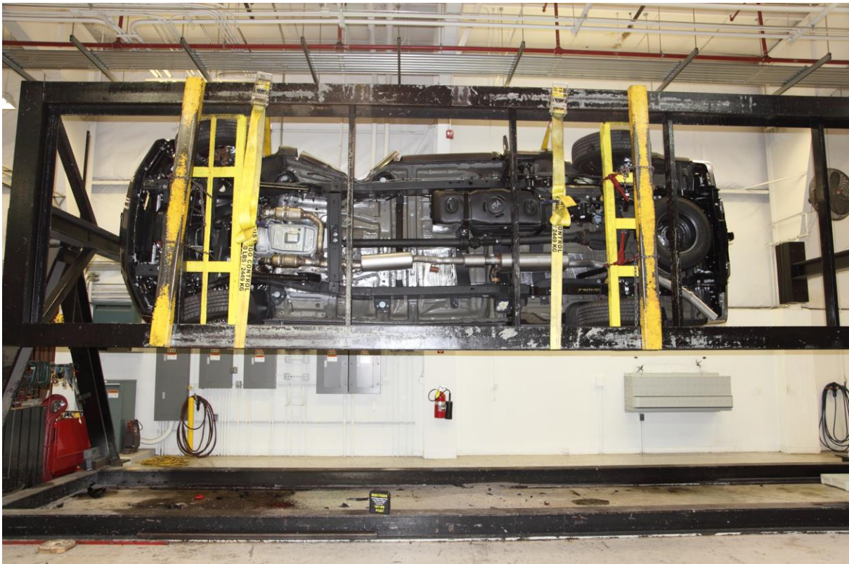
No. 066 FMVSS No. 301 Static Rollover 270 Degrees
