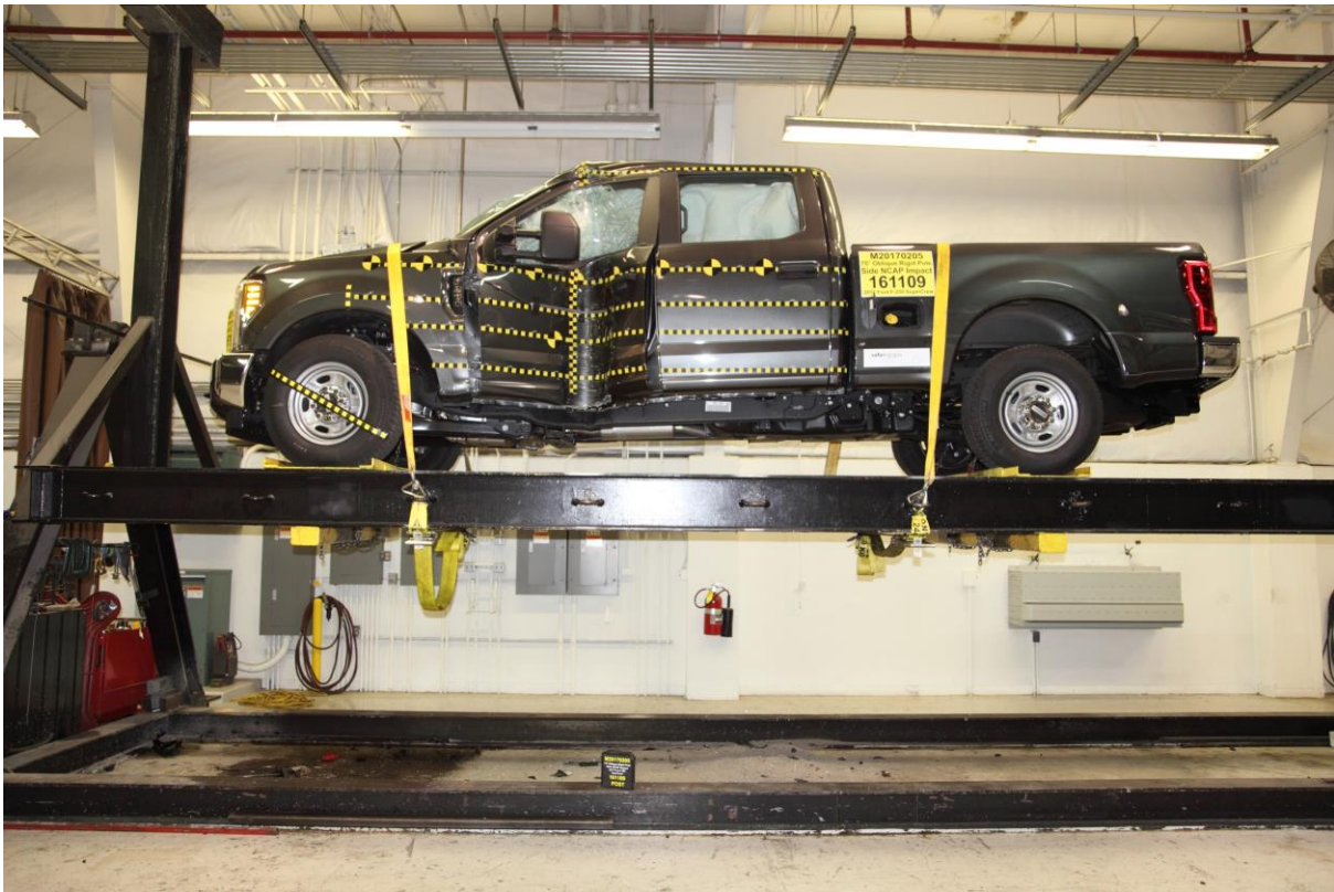
No. 063 FMVSS No. 301 Static Rollover 0 Degrees
