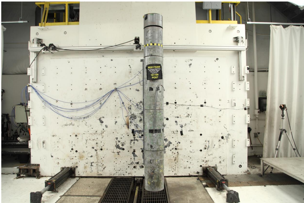
No. 058 Post-Test Pole Barrier Front View
