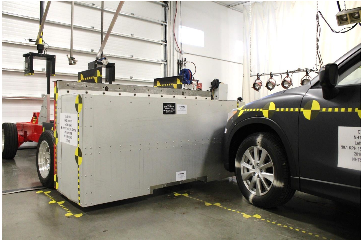
No. 193: Pre-Test OMDB & Vehicle Alignment
