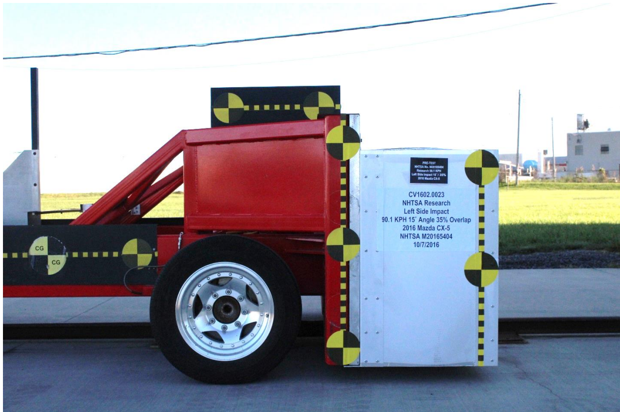
No. 169: Pre-Test Right Side View of OMDB
