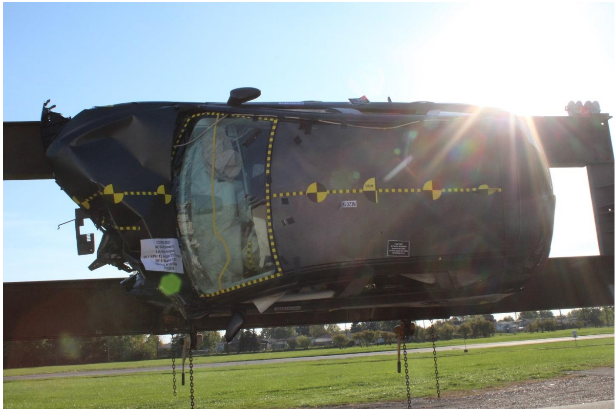
No. 195: Vehicle at 90 Degrees on Static Rollover Device
