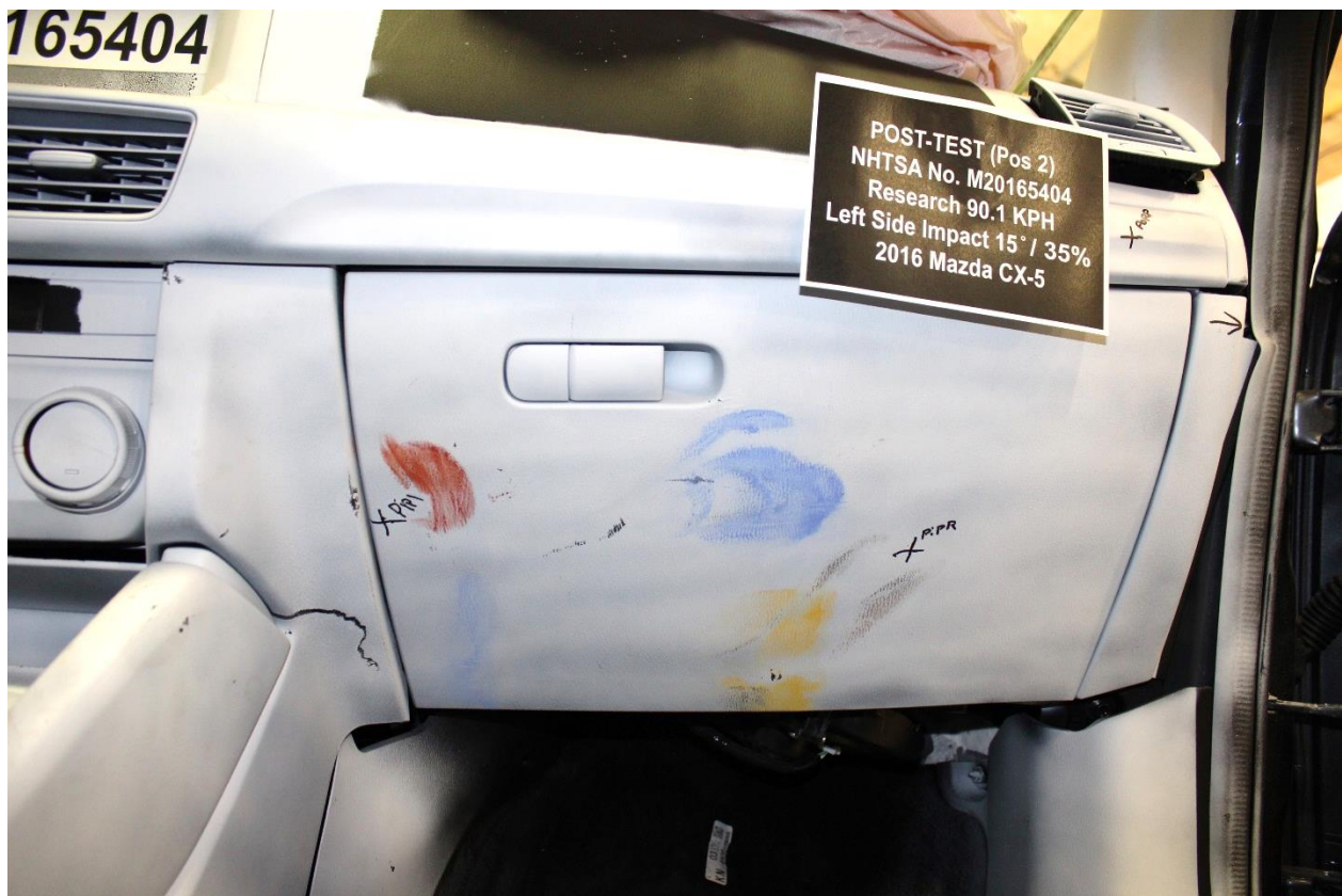
No. 123: Post-Test Passenger Contact With Glovebox
