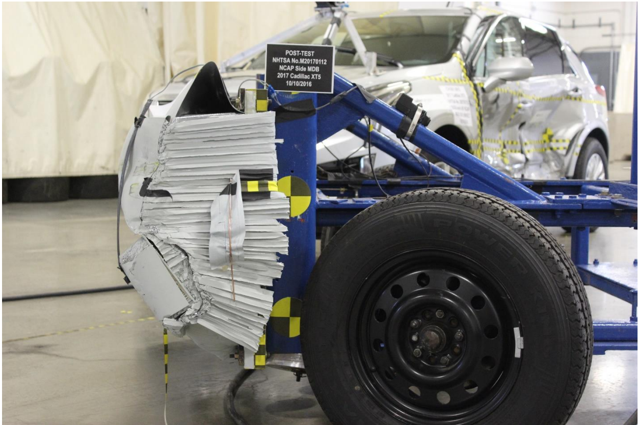
Figure A-89: Post-Test Left Side View of MDB Impactor Face
