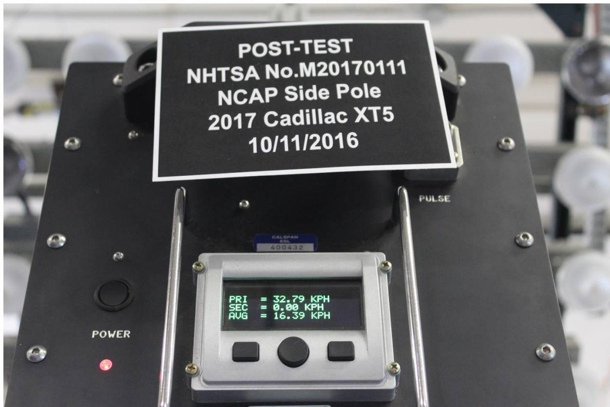
Figure A-62: Post-Test Primary and Redundant Speed Trap Read-Out
