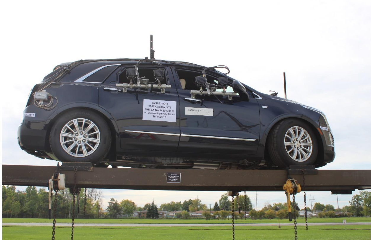
Figure A-63: FMVSS No. 301 Static Rollover 0 Degrees
