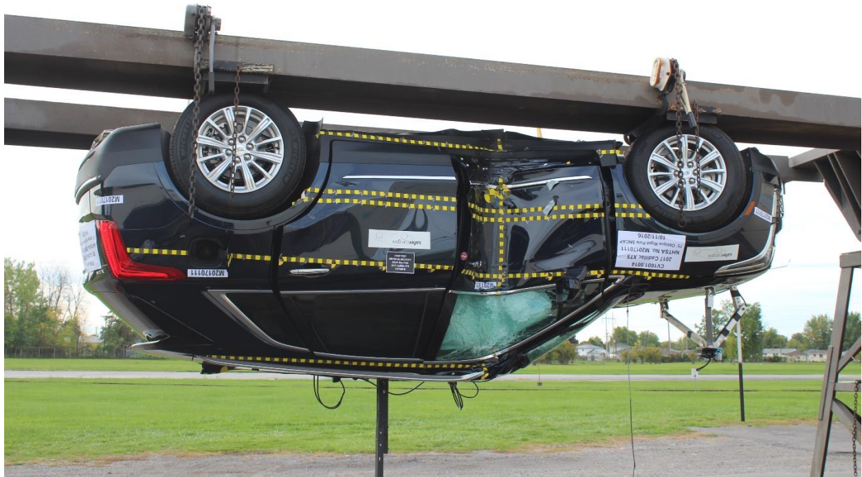
Figure A-65: FMVSS No. 301 Static Rollover 180 Degrees
