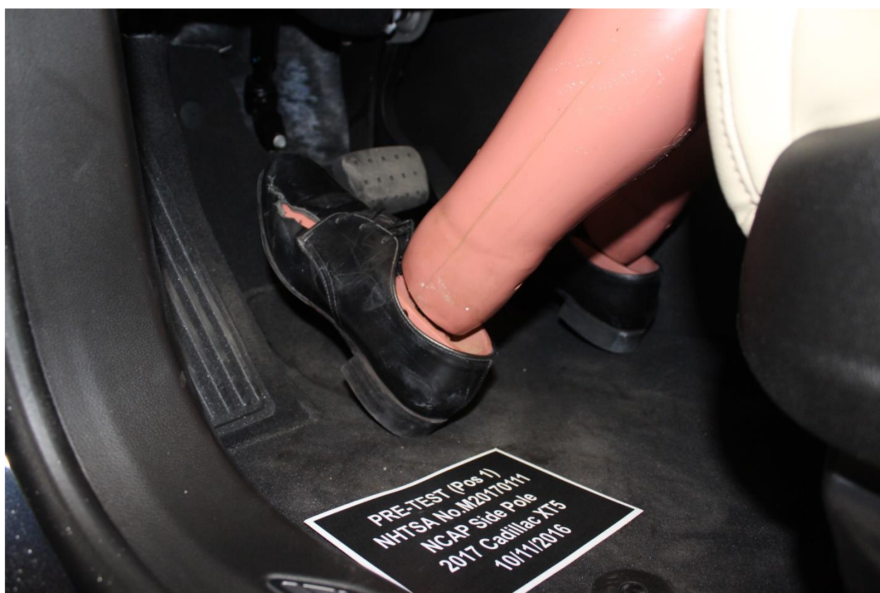
Figure A-32: Pre-Test Placement of Dummy's Feet
