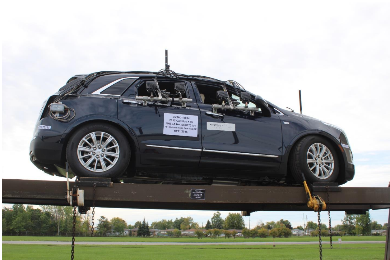
Figure A-67: FMVSS No. 301 Static Rollover 360 Degrees
