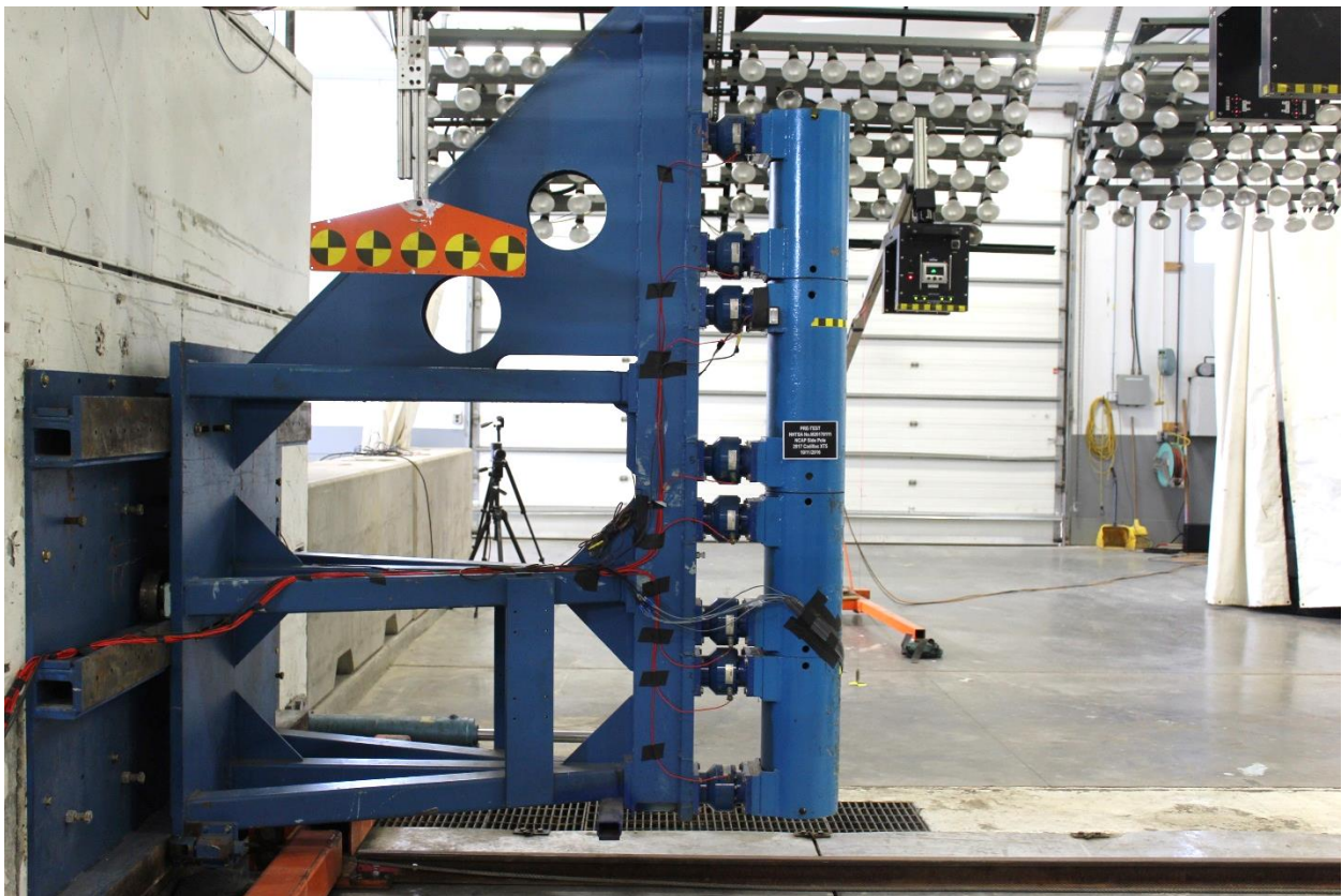
Figure A-59: Pre-Test Pole Barrier Side View
