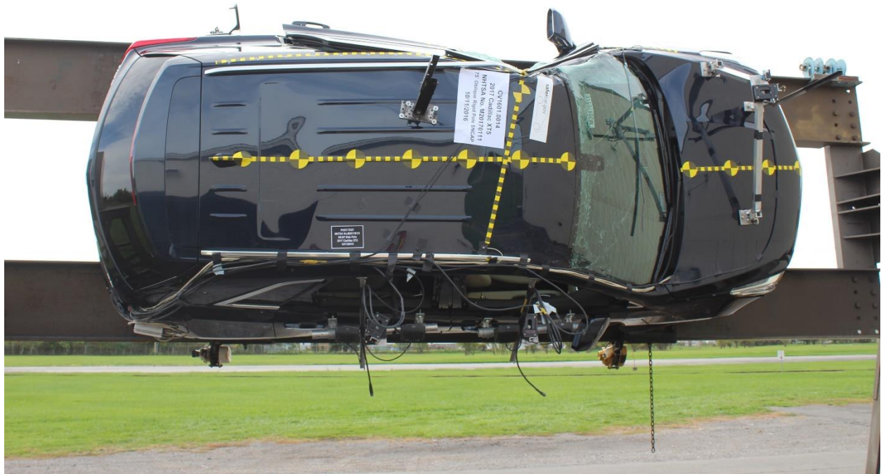
Figure A-66: FMVSS No. 301 Static Rollover 270 Degrees
