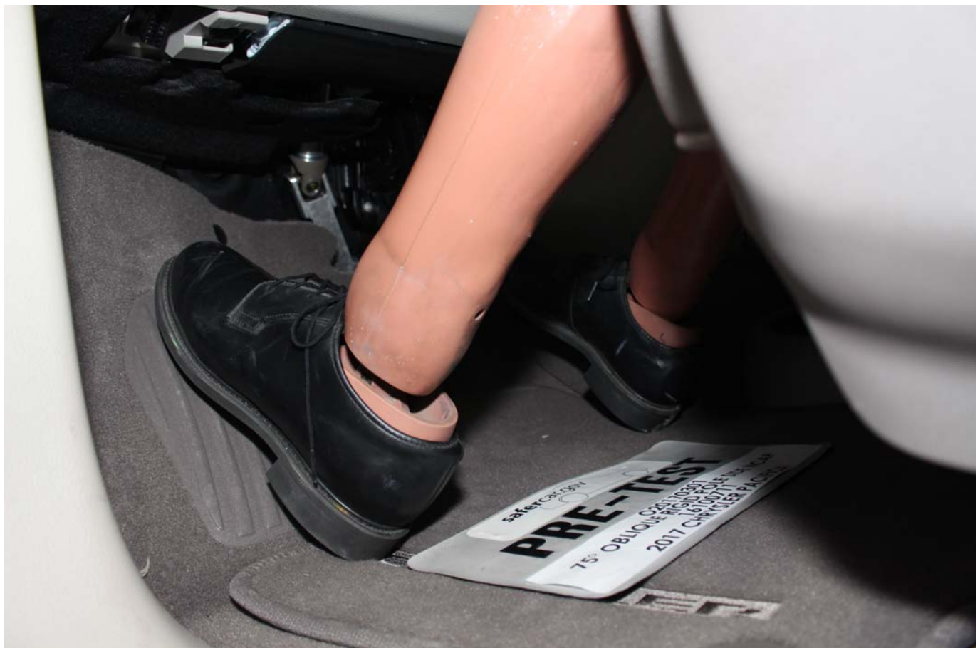
Photo No. 032 - Pre-Test Placement of Dummy's Feet
