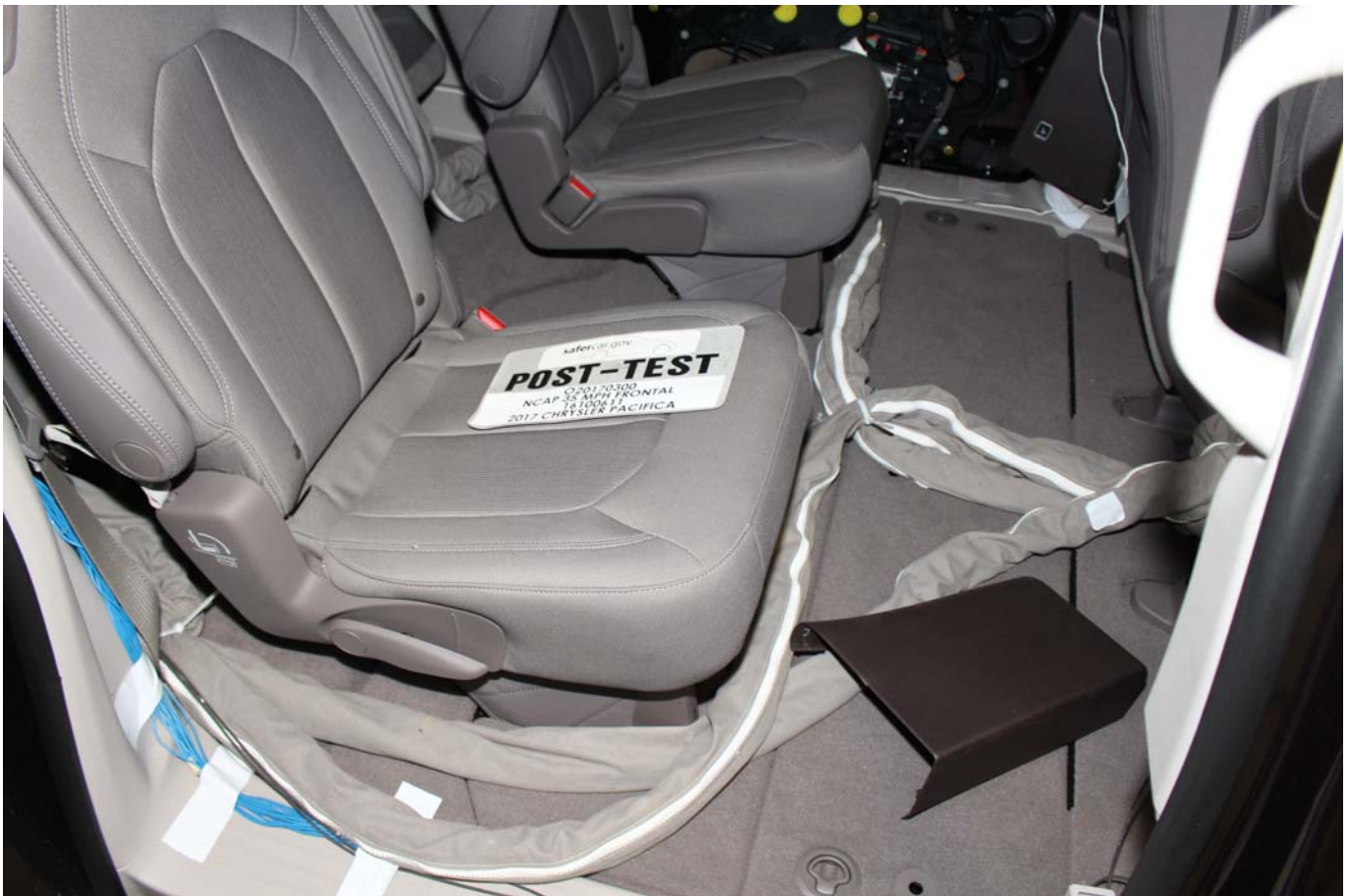
Photo No. 029 - Post-Test Dummy Cable Routing
