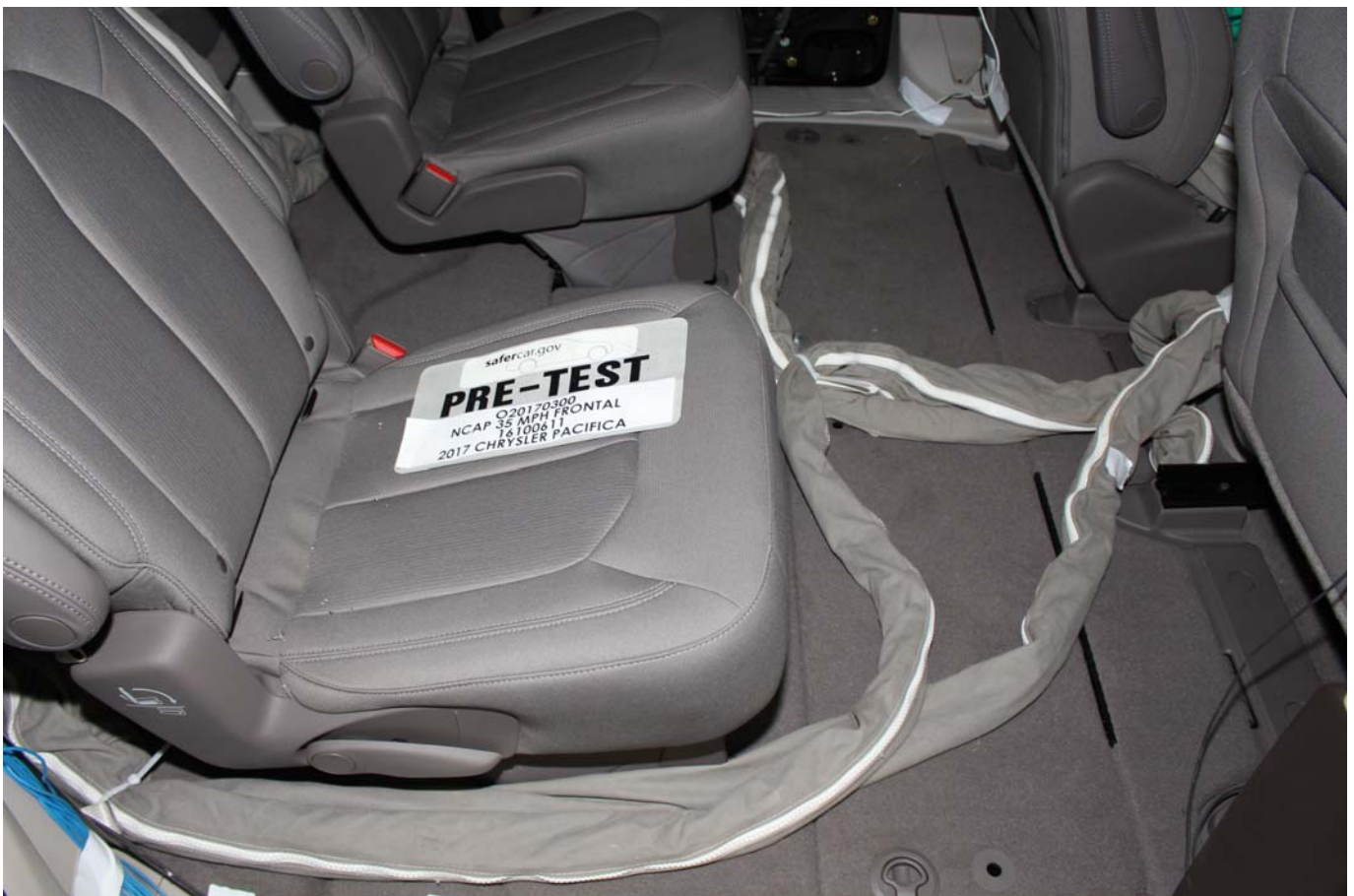
Photo No. 028 - Pre-Test Dummy Cable Routing
