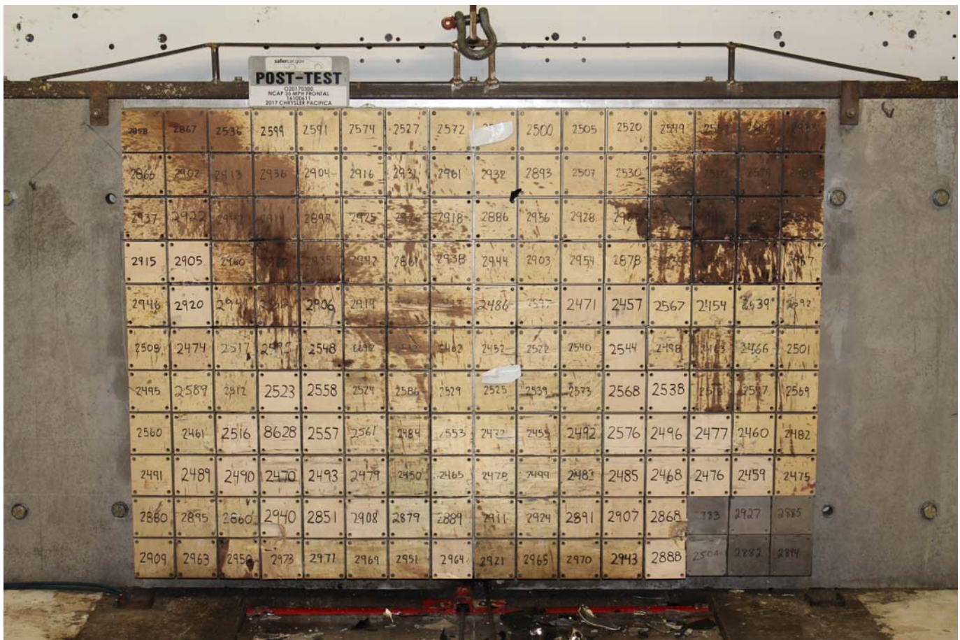
Photo No. 003 - Post-Test Load Cell Wall
