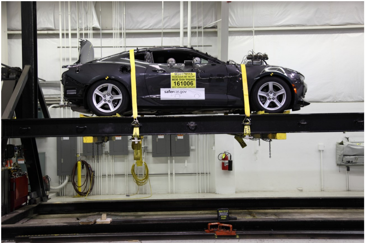
100 FMVSS No. 301 Static Rollover 360 Degrees
