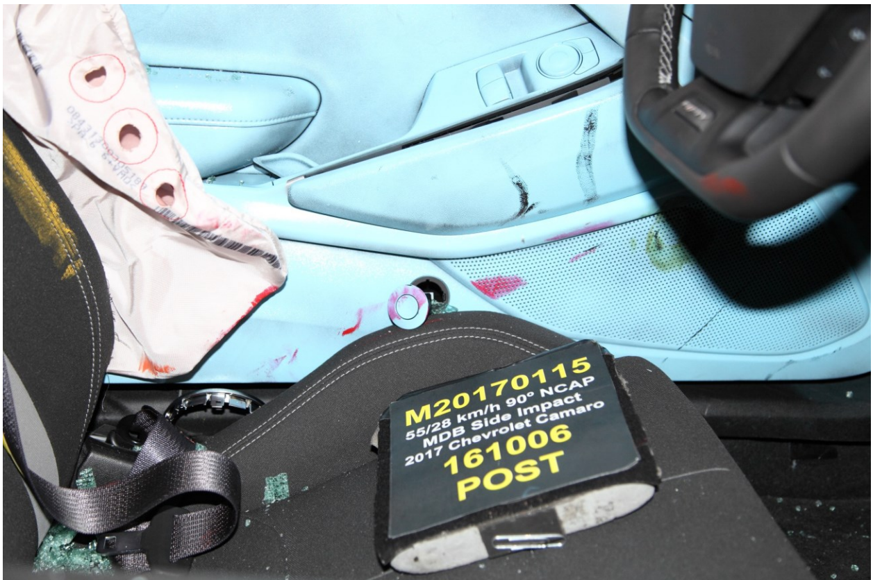
052 Post-Test Driver Dummy Close-Up Pelvis Contact View
