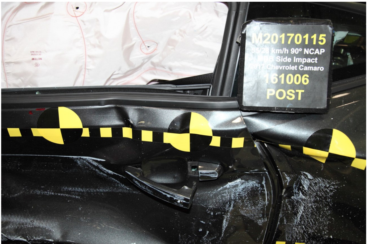
022 Post-Test Left Front Door Latch Close-Up
