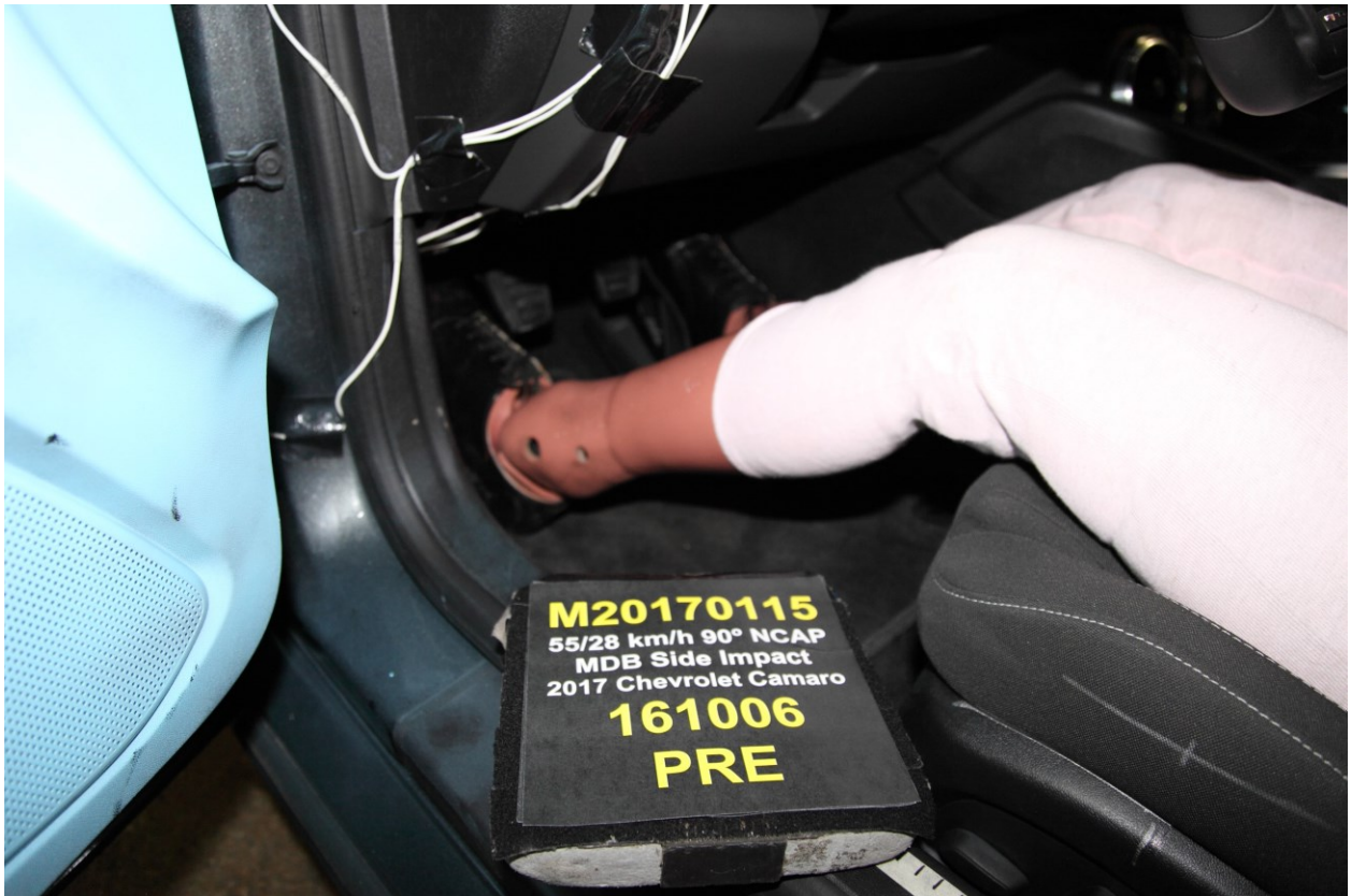
034 Pre-Test Placement of Driver Dummy Feet
