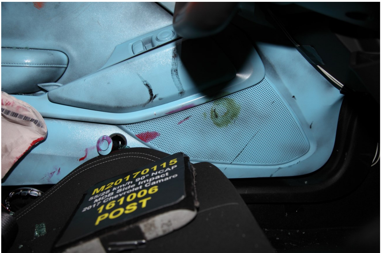
054 Post-Test Driver Dummy Close-Up Knee Contact View
