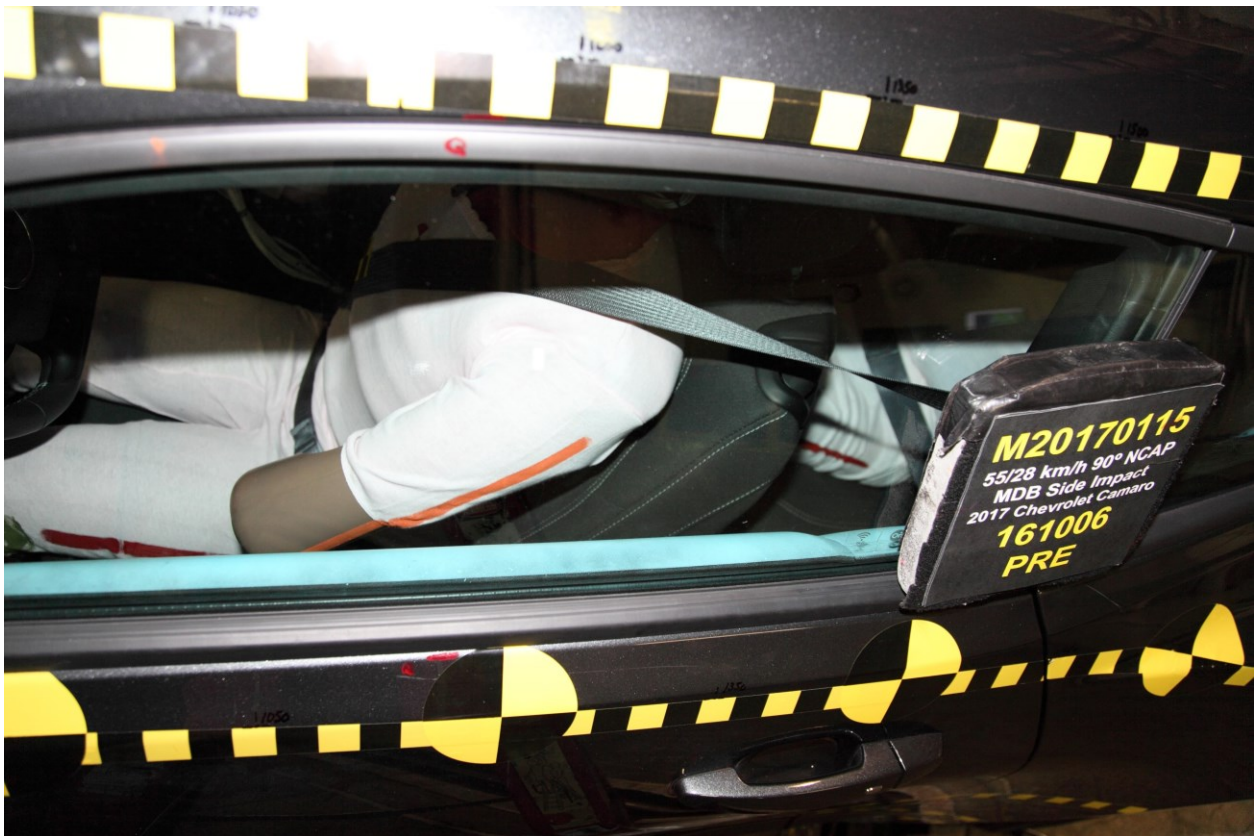
042 Pre-Test Driver Dummy and Door Clearance View
