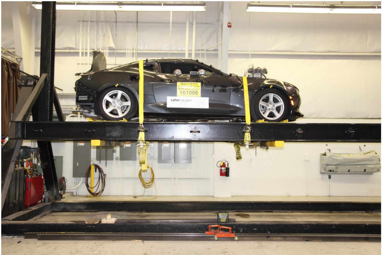
096 FMVSS No. 301 Static Rollover 0 Degrees
