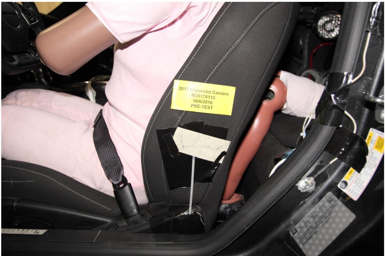
064 Pre-Test Placement of Rear Passenger Dummy Feet
