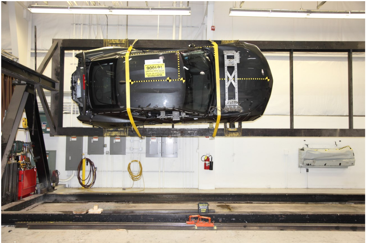
097 FMVSS No. 301 Static Rollover 90 Degrees
