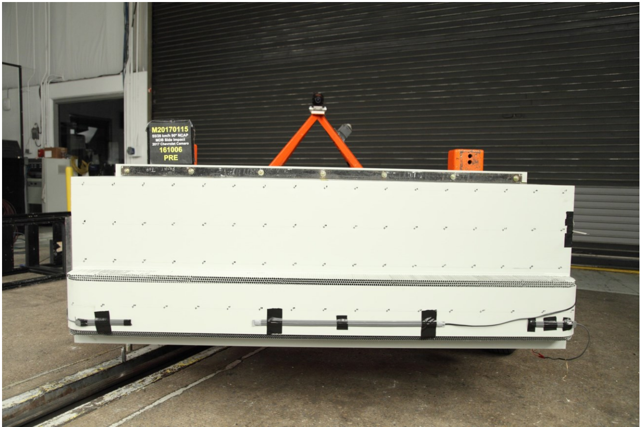
084 Pre-Test Front View of MDB Impactor Face
