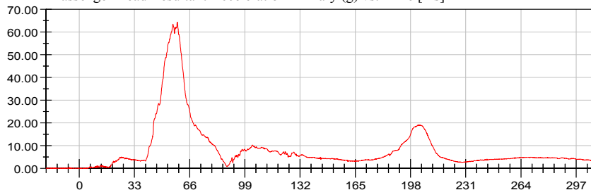
Passenger Lower Spine T12 Acceleration (X) (g) vs. Time [ms]
