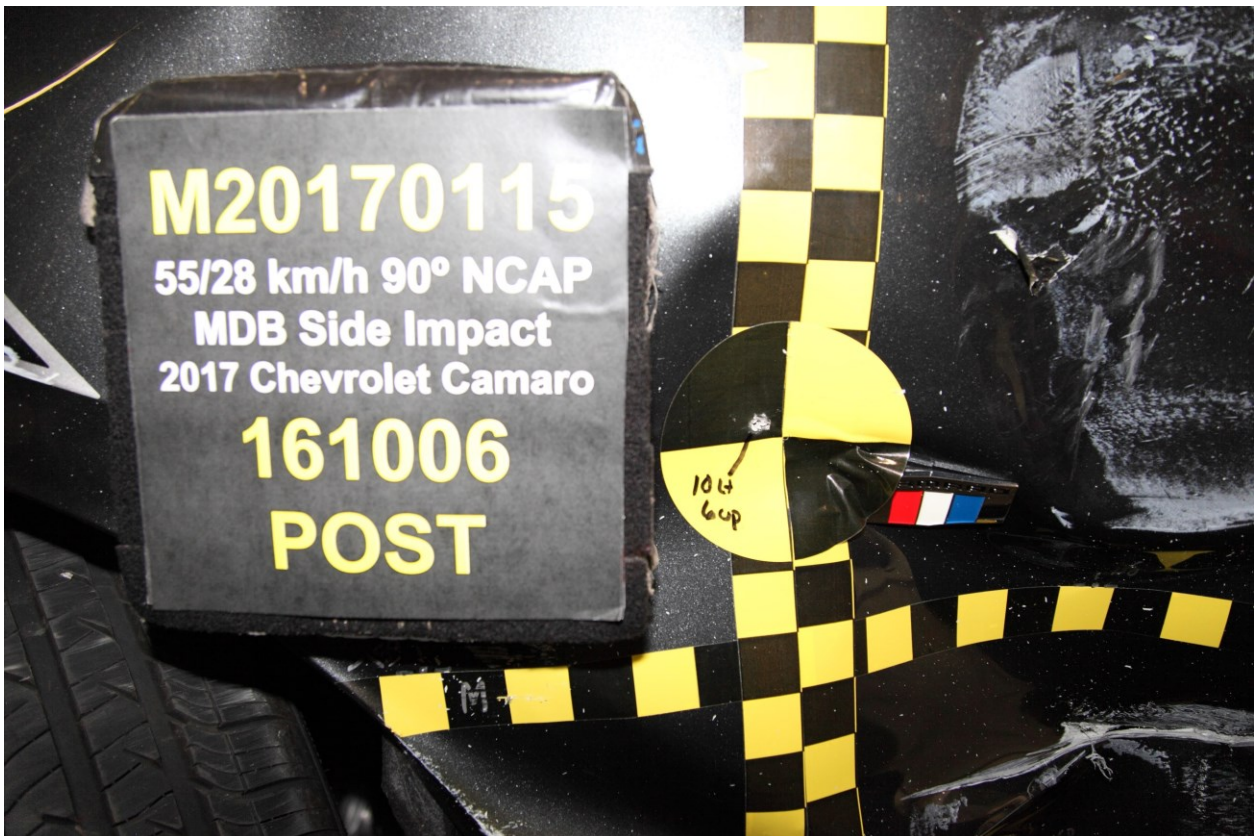
020 Post-Test Close-Up View of Impact Point Target
