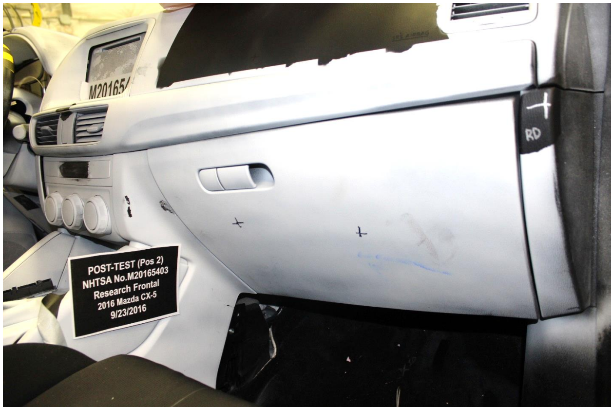
Figure A-63: Post-Test Passenger's Side Knee Bolster
