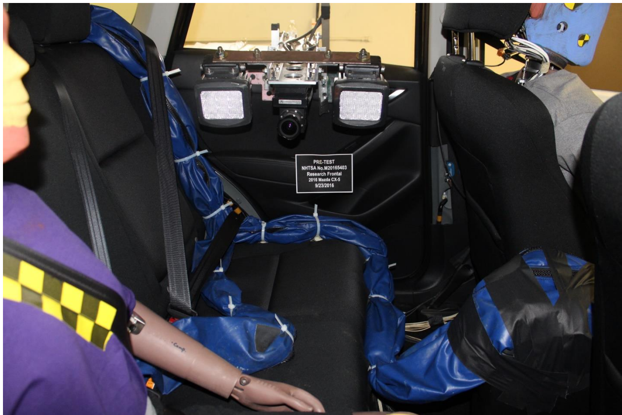
Figure A-27: Pre-Test Dummy Cable Routing
