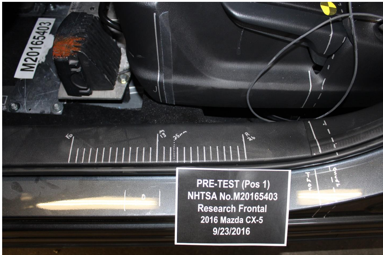
Figure A-35: Pre-Test Driver's Seat Fore-Aft Markings
