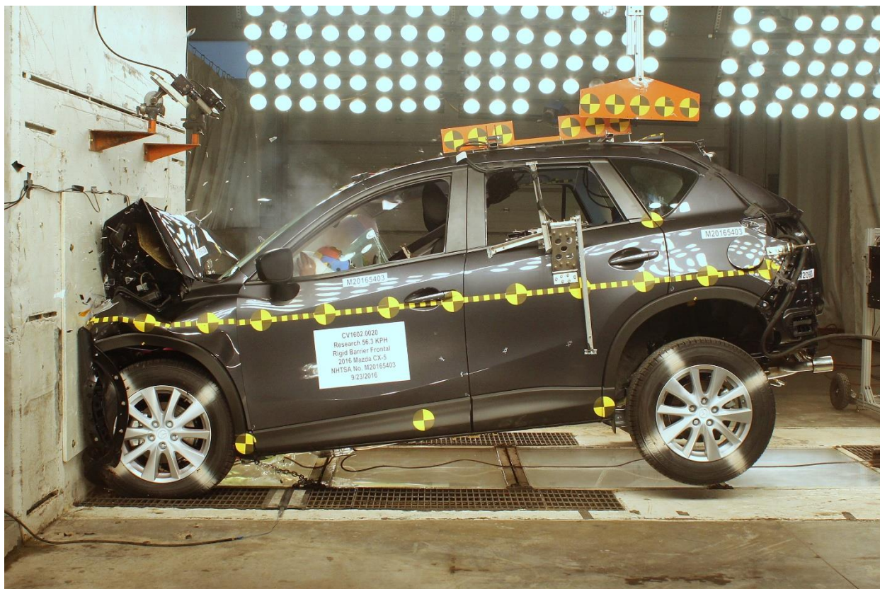
Figure A-77: 2016 Mazda CX-5 Frontal Impact Event
