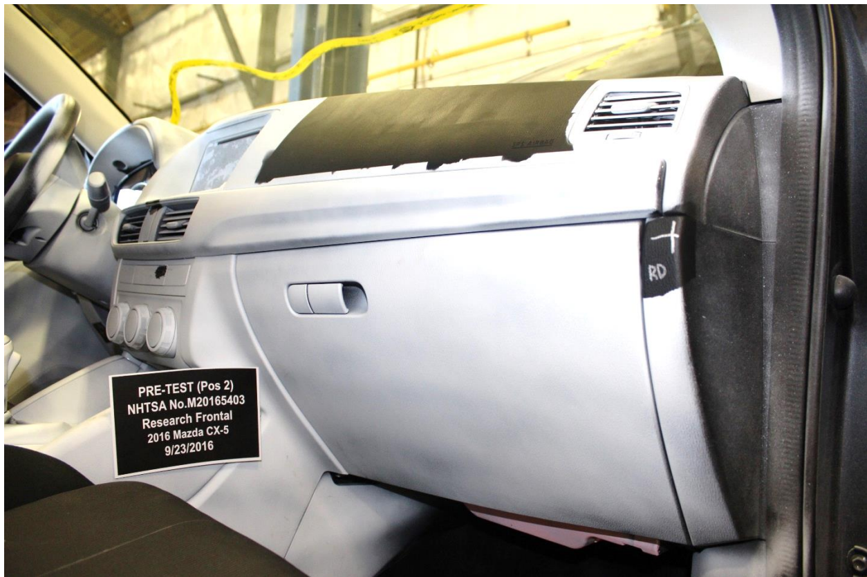
Figure A-62: Pre-Test Passenger's Side Knee Bolster
