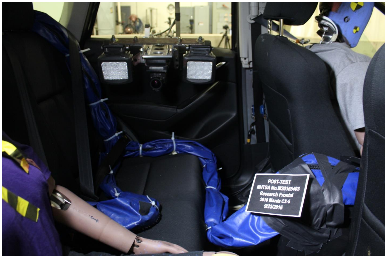
Figure A-28: Post-Test Dummy Cable Routing
