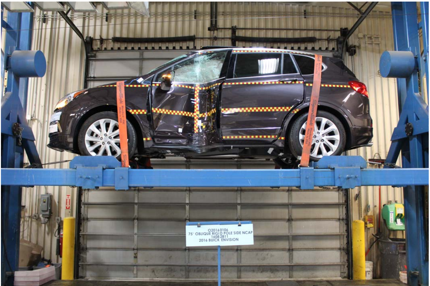
Photo No. 067 - FMVSS No. 301 Static Rollover 360 Degrees
