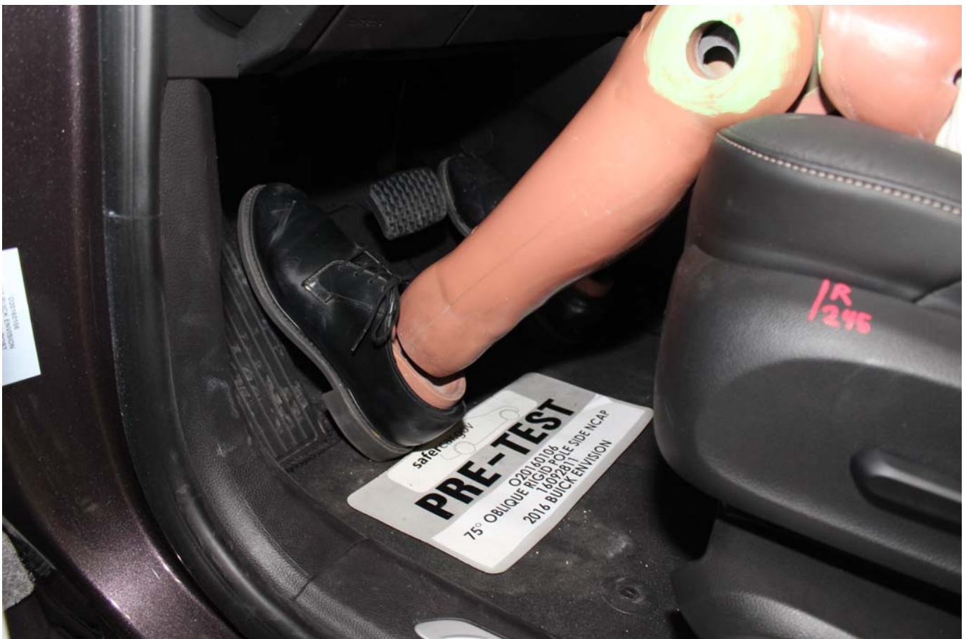
Photo No. 032 - Pre-Test Placement of Dummy Feet
