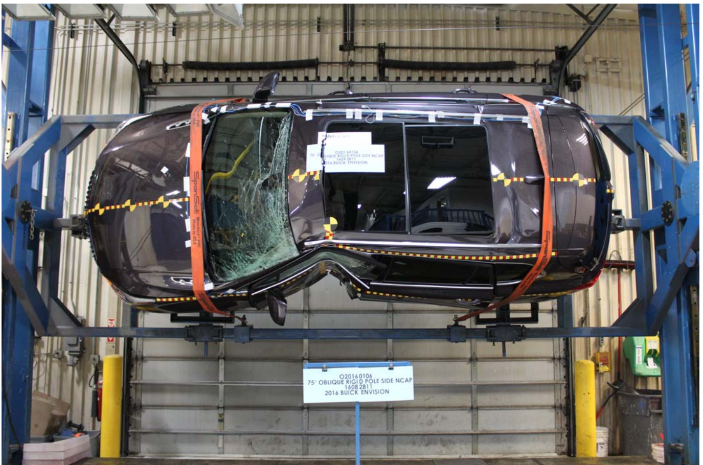
Photo No. 066 - FMVSS No. 301 Static Rollover 270 Degrees
