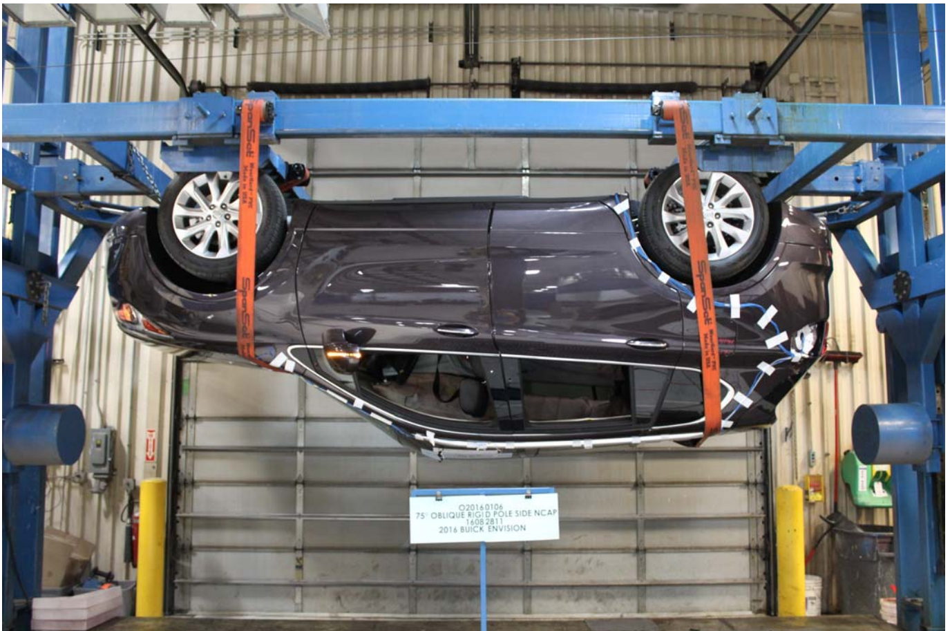
Photo No. 065 - FMVSS No. 301 Static Rollover 180 Degrees
