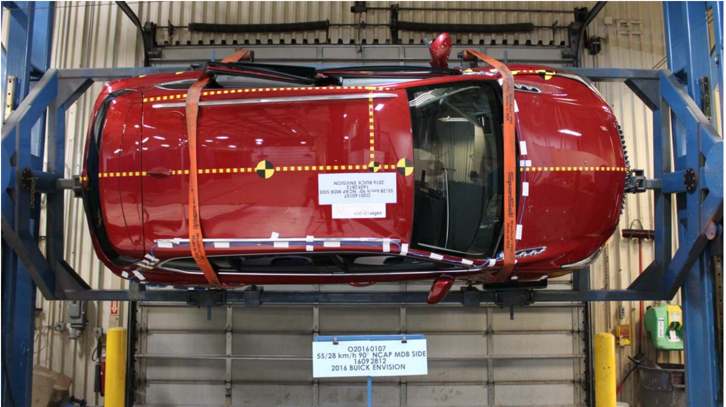
Photo No. 097 - FMVSS No. 301 Static Rollover 90 Degrees
