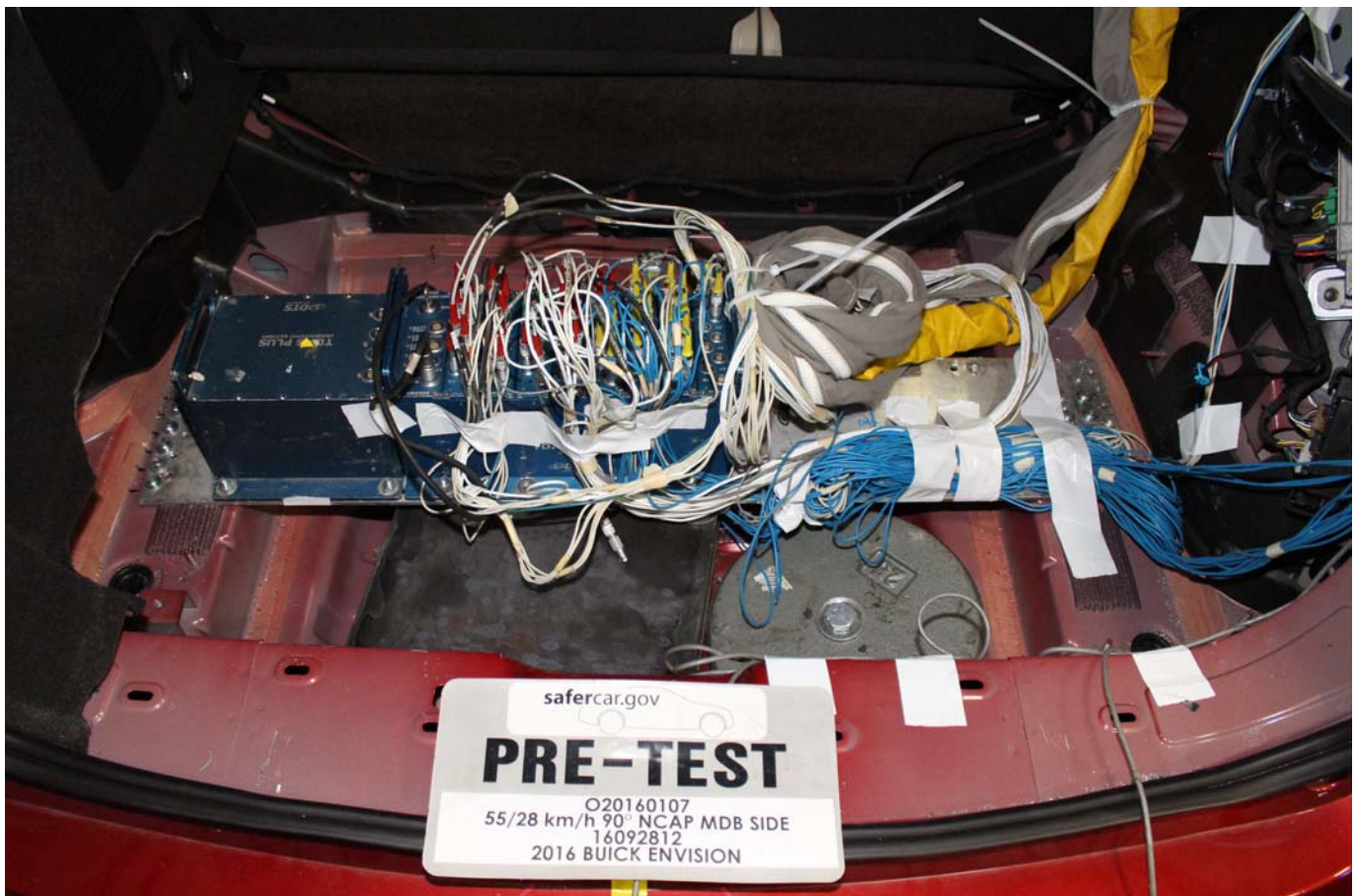
Photo No. 094 - Pre-Test Ballast View
