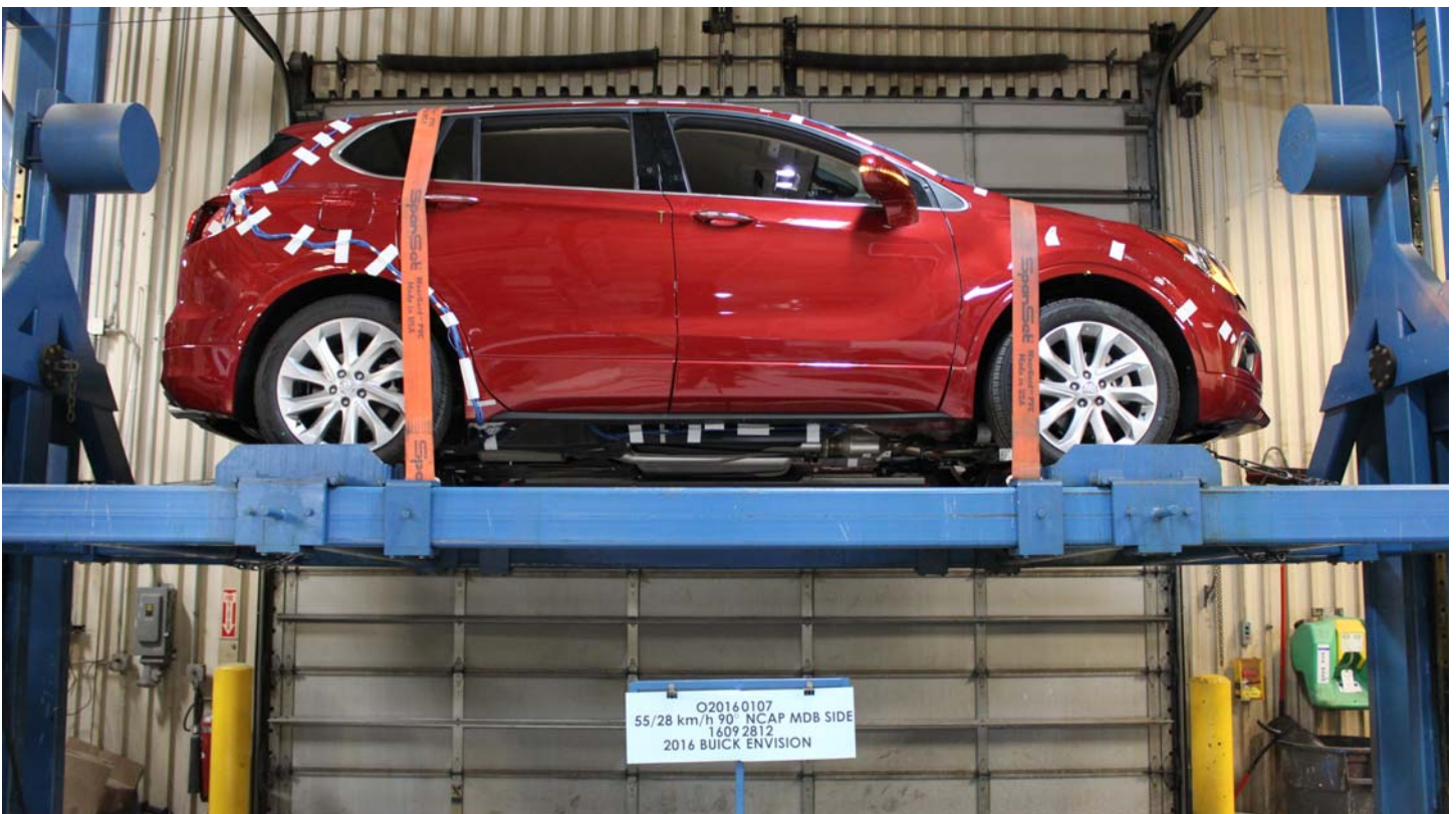
Photo No. 100 - FMVSS No. 301 Static Rollover 360 Degrees
