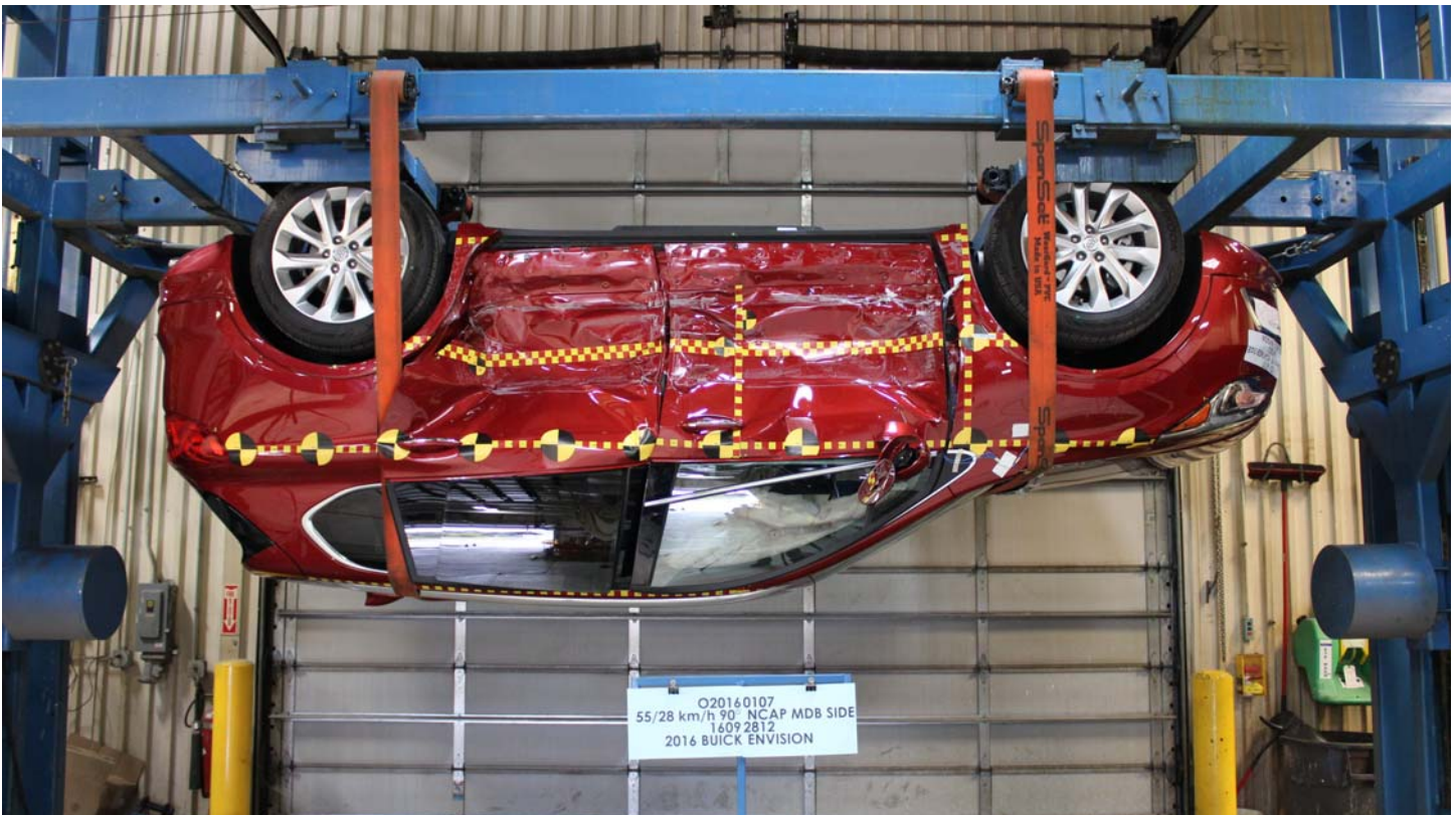
Photo No. 098 - FMVSS No. 301 Static Rollover 180 Degrees
