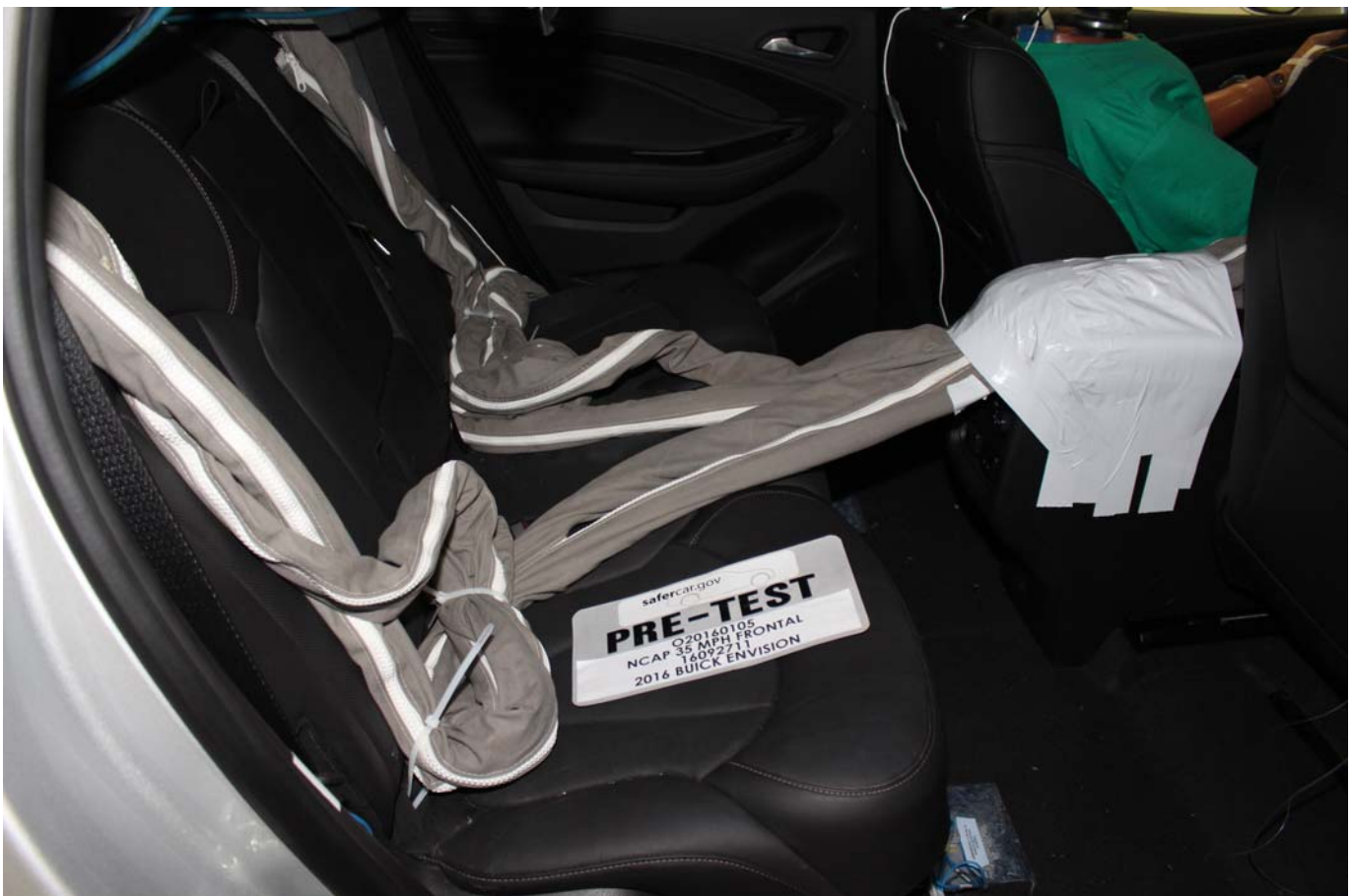
Photo No. 028 - Pre-Test Dummy Cable Routing
