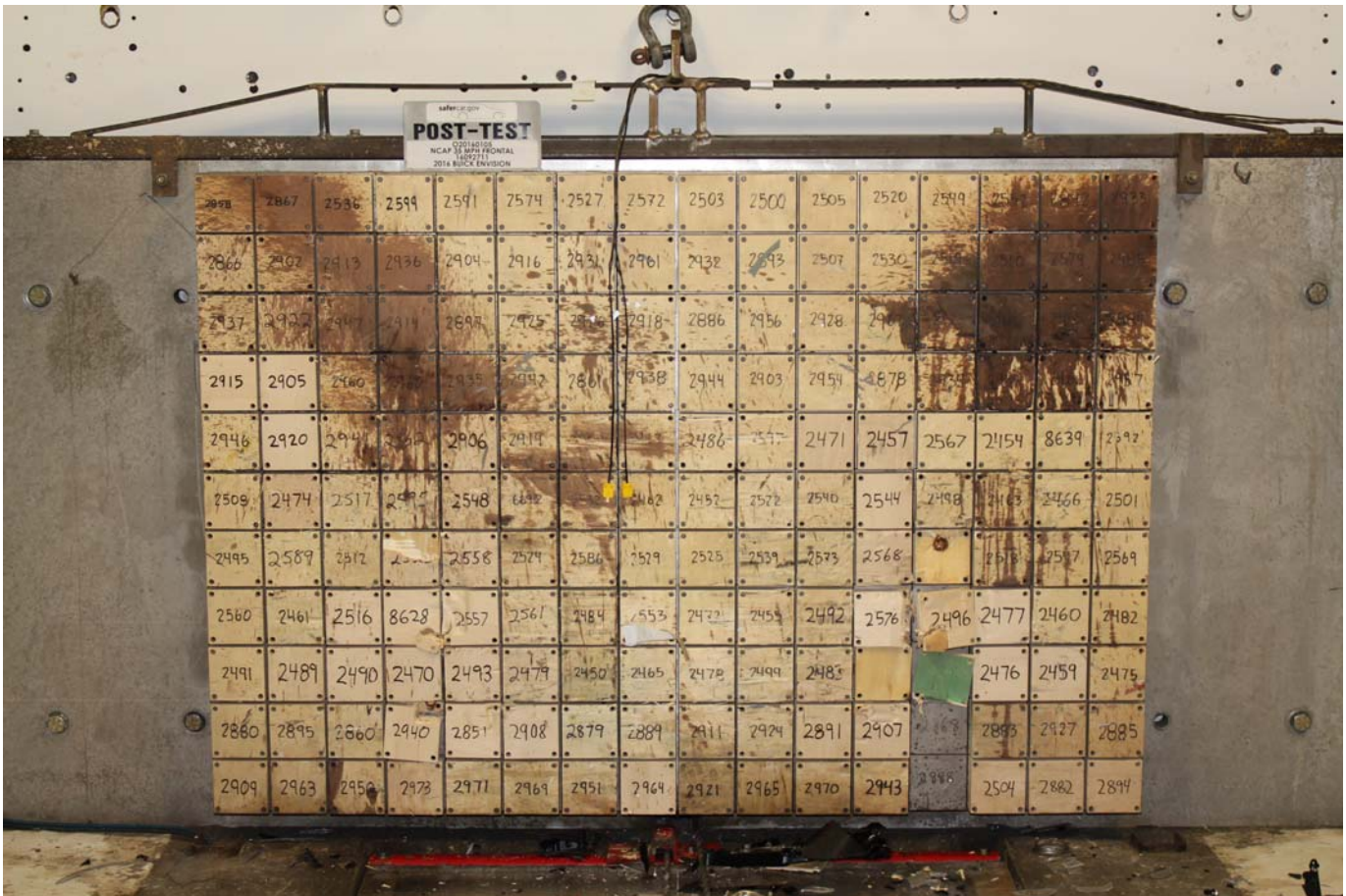
Photo No. 003 - Post-Test Load Cell Wall
