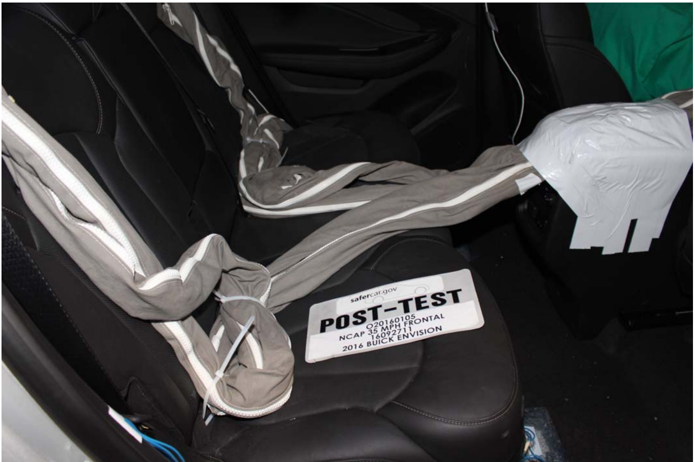
Photo No. 029 - Post-Test Dummy Cable Routing
