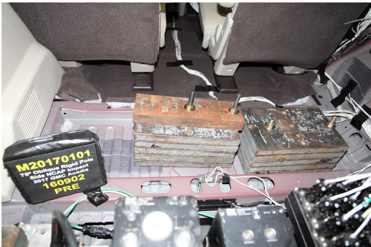
No. 061a Pre-Test Ballast View
