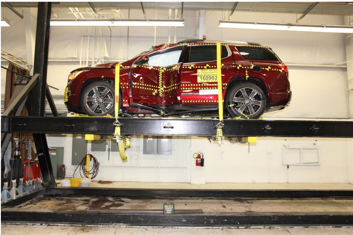
No. 067 FMVSS No. 301 Static Rollover 360 Degrees
