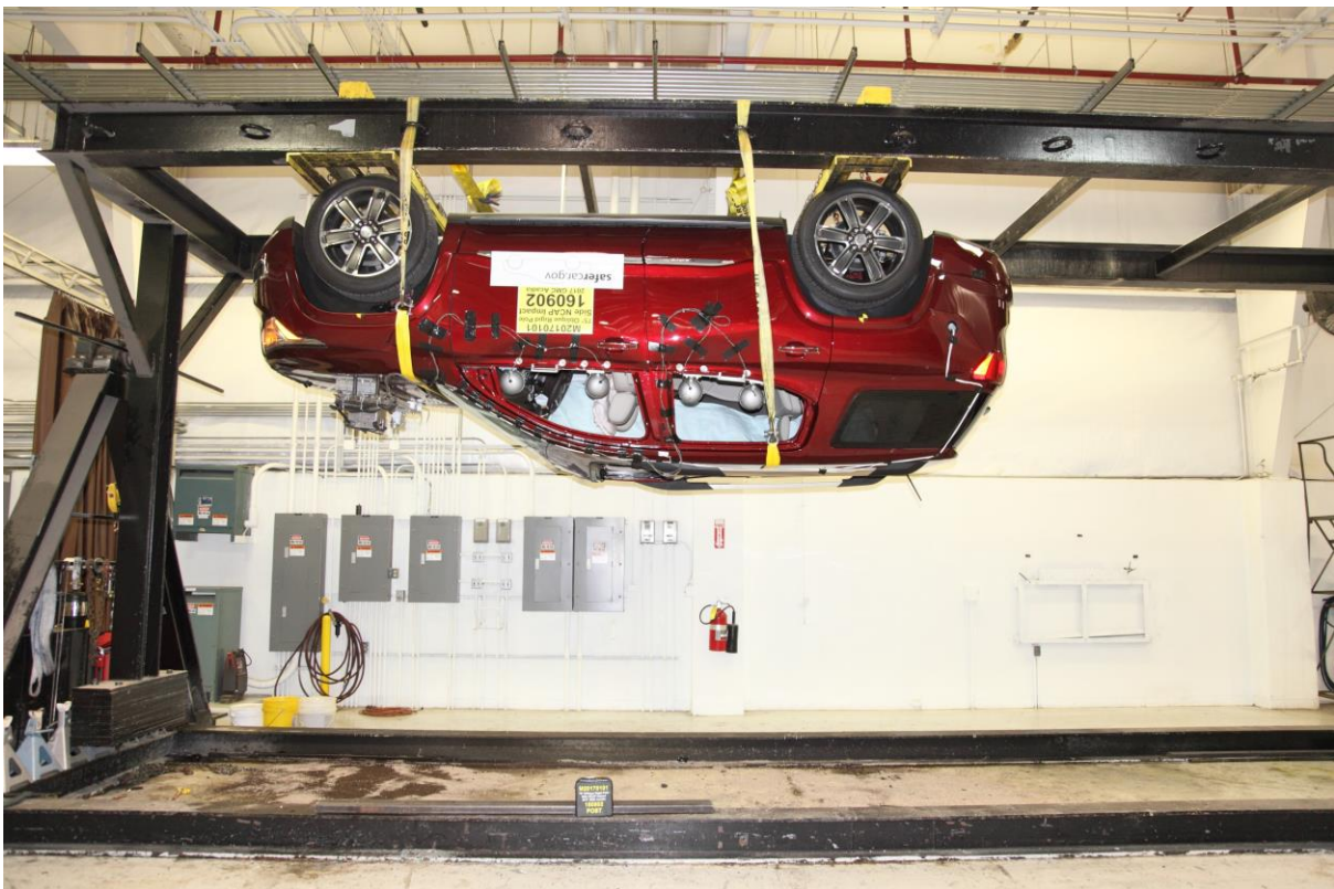
No. 065 FMVSS No. 301 Static Rollover 180 Degrees
