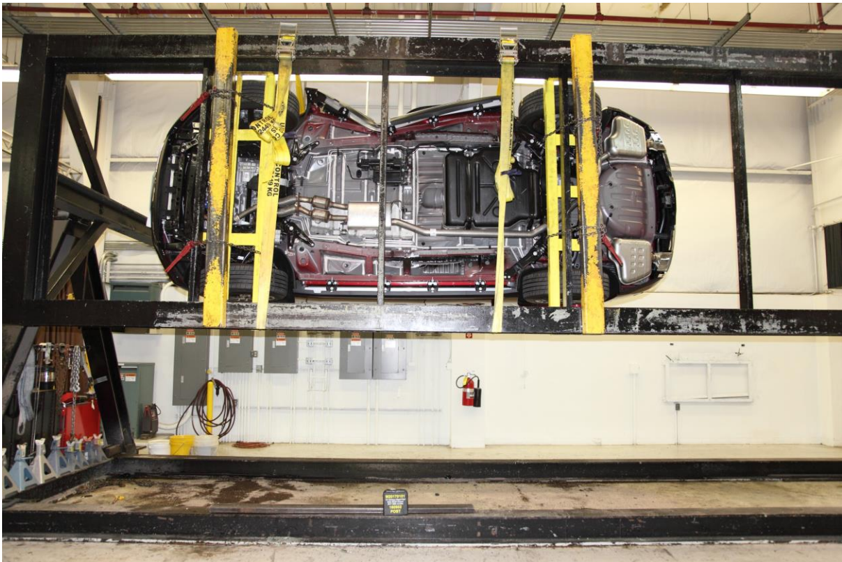
No. 066 FMVSS No. 301 Static Rollover 270 Degrees
