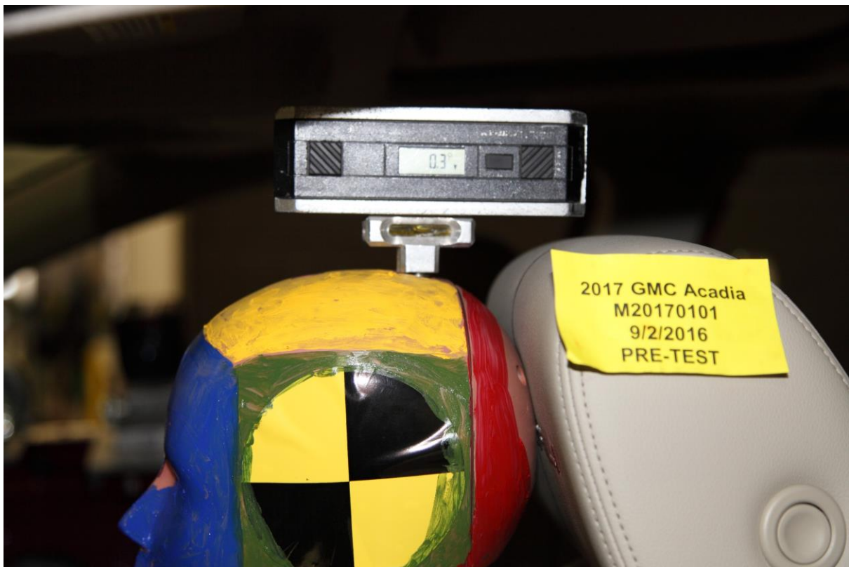
No. 031 Pre-Test Left Side View of Dummy Head Showing Dummy Head is Level
