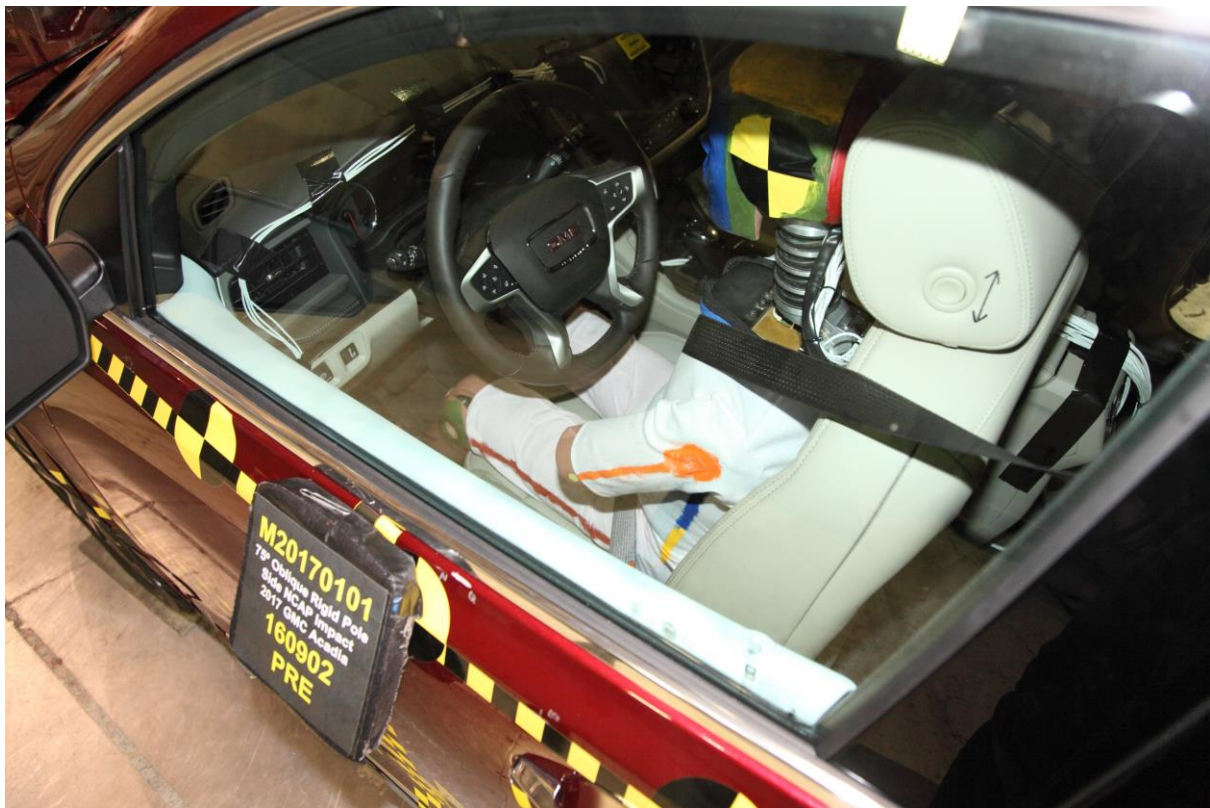
No. 040 Pre-Test Dummy and Door Clearance View
