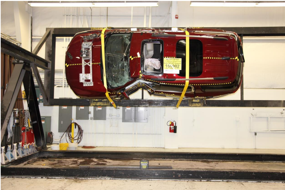
No. 064 FMVSS No. 301 Static Rollover 90 Degrees
