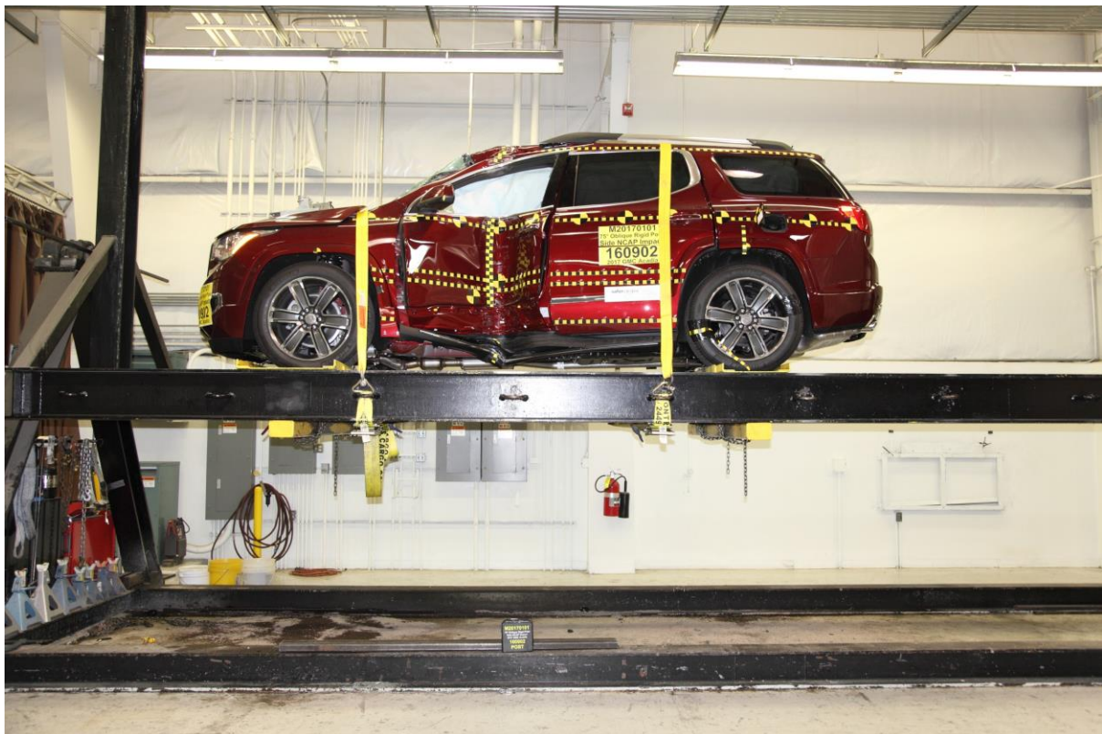
No. 063 FMVSS No. 301 Static Rollover 0 Degrees
