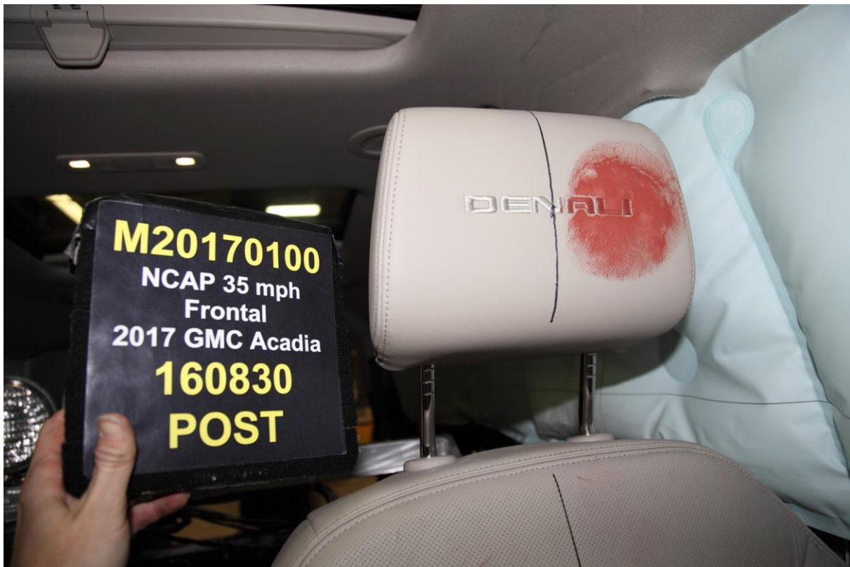
048 Post-Test Driver Dummy Contact With Headrest
