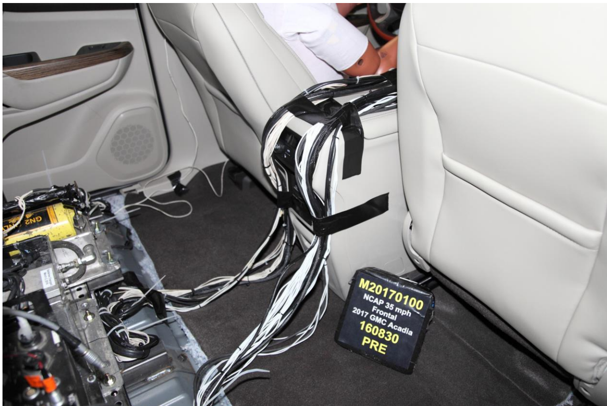
028 Pre-Test Dummy Cable Routing
