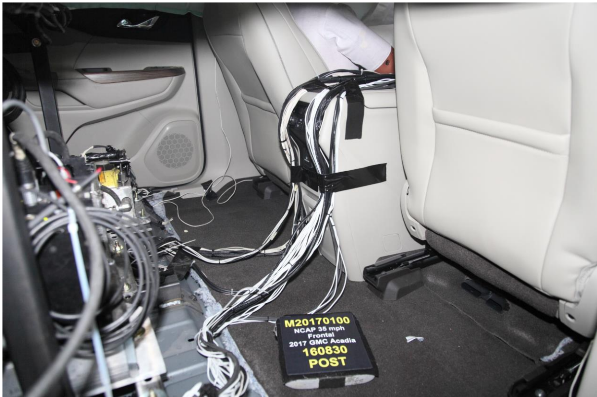
029 Post-Test Dummy Cable Routing
