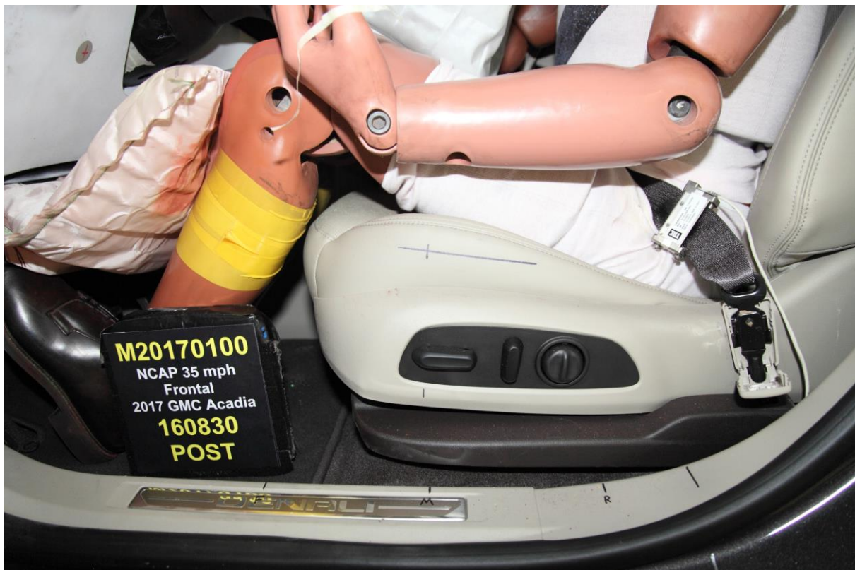
037 Post-Test Driver's Seat Fore-Aft Markings
