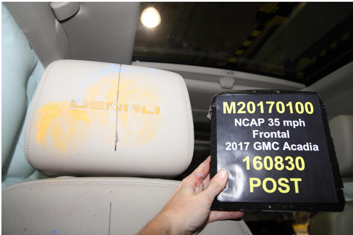
069 Post Test Passenger Dummy Contact With Headrest
