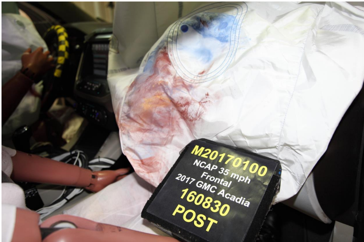
068 Post-Test Passenger Dummy Contact With Airbag
