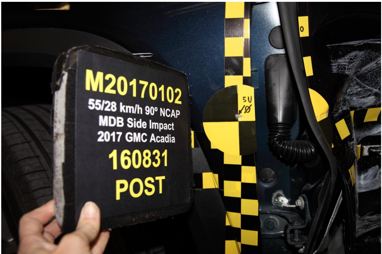
020 Post-Test Close-Up View of Impact Point Target
