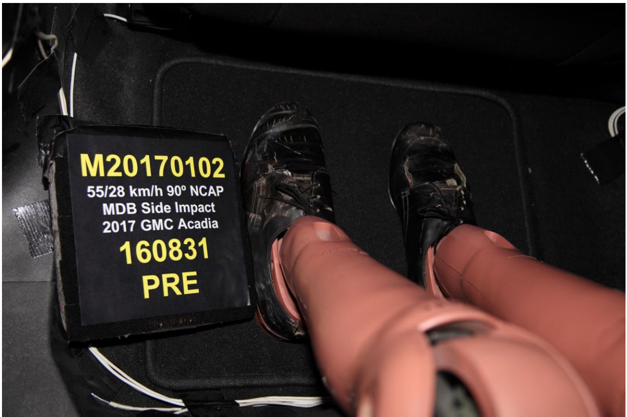
064 Pre-Test Placement of Rear Passenger Dummy Feet
