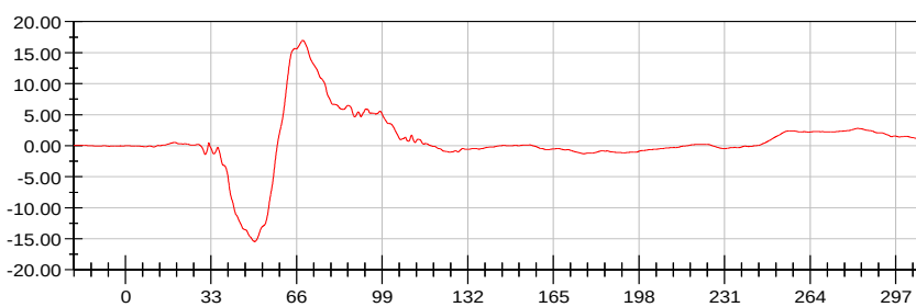
Passenger Lower Spine T12 Acceleration (Z) (g) vs. Time [ms]
