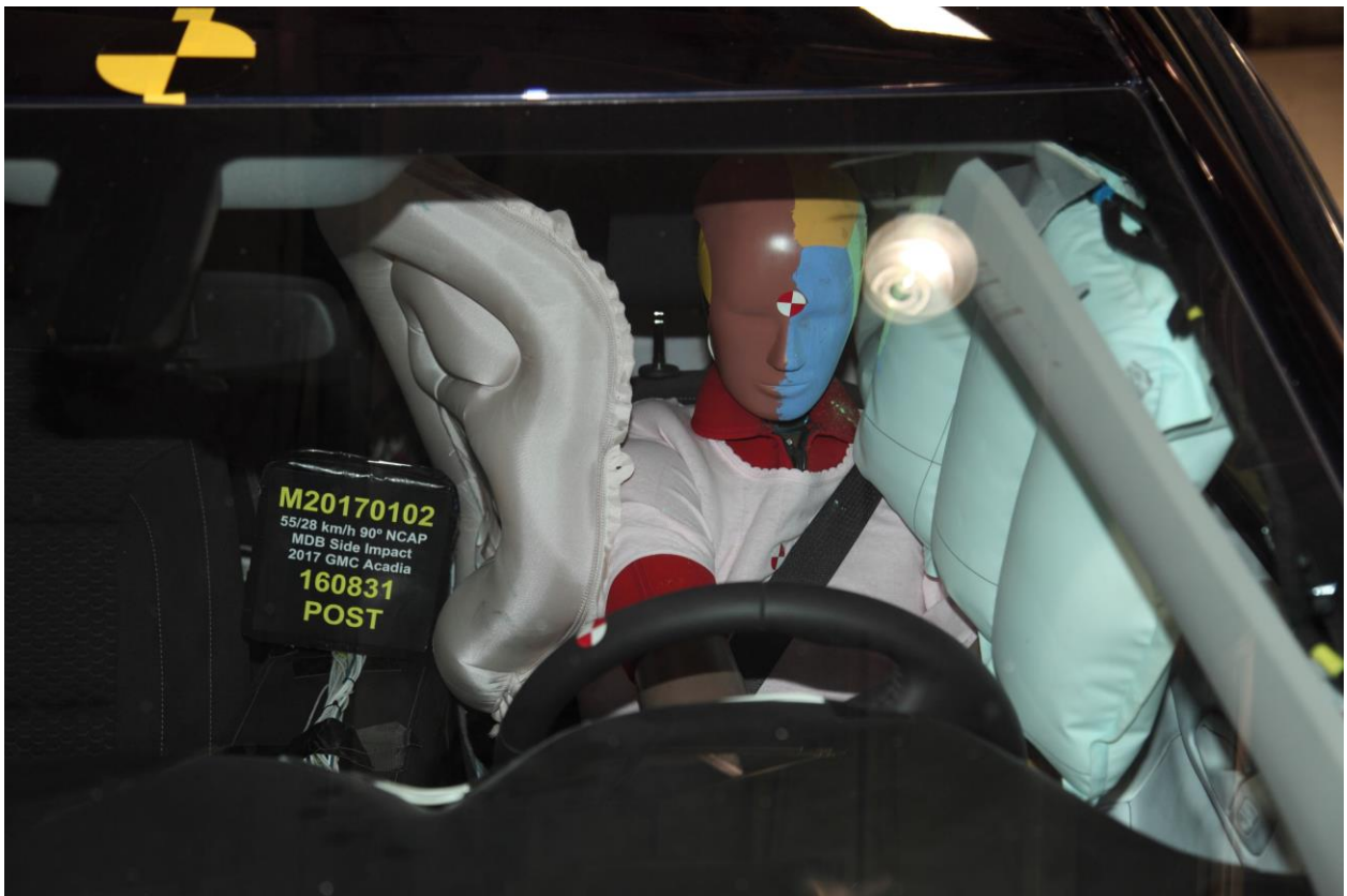
026 Post-Test Front Close-Up View of Driver Dummy
