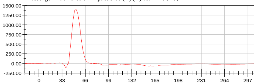
Passenger Acetabulum Force on Impact Side (Y) (N) vs. Time [ms]
