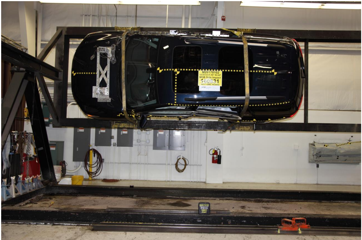
097 FMVSS No. 301 Static Rollover 90 Degrees
