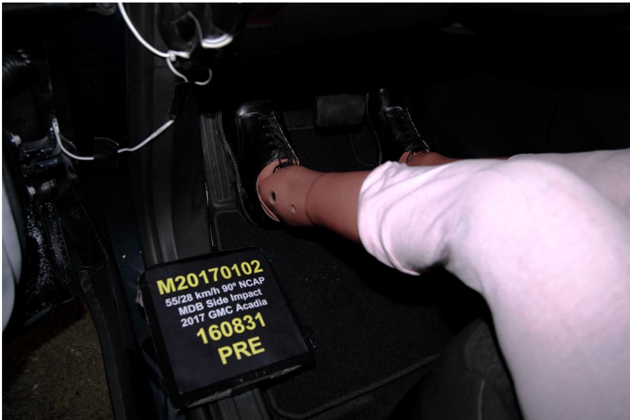
034 Pre-Test Placement of Driver Dummy Feet
