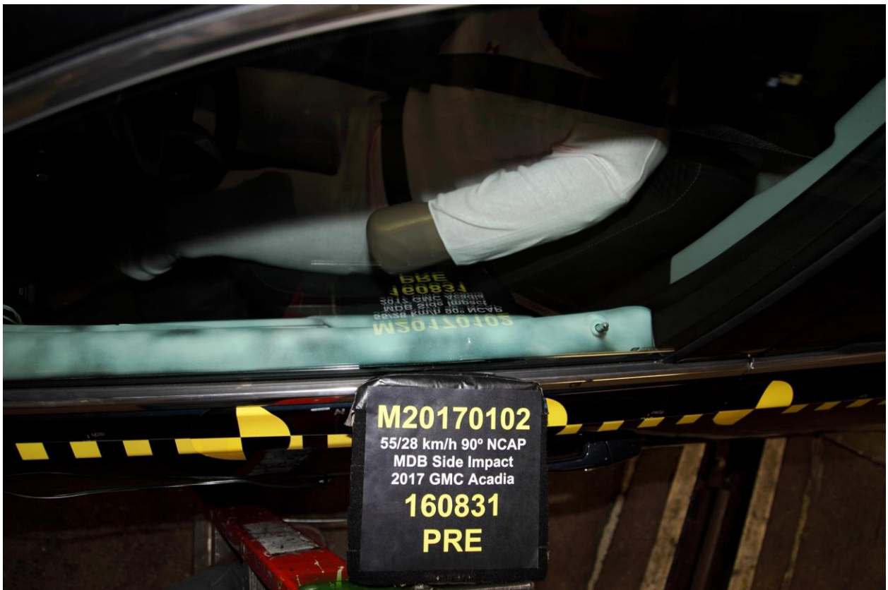
042 Pre-Test Driver Dummy and Door Clearance View
