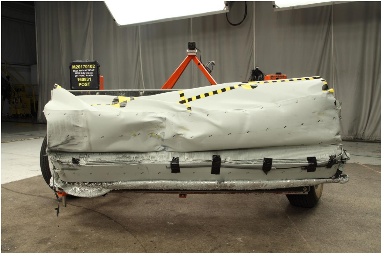
085 Post-Test Front View of MDB Impactor Face
