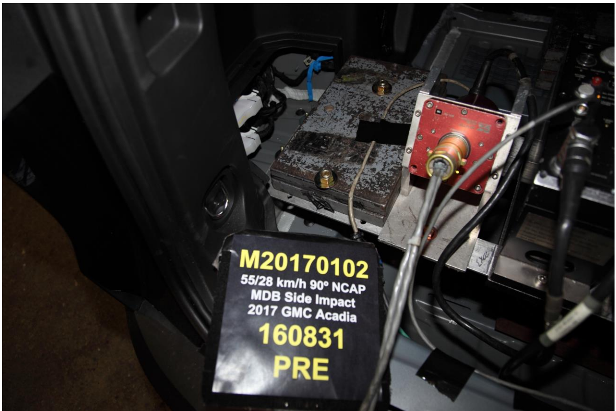
094b Pre-Test Ballast View 3
