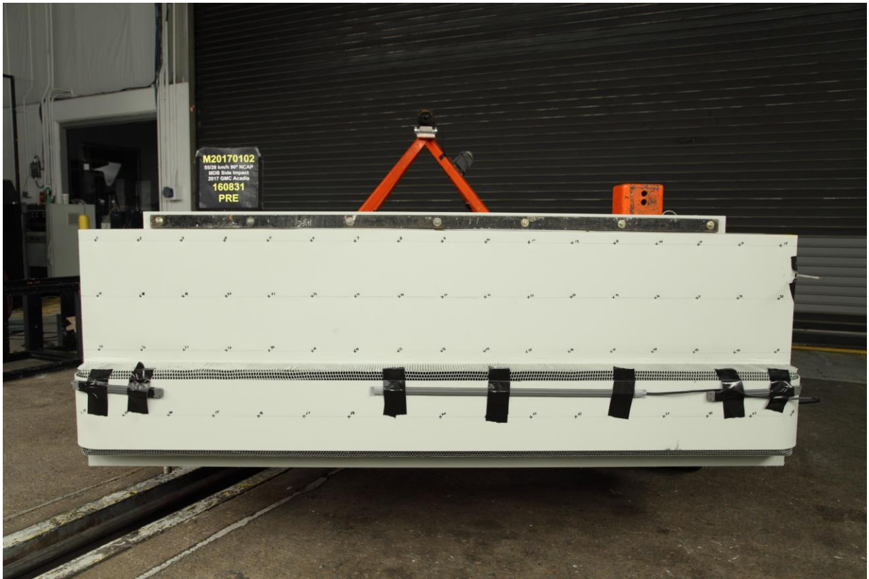
084 Pre-Test Front View of MDB Impactor Face
