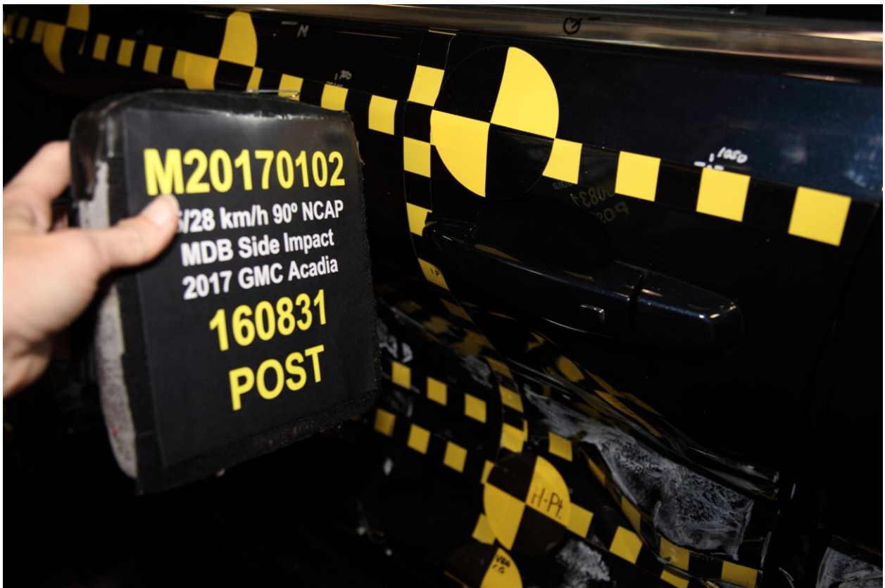
022 Post-Test Left Front Door Latch Close-Up
