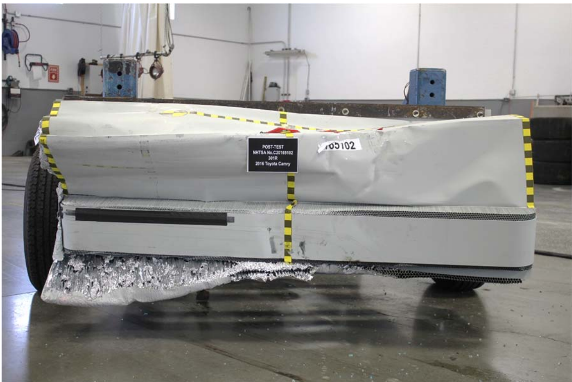
Figure A-20: Post-Test MDB Front View
