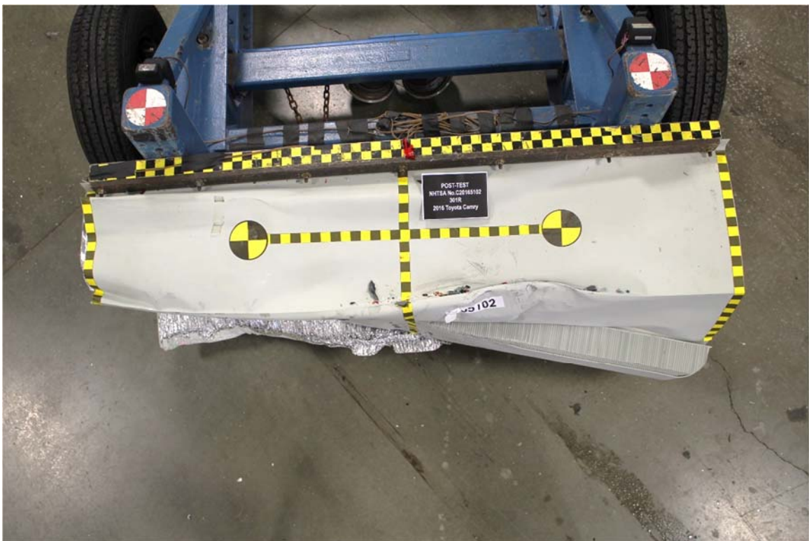
Figure A-26: Post-Test MDB Top View
