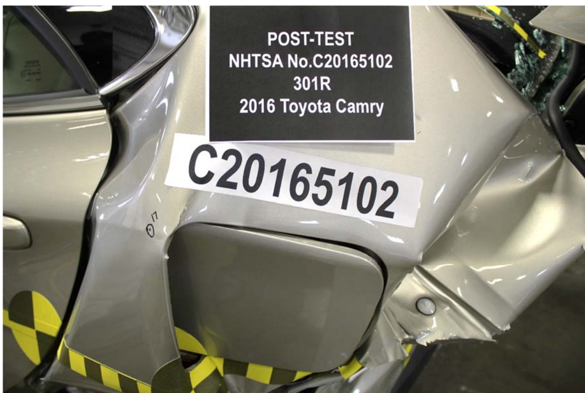
Figure A-36: Post-Test Fuel Filler Cap View
