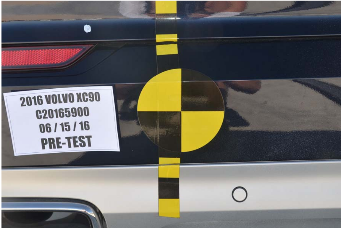
FIGURE 21. Pre-Test Close-Up View of Impact Point Target
