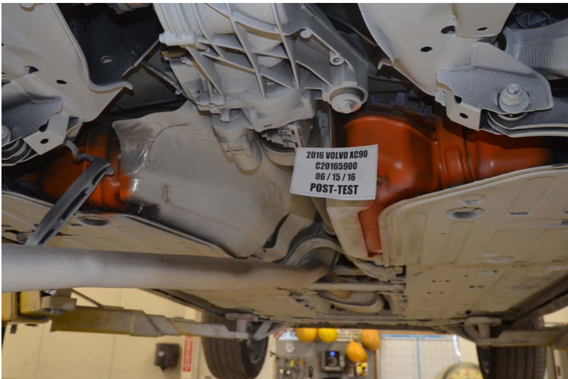
FIGURE 28. Post-Test Underbody View of Fuel Tank
