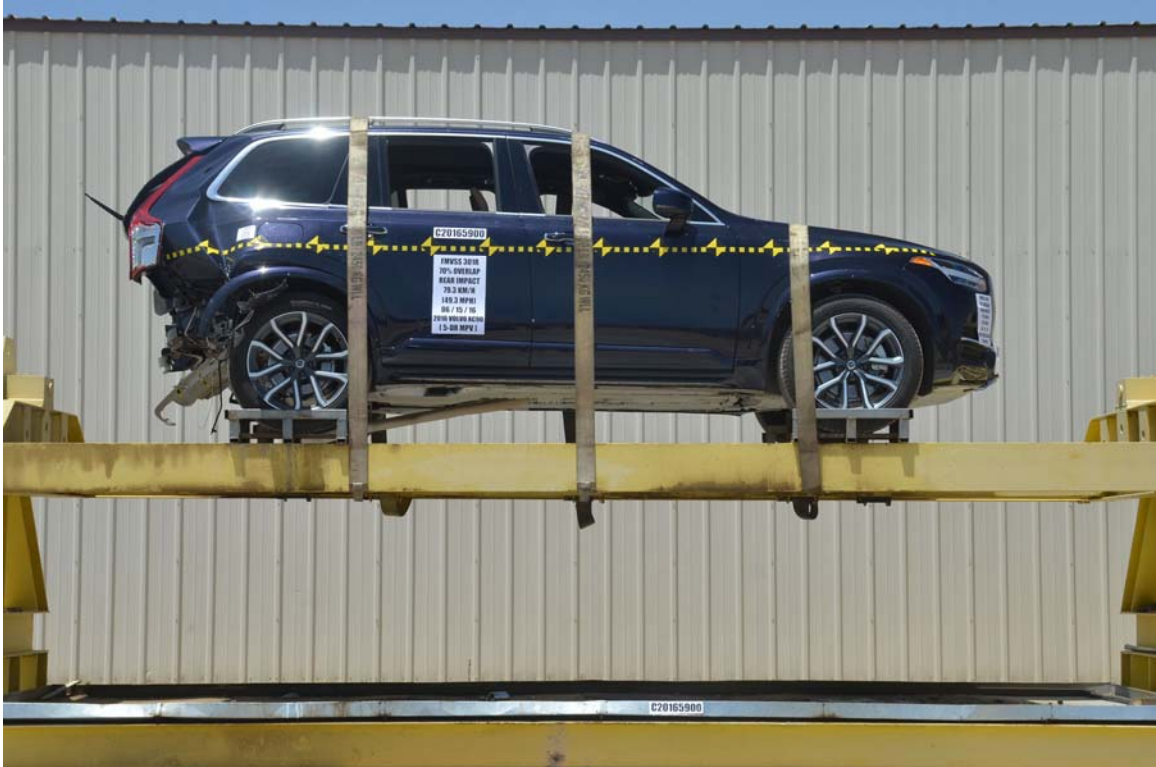
FIGURE 29. Test Vehicle at 0° on FMVSS 301 Static Rollover Device
