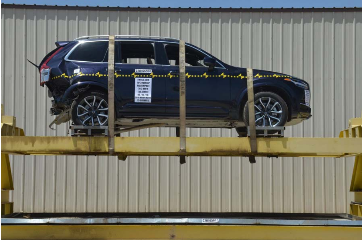
FIGURE 33. Test Vehicle at 360° on FMVSS 301 Static Rollover Device
