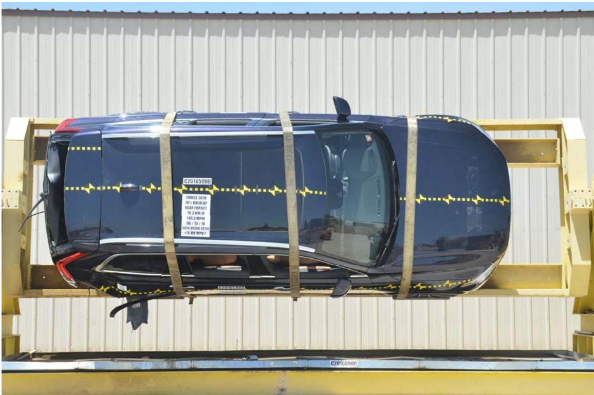
FIGURE 30. Test Vehicle at 90° on FMVSS 301 Static Rollover Device
