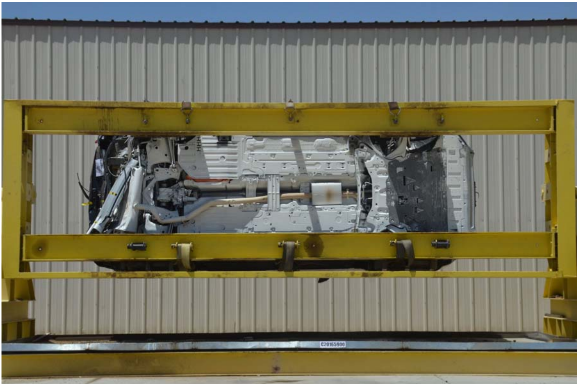
Test Vehicle at 270° on FMVSS 301 Static Rollover Device
