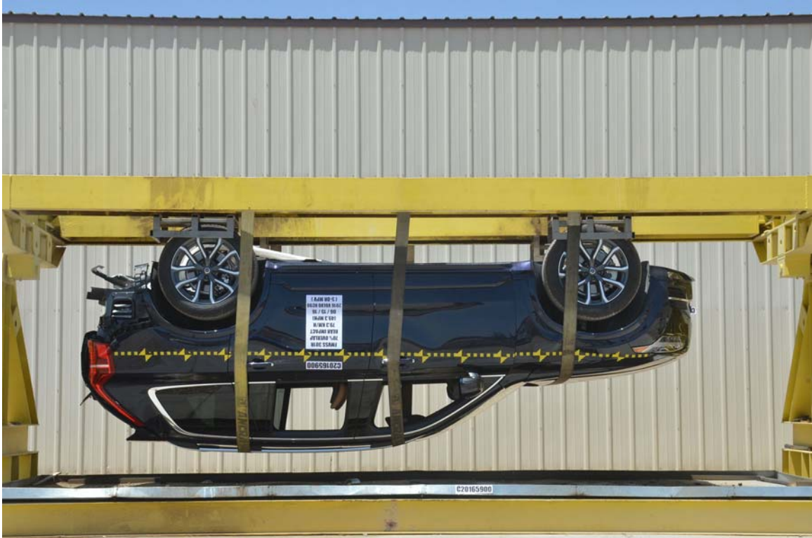
FIGURE 31. Test Vehicle at 180° on FMVSS 301 Static Rollover Device
