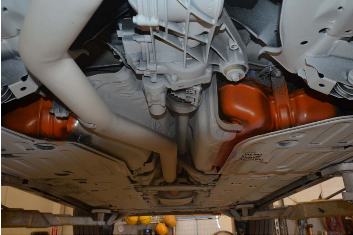
FIGURE 27. Pre-Test Underbody View of Fuel Tank
