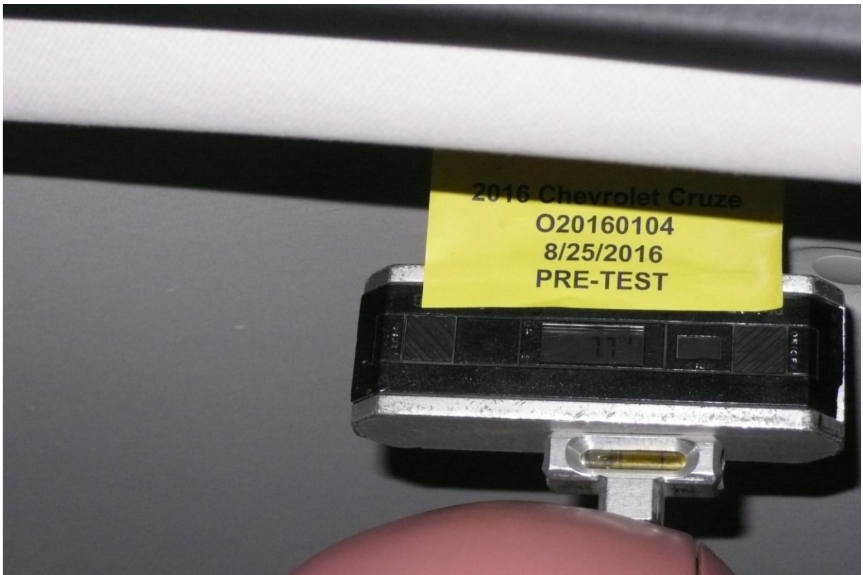
063 Pre-Test View of Rear Passenger Dummy Head Showing Dummy's Head is Level
