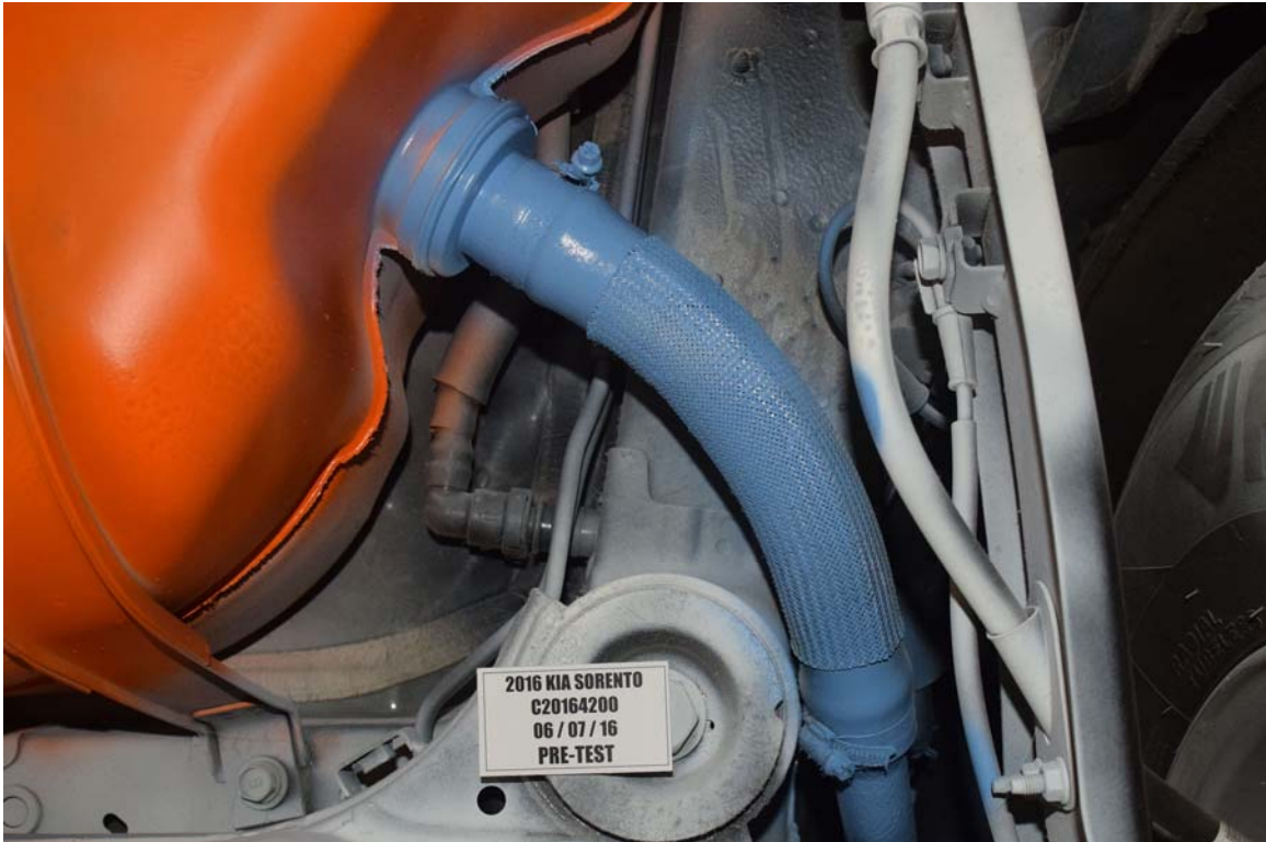
FIGURE 29. Pre-Test Underbody View of Fuel Lines
