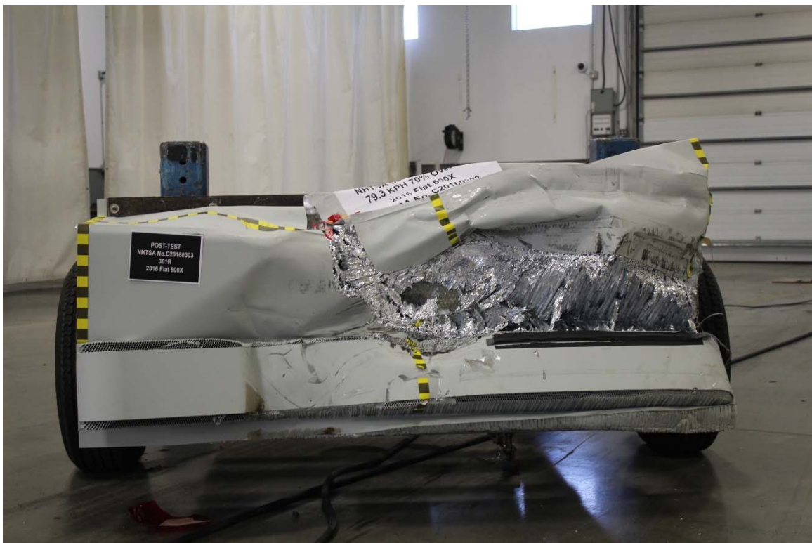
Figure A-20: Post-Test MDB Front View
