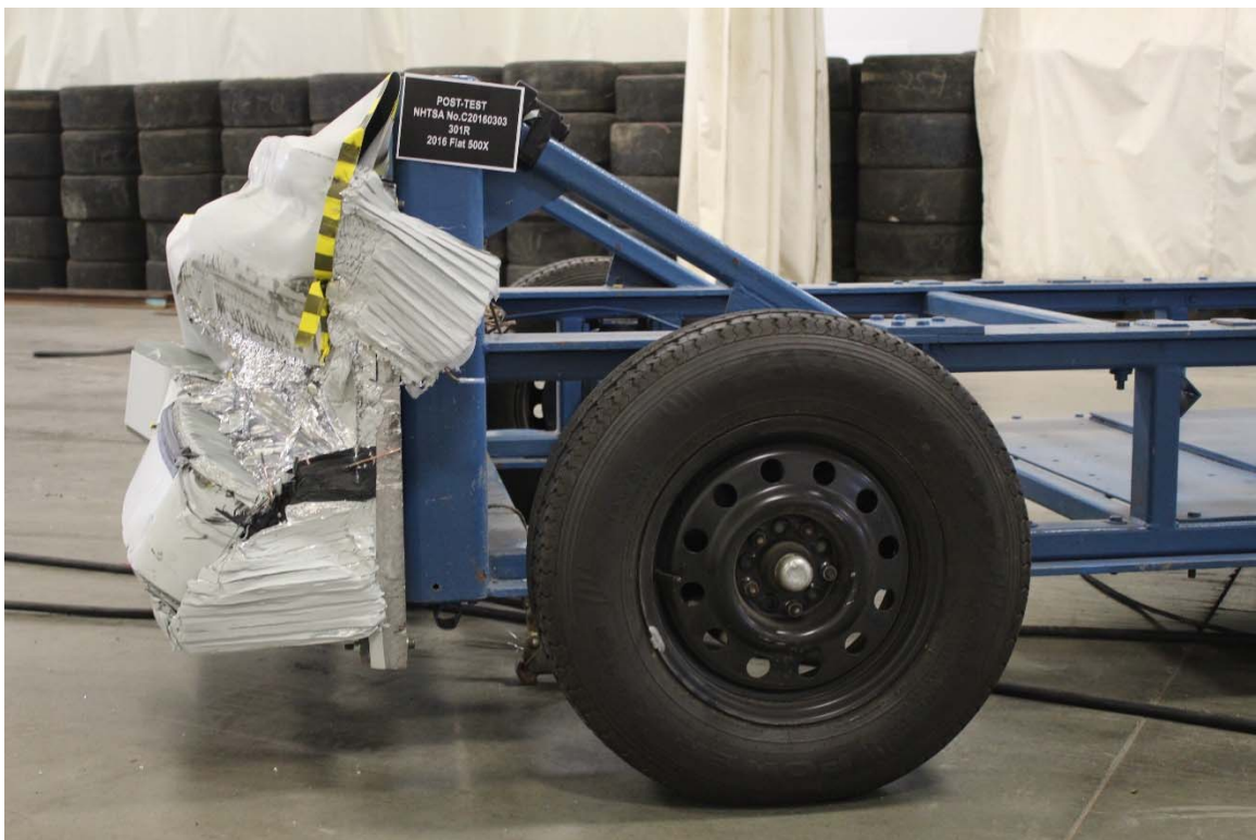
Figure A-22: Post-Test MDB Left Side View
