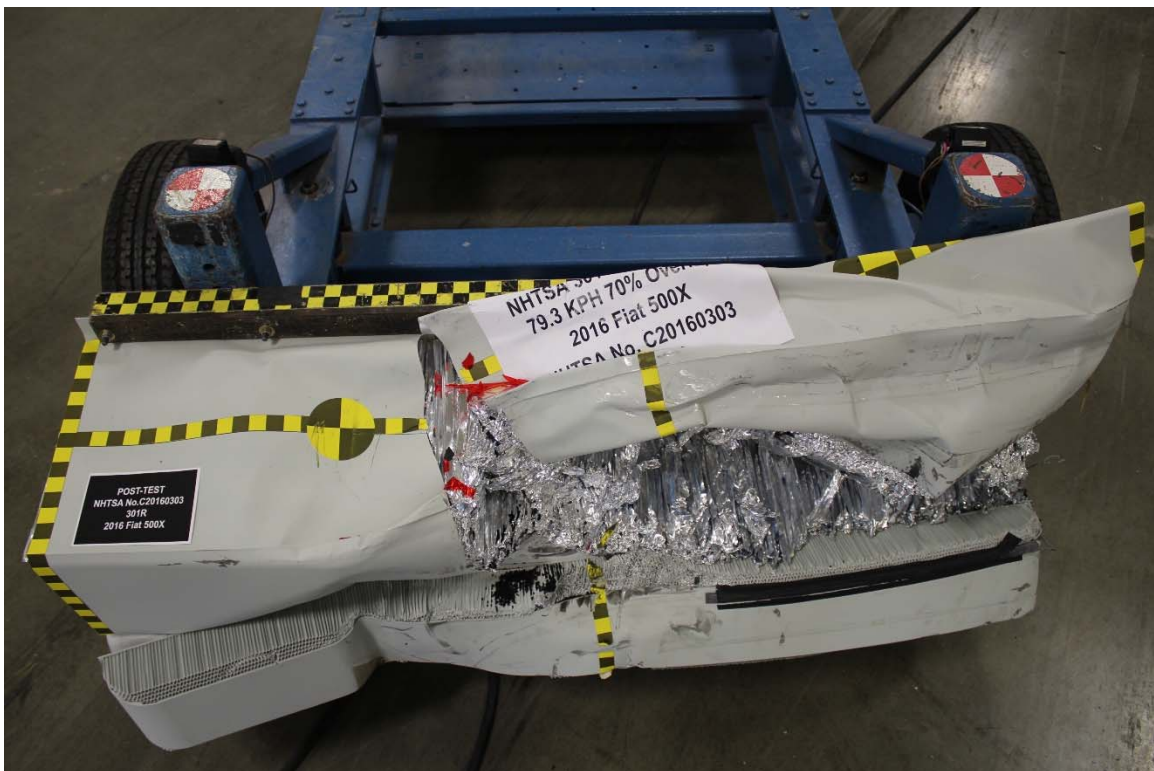
Figure A-26: Post-Test MDB Top View
