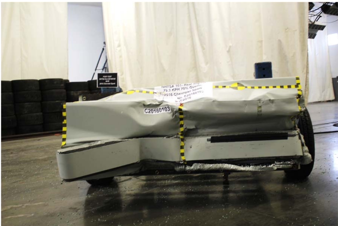
Figure A-20: Post-Test MDB Front View
