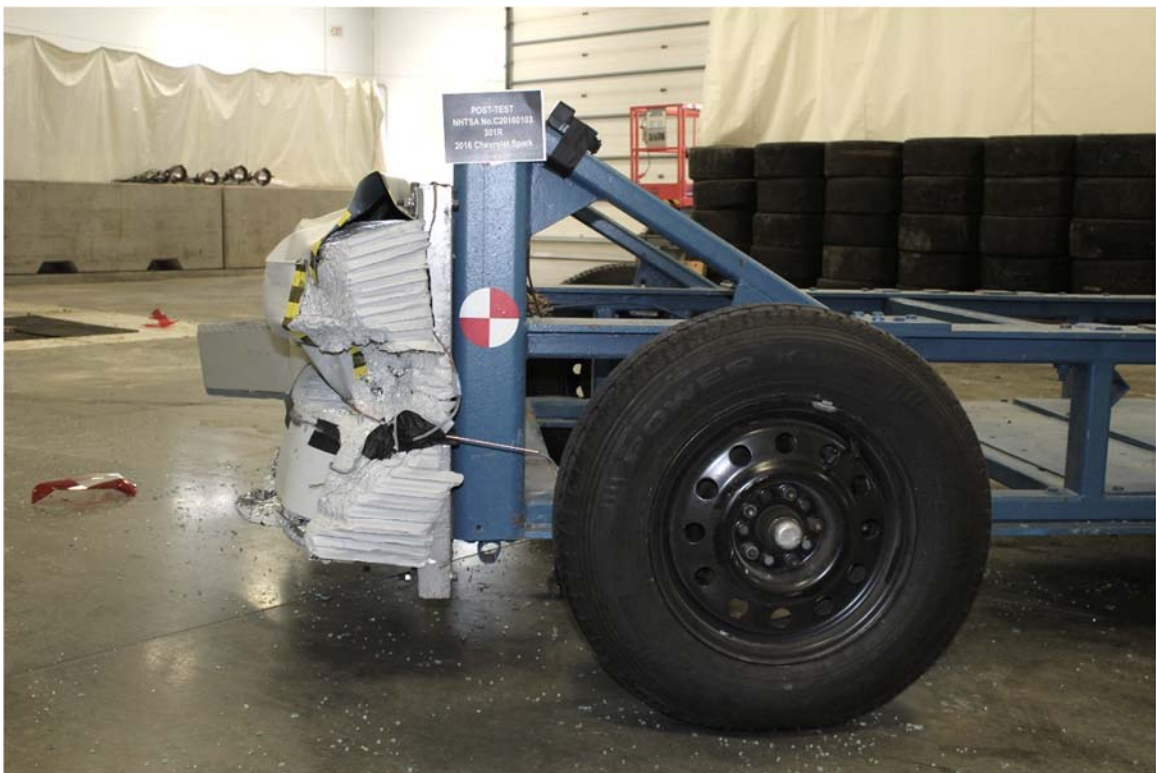
Figure A-22: Post-Test MDB Left Side View
