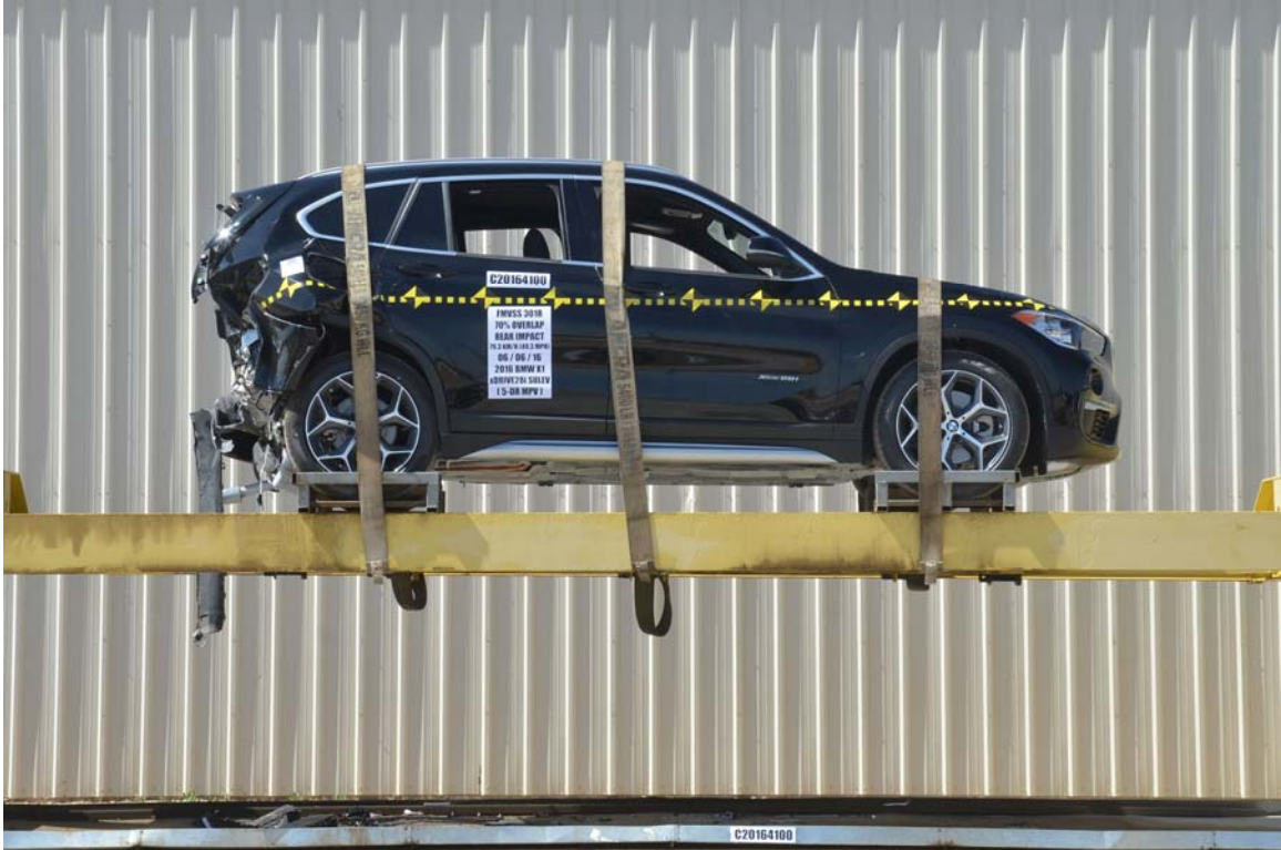
FIGURE 31. Test Vehicle at 0° on FMVSS 301 Static Rollover Device
