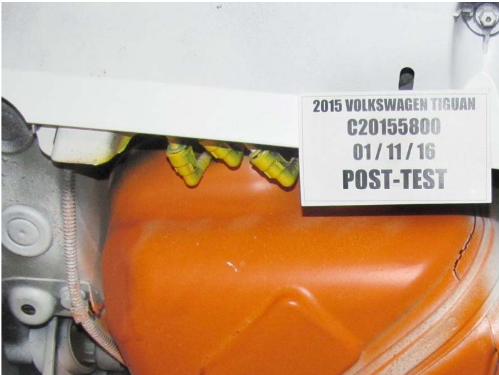
FIGURE 32. Post-Test Underbody View of Fuel Lines
