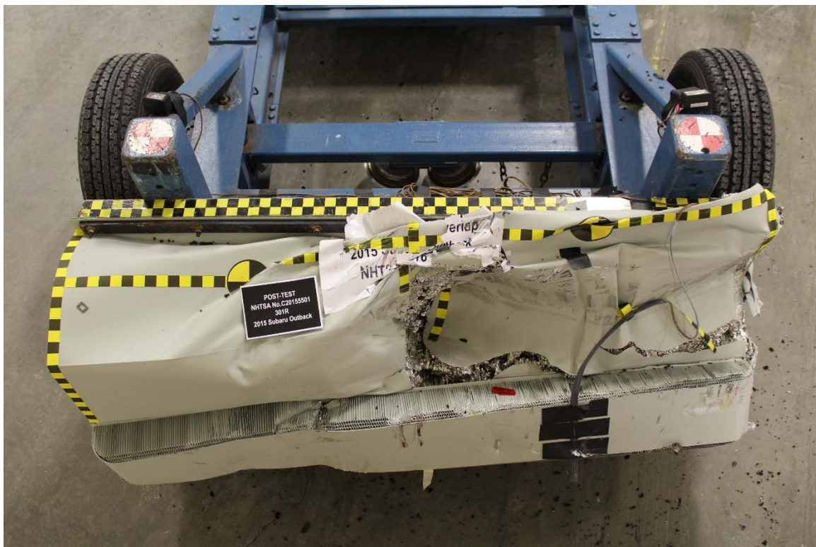
Figure A-26: Post-Test MDB Top View
