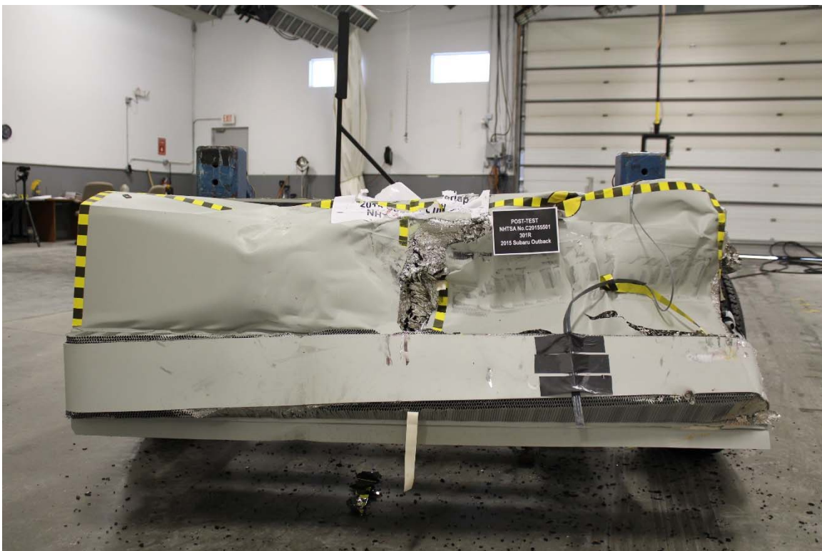
Figure A-20: Post-Test MDB Front View
