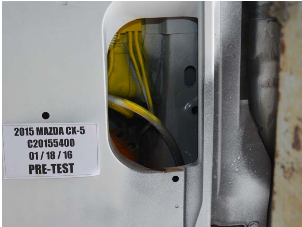
FIGURE 31. Pre-Test Underbody View of Fuel Lines
