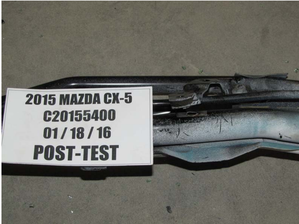
FIGURE 37. Post-Test View of Fuel Filler Neck Damage
