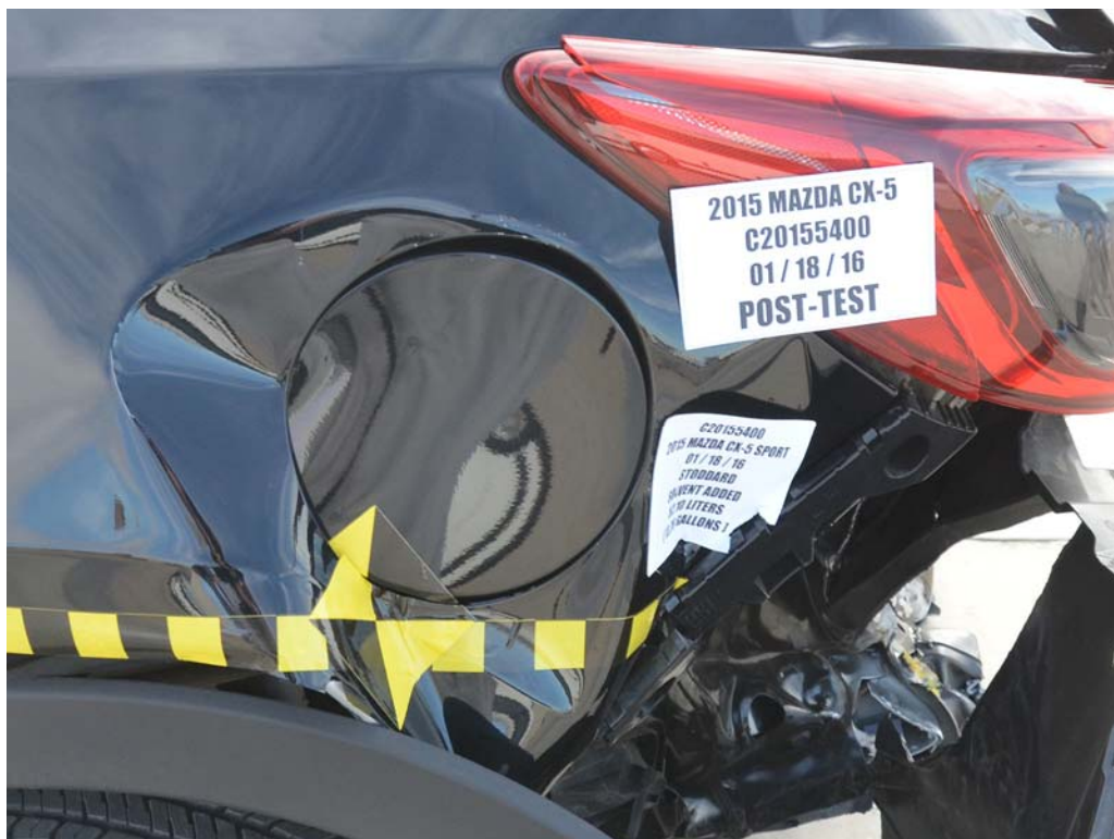
FIGURE 24. Post-Test View of Fuel Filler Cap
