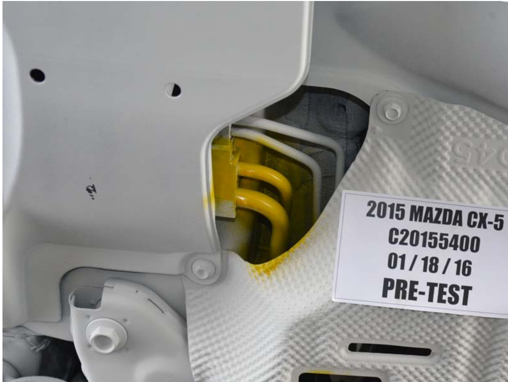
FIGURE 29. Pre-Test Underbody View of Fuel Lines
