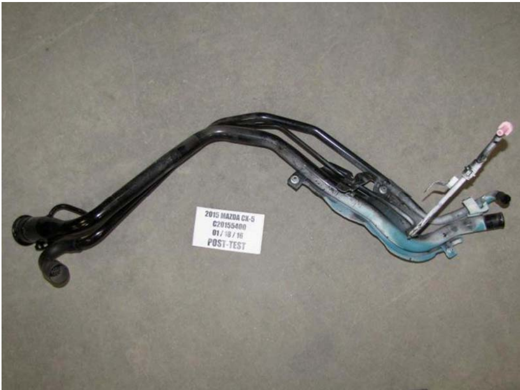
FIGURE 36. Post-Test View of Fuel Filler Neck Damage
