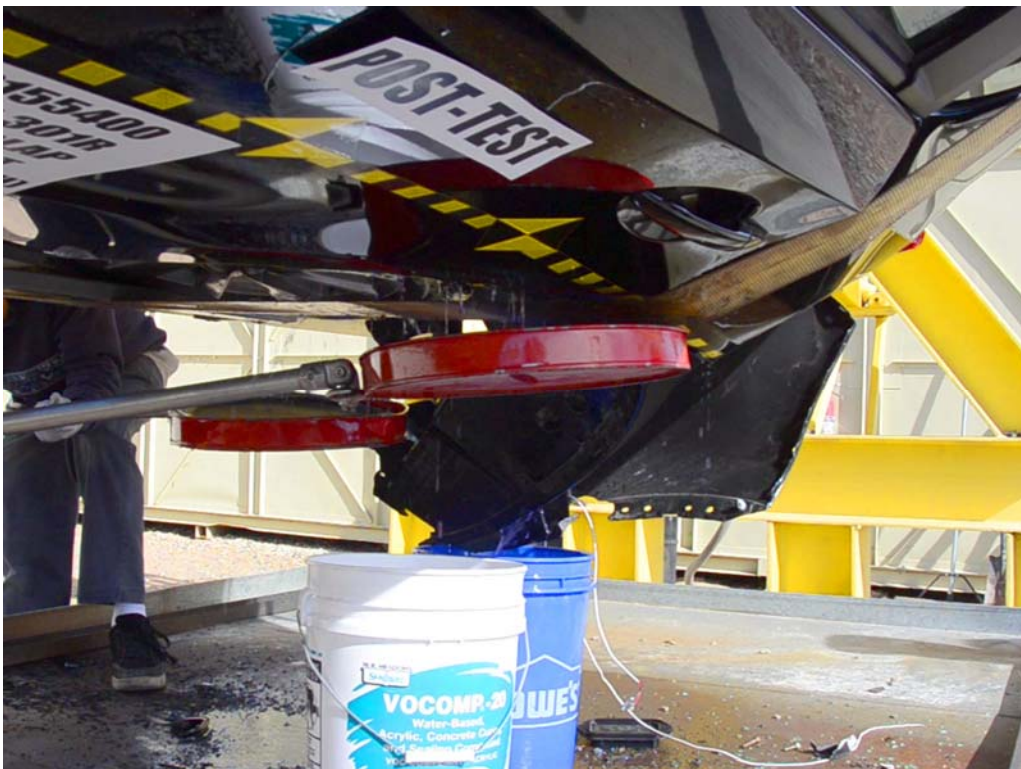
FIGURE 34. Solvent Spillage at 90° on FMVSS 301 Static Rollover Device
