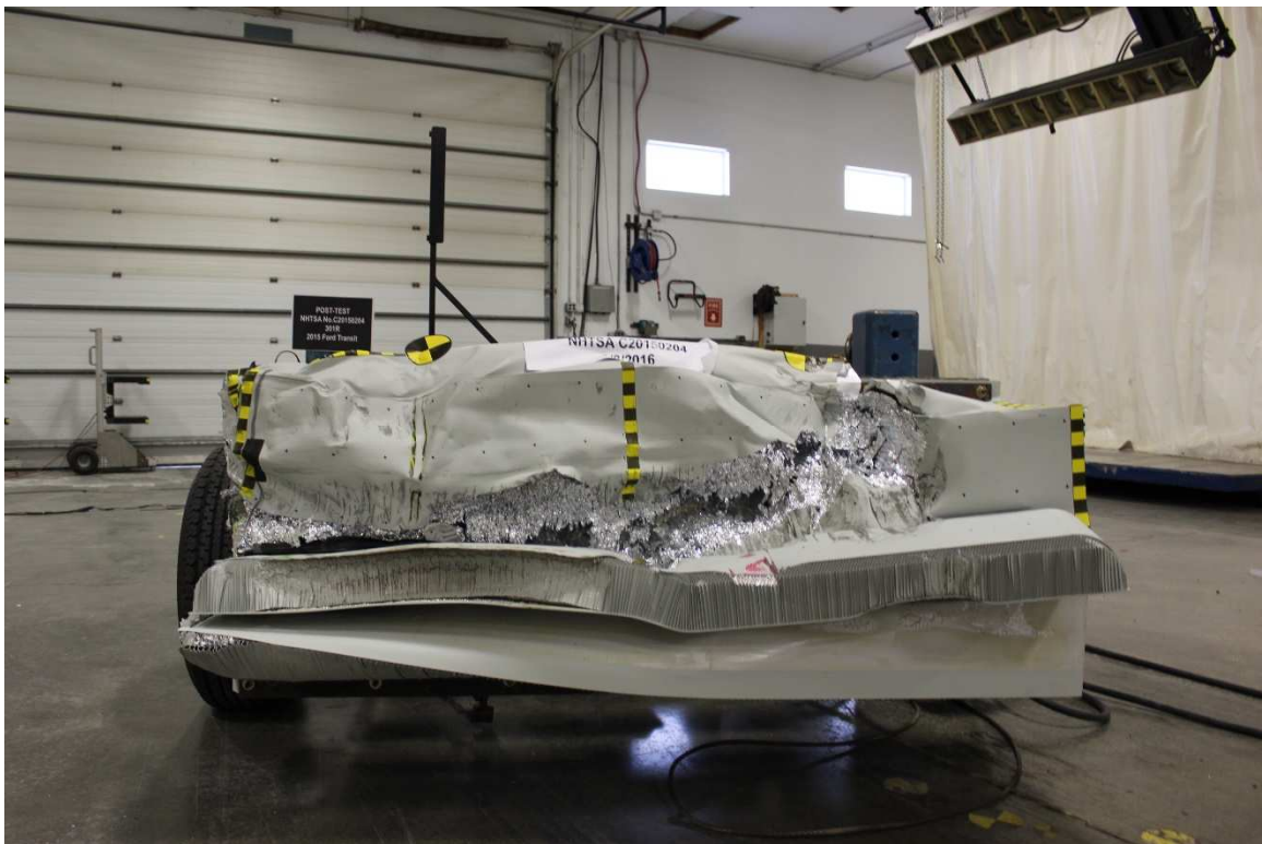
Figure A-20: Post-Test MDB Front View
