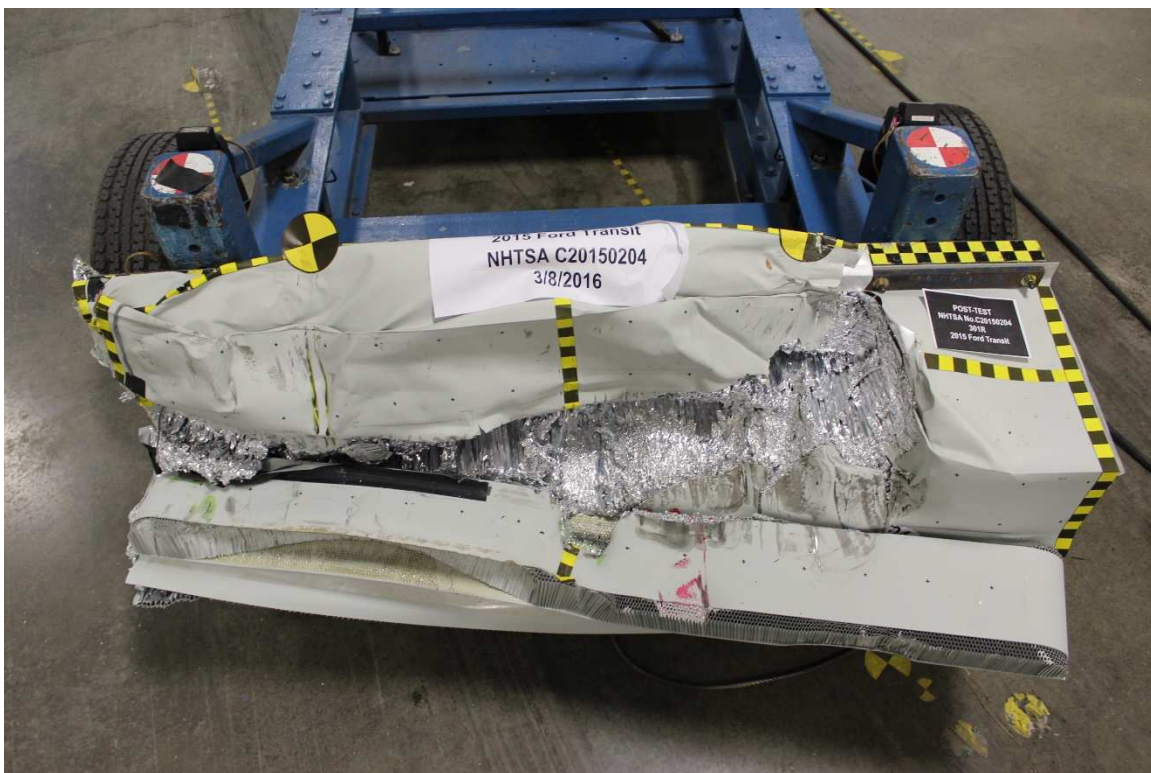
Figure A-26: Post-Test MDB Top View
