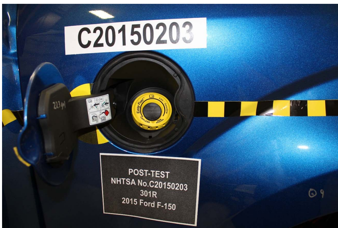
Figure A-36: Post-Test Fuel Filler Cap View
