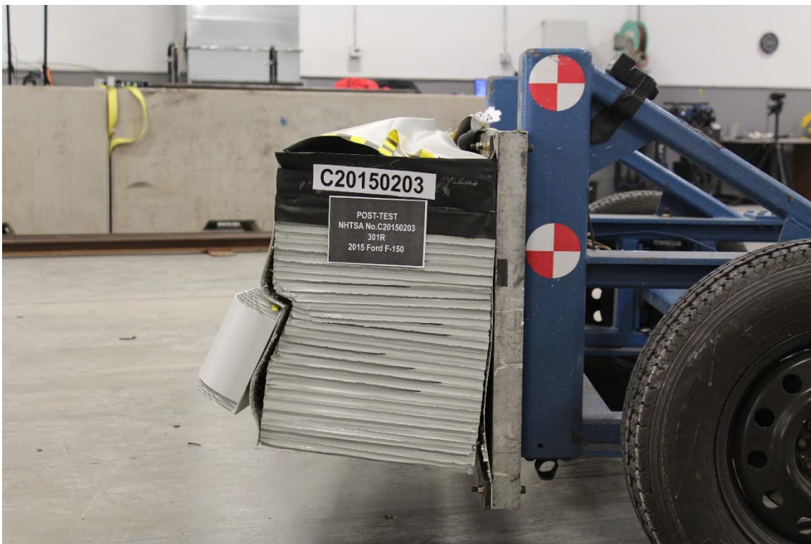
Figure A-22: Post-Test MDB Left Side View
