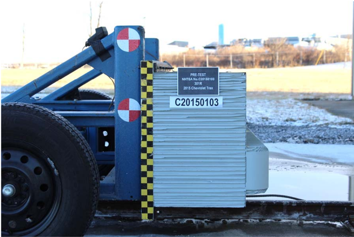
Figure A-23: Pre-Test MDB Right Side View
