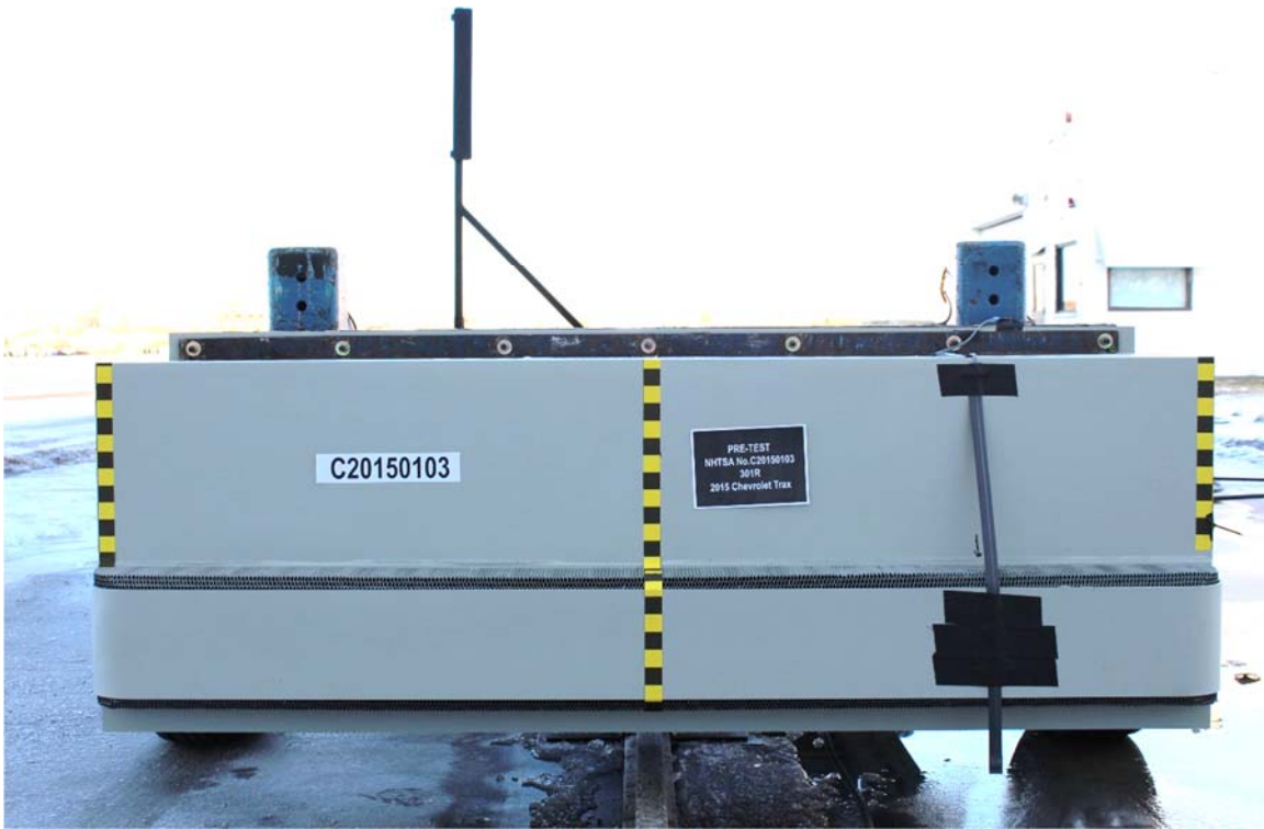
Figure A-19: Pre-Test MDB Front View
