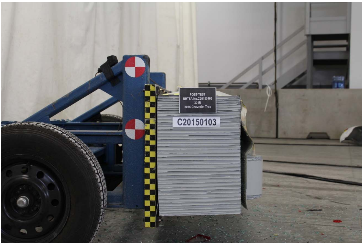
Figure A-24: Post-Test MDB Right Side View
