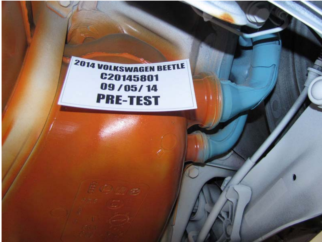
FIGURE 29. Pre-Test Underbody View of Fuel Filler Neck
