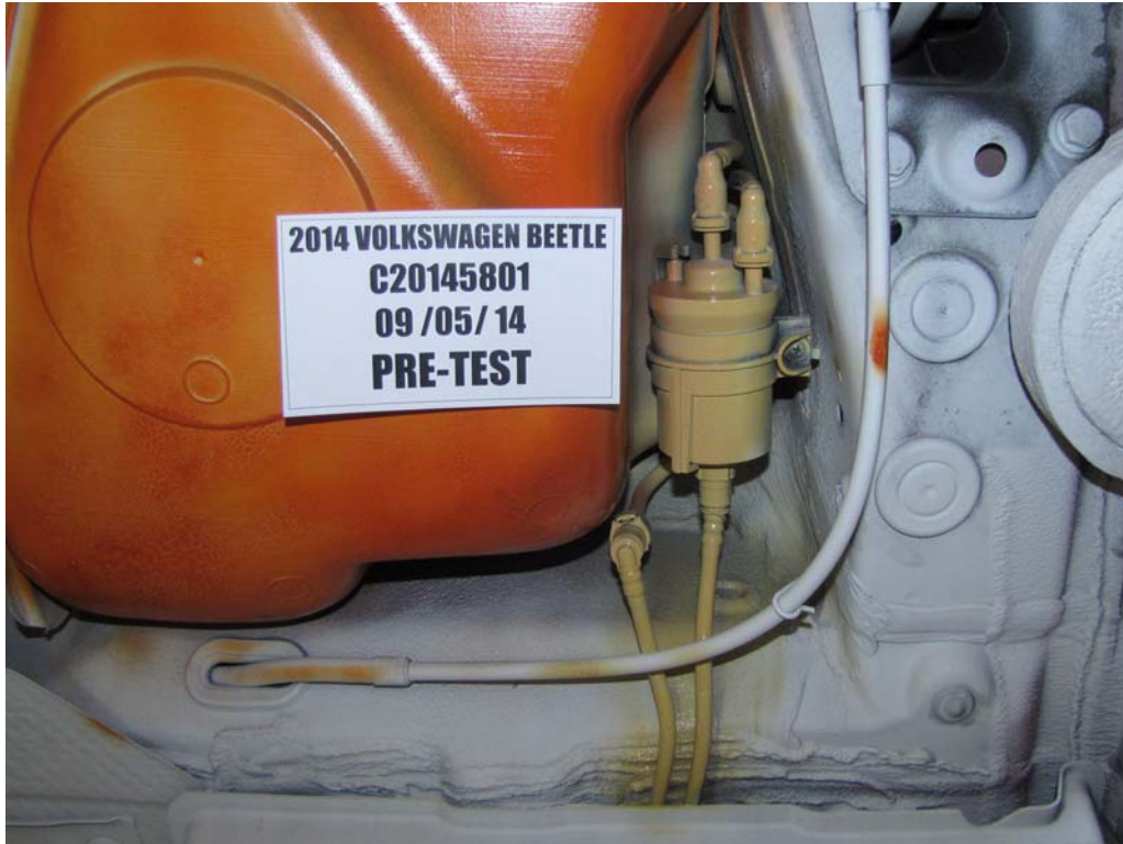
FIGURE 31. Pre-Test Underbody View of Fuel Lines
