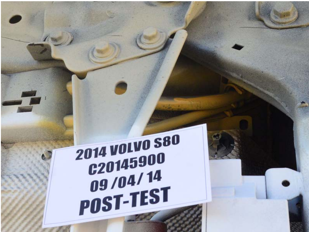
FIGURE 32. Post-Test Underbody View of Fuel Lines
