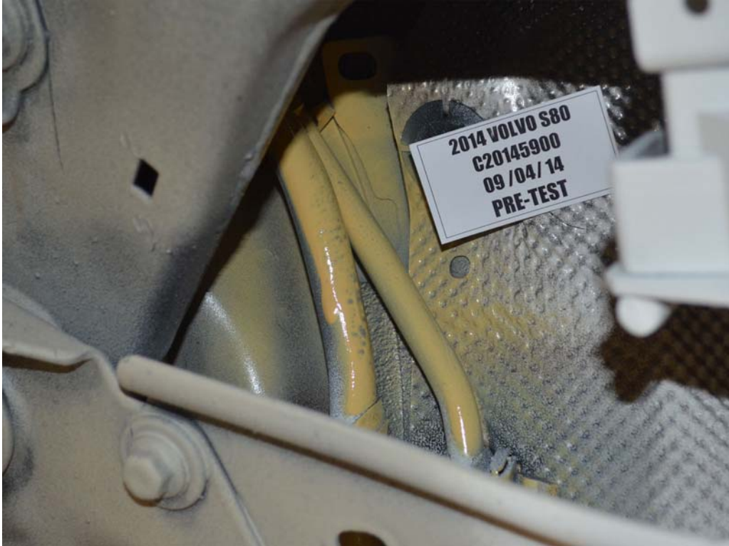
FIGURE 31. Pre-Test Underbody View of Fuel Lines
