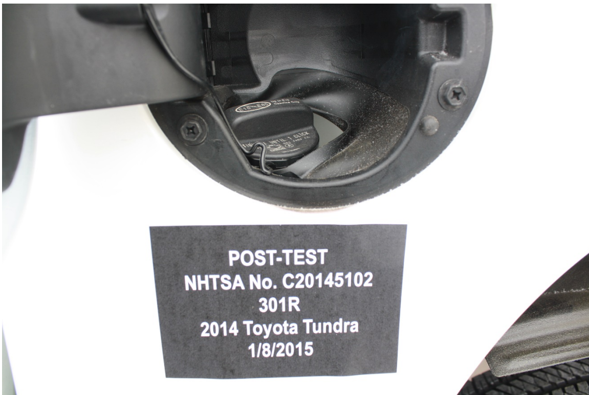
Figure A-36: Post-Test Fuel Filler Cap View
