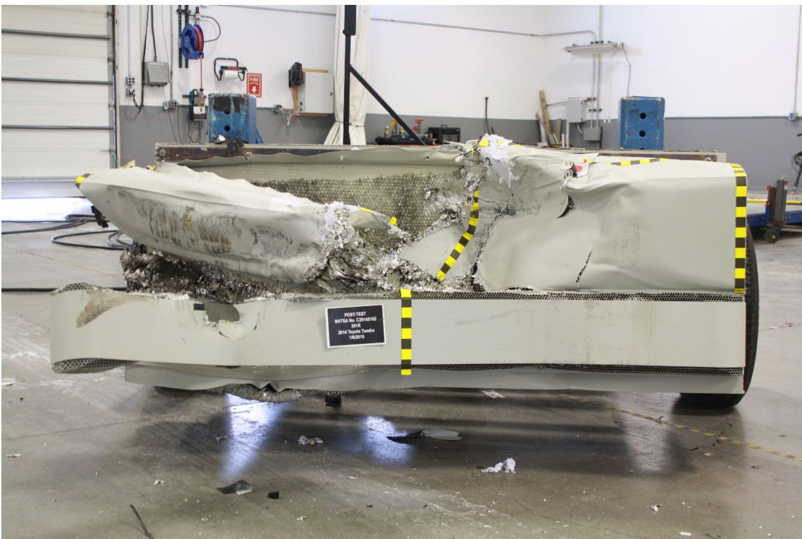
Figure A-20: Post-Test MDB Front View
