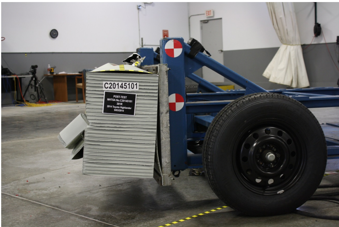
Figure A-22: Post-Test MDB Left Side View
