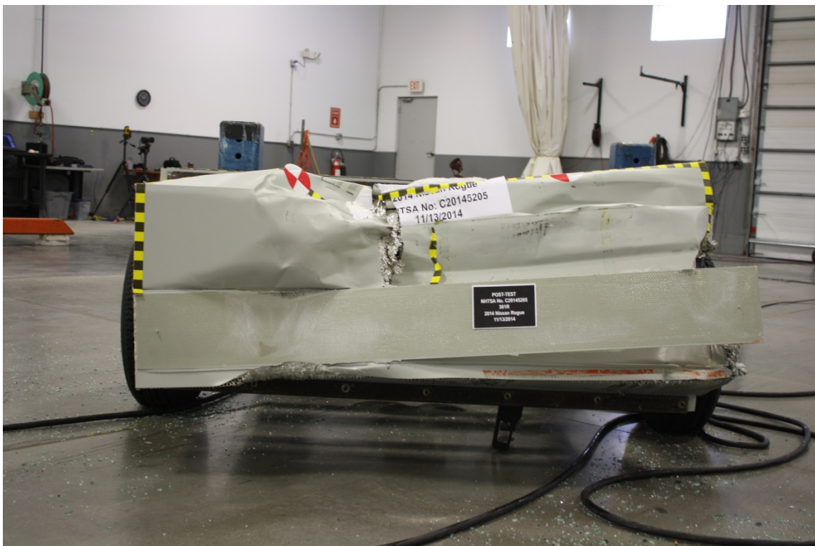
Figure A-20: Post-Test MDB Front View
