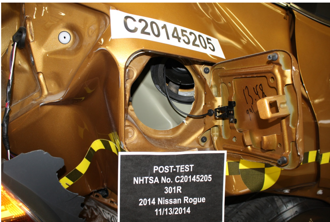
Figure A-36: Post-Test Fuel Filler Cap View
