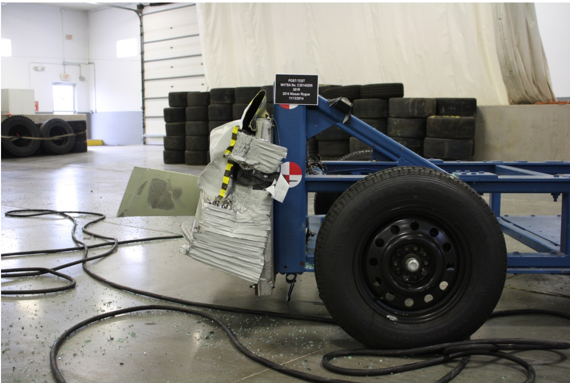
Figure A-22: Post-Test MDB Left Side View
