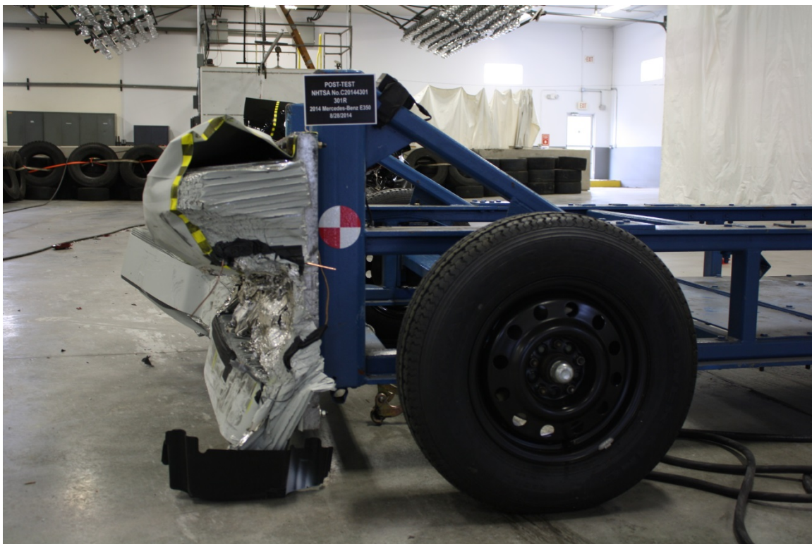
Figure A-22: Post-Test MDB Left Side View
