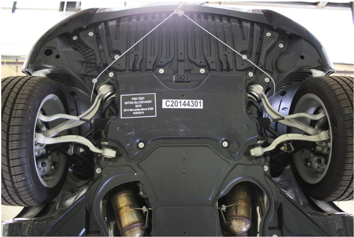
Figure A-29: Pre-Test Front Underbody View
