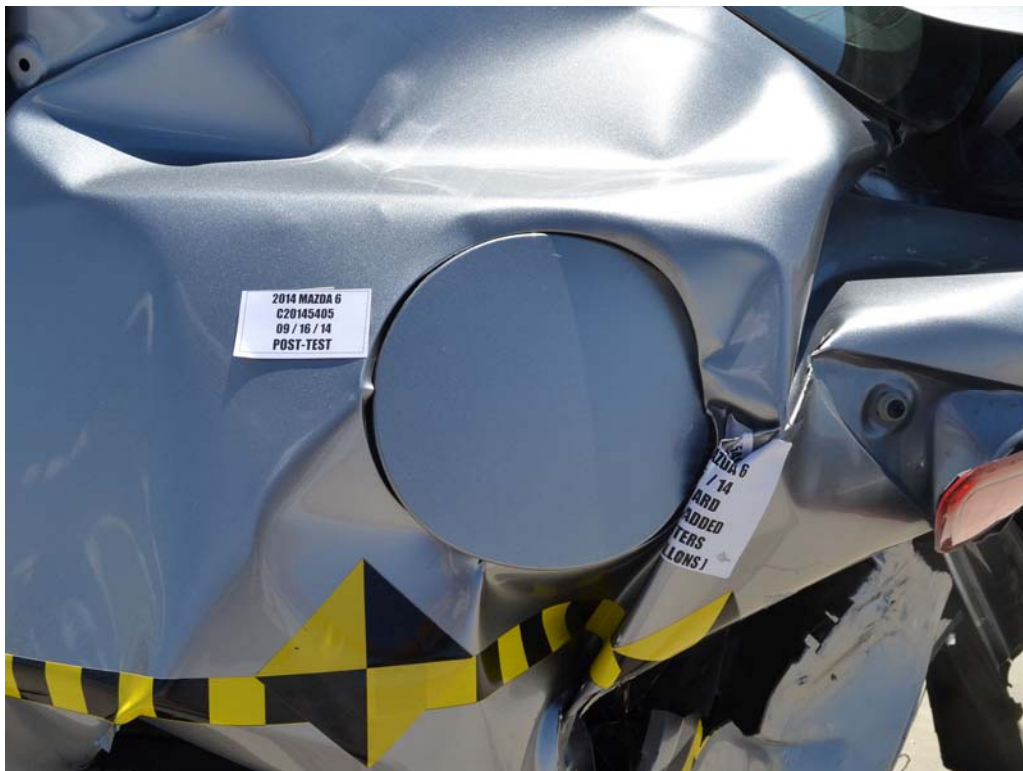
FIGURE 24. Post-Test View of Fuel Filler Cap
